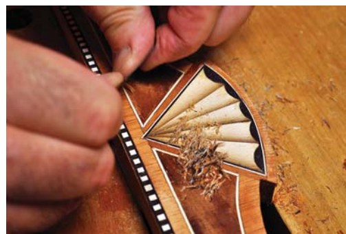
Flushed face. After leveling the stringing, banding, inlay and veneer with a chisel and small plane, scrape it flush with a small card scraper.
