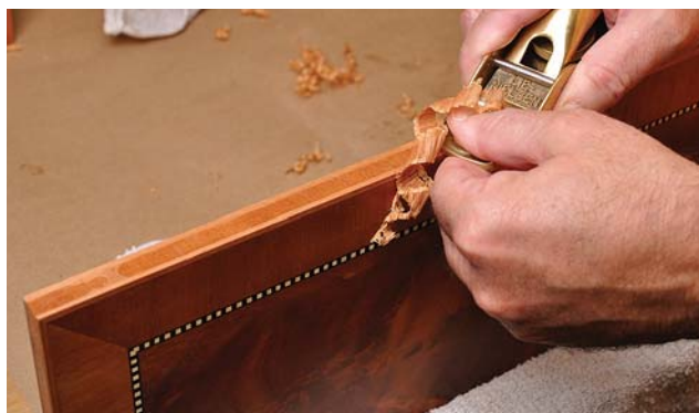
Sharpen first. After the glue holding the vertical mahogany veneer in the groove has cured overnight, sharpen your plane iron and flush the solid banding to the veneer.
