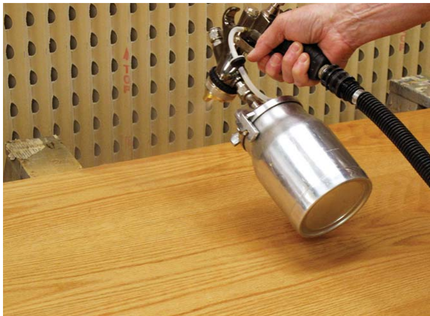
Spraying. There’s nothing special about spraying catalyzed finishes; they spray similarly to nitrocellulose lacquer.
