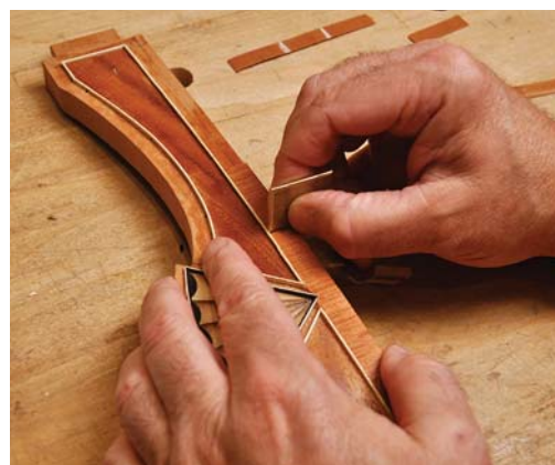
Tight quarters. A traditional veneer hammer is too large and clumsy to use on the crossbanding; I made a "finger hammer" from a piece of brass bar stock.
