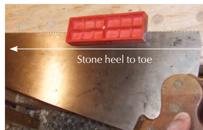
Stoning. To remove burrs left by the filing, and to remove set, make no more than four passes down each side of the teeth with a fine India stone or #600-grit diamond stone.
