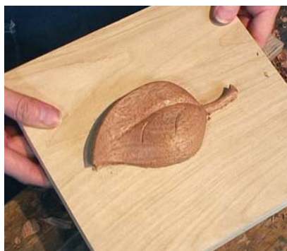
Apply yourself. Carvings may also be separate from the background and applied to a panel after the carving is complete.
