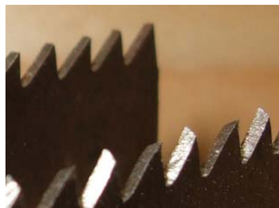
Rip teeth vs. crosscut teeth. Rip teeth (left) are shaped like tiny chisels and are shaped and sharpened by filing square across the blade. Crosscut teeth are shaped more like knives and are formed by filing at an angle to the blade.
