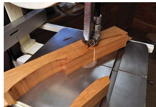
Shapely rail. Use a band saw to rough-cut the profile of the lower rail.
