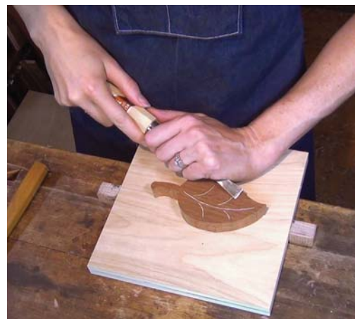
Get a grip. Use both hands on the gouge for control and safety. Keep the hand that holds the metal shaft in contact with the wood and use it to pivot the tool.
