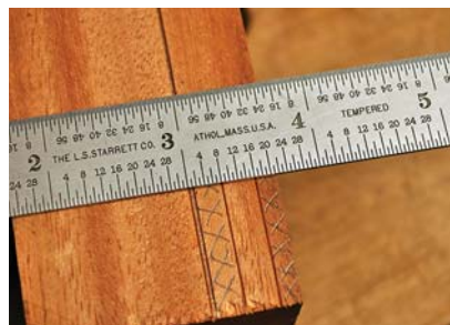
Offset allowance. Lay out 1/4"-thick tenons on the lower rail with a 1/8" rear shoulder and a 1/4" front shoulder – and consider your veneer thickness when laying out.
