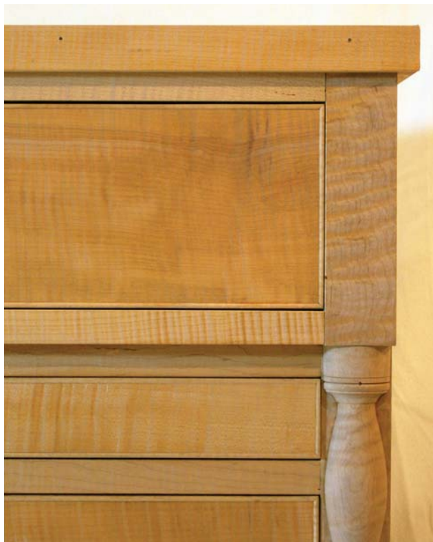
A top with purpose. This unfinished cabinet has minimal overhang to showcase the figured drawers below. The top employs an applied strip on its perimeter to bring it more in scale with the robust structure below.
