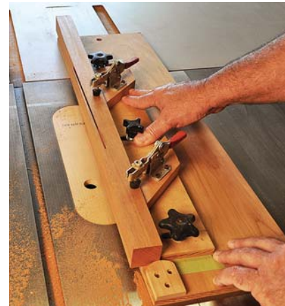
Accurate taper. A sliding jig for the table saw makes precise tapers. Cut two adjacent tapers on all four legs.
