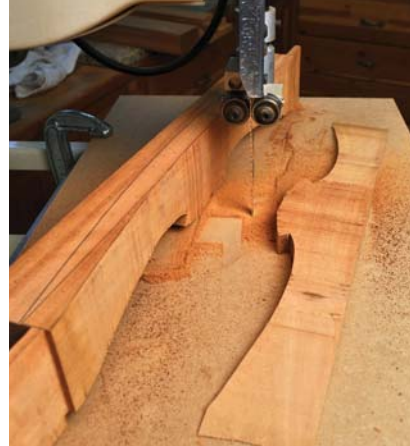
Ample support. An auxiliary table attached to the band saw supports the flat at the center and both ends as you cut the curve on the front and back of the lower rail.
