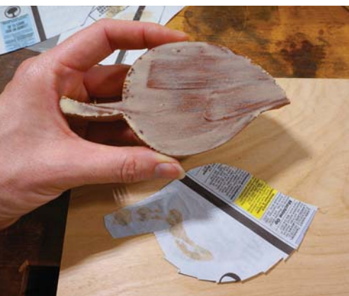
Temporary fix. Paper glued between a backer board and a carving can be easily removed after the carving is complete.
