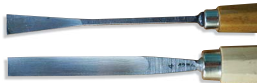
Within reach. These two gouges are the same size and sweep, but the fishtail gouge at the top is more versatile. It can cut into corners and other tight spaces.
