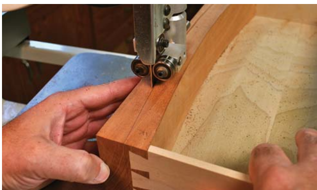
Perfect fit. After fitting the drawer, trace the final curve of the front from the top rail and cut it on the band saw.
