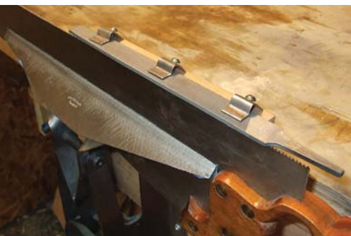
Joint. A file (held here in a shop-made saw jointing guide) levels the teeth to one another and creates a flat top on each. (You can purchase a similar jointing guide; search for “card scraper jointing guide” online.)
