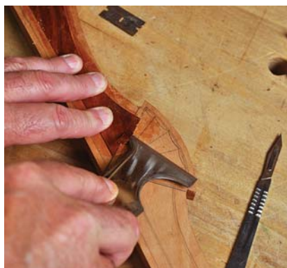
Excess field. A painter's 5-in-1 tool makes quick work of removing excess materials from the field after you've cut to the layout lines.
