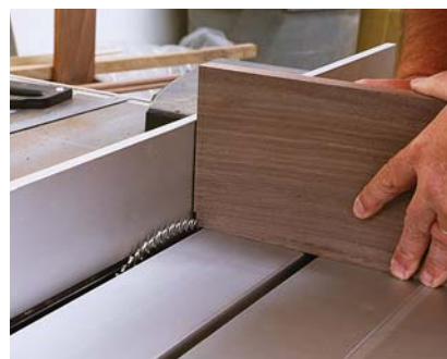
Step out. Each of the parts housed in dados (except for the bit shelves) need to be notched at the ends; it's a simple and clean process using a table saw.
