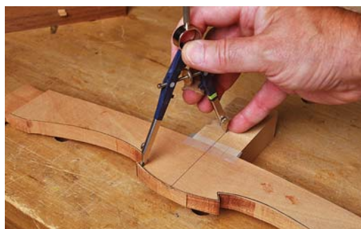
Refine the rail. After roughing out the rail, refine the curves and use a compass to center the drop for the fan.
