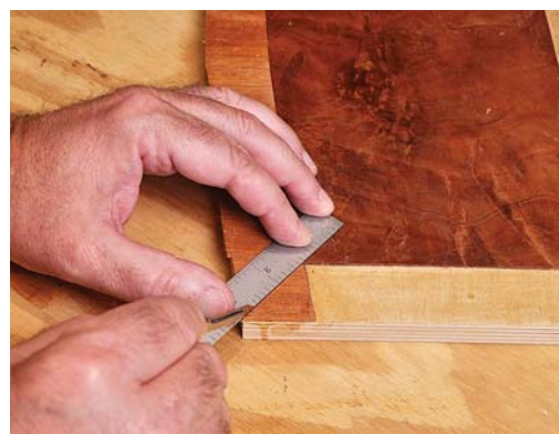
Don't measure. Don't even try to measure the miters. Cut them with a knife against a straightedge from the corner of the veneer to the corner of the top.
