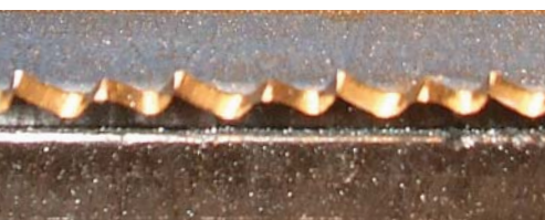
Crosscut tooth geometry. Jointing crosscut saw teeth creates triangular flats at the point of each tooth. These reflect light and help guide the sharpening process.
