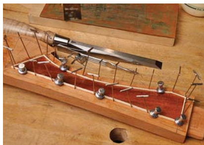
Pinned in place. After the crotch mahogany field is set, apply stringing, mitering the corners and holding the holly tight to the field and down to the rail with pins.
