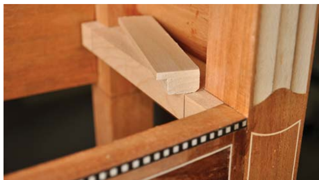
Sneak up on the fit. Rabbeted guides can be tweaked with a small block plane after being glued in place. Cut them tight, then plane a shaving at a time until the drawer fits perfectly.
