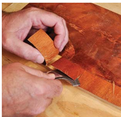
Invisible seam. Overlap the mahogany crossbanding sections, cut through both, peel and remove the waste, then re-glue and re-hammer for a gap-free joint.
