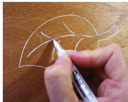
Lighten up. On dark woods, a light-colored pencil or gel marker creates lines that are easy to see. Complete the interior lines by drawing freehand.
