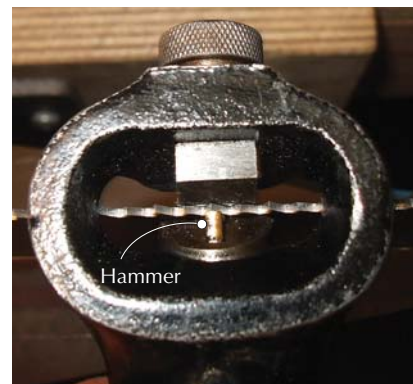
Set. Slip the saw set over the saw blade, rest it firmly on the toothline, align the hammer with a sawtooth, then squeeze.
