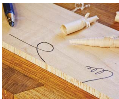
On your mark. The "true face" mark (left) labels this surface as flat and it typically also indicates the inside surface of a cabinet. The second mark (right) is a modern mark used by David Charlesworth. The curls form a point that indicates the grain direction of the board.
