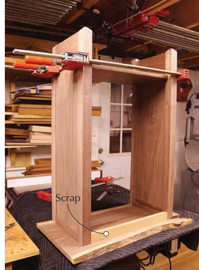
Topper. A scrap cut to the exact length of the opening helps you both to hold things in place and keep things square as you attach the top.
