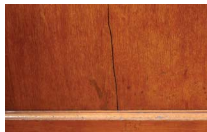
Split. The solid mahogany side of this mid-19th-century desk shrank in the drier air of a modern building. Because the side was attached to a perpendicular baseboard, shrinking was retarded so the side split.
