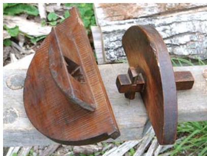
Howell & croze. These tools, part of the period cooper’s arsenal, are used for cutting the groove around the top and bottom of a barrel in which the “heads” (what we might wrongly call the top and bottom) sit. These 19th-century examples are from a private collection.
