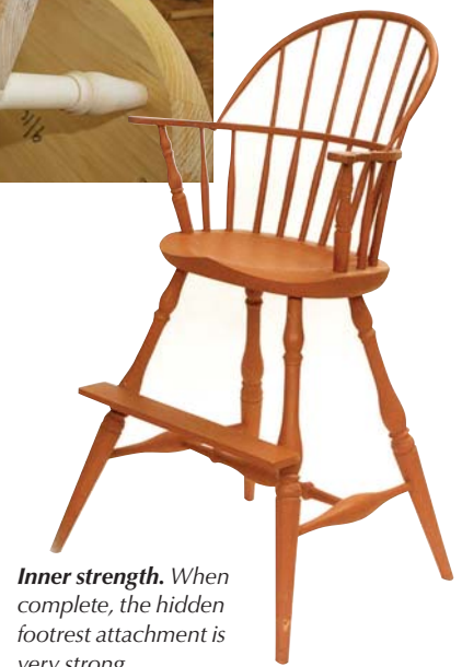
This to that. After placing the splayed dowels in the legs, hold the footrest against them and mark the location and the angle on the bottom face.
