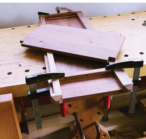
Cleats. After applying glue, clamp the cleats (or secure them with nails) to hold them in place as the glue dries. Either way, just make sure the countersunk holes are facing in the correct direction – toward the floor. (Here, you can also see the case bottom, with the corners notched to fit around the posts.)
