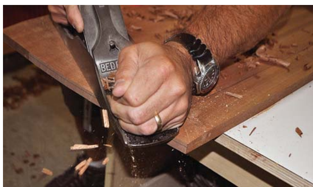
Around the bend. Working the taper around the curves in the top requires hand tools. I find that a plane is the fastest and most accurate method.
