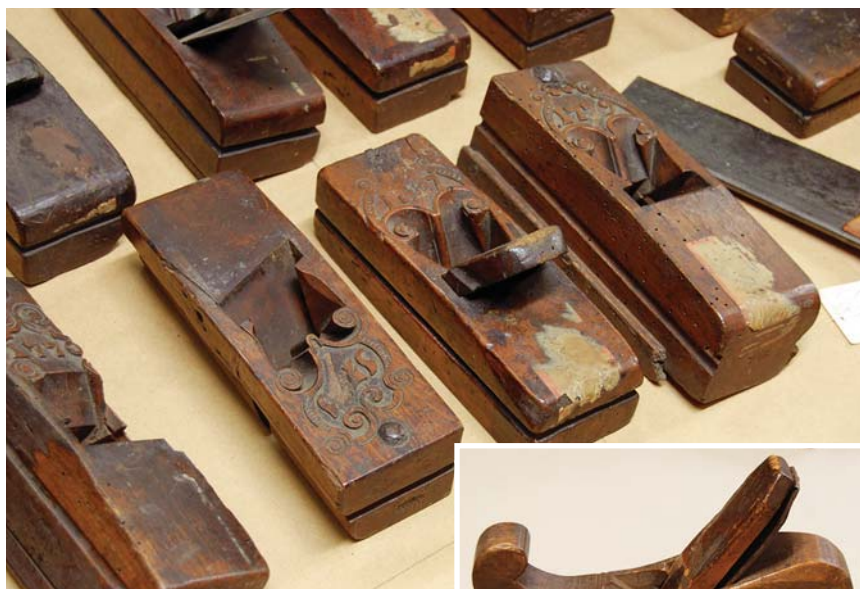
Dutch planes. The planes mentioned in apprenticeship contracts were all shop-made examples; these 18th-century Dutch planes are probably the work of a dedicated plane-maker, but are still entirely hand-made.
