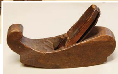
Scroll plane. This Dutch-style smooth plane was also an English form; one appears in Randle Holme's "Academie of Armory and Blazon" (1688). Without Holme's depiction, we would not attribute this style of plane to England. (The planes above are on display at Yale University Art Gallery's Furniture Study.)
