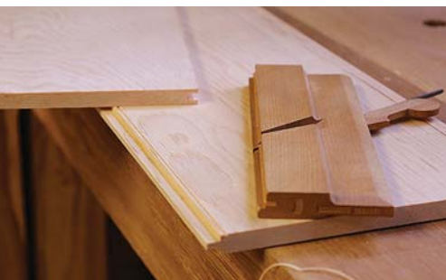
My favorite moulding plane. In just a few passes, a beading plane produces a lovely and crisp detail. Here, I'm using it to dress up the tongue side of my backboards.
