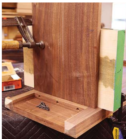
Bottoms up. Ensure the bottom is well clamped before driving screws through the cleats to secure it in place.
