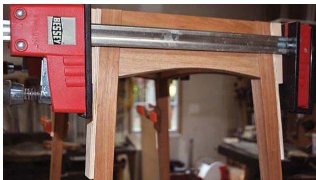
A good bite. Stepped cauls allow the best opportunity for accurate clamping.
