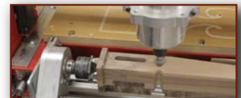
Using the turning system to mill the legs and M/T joint.
