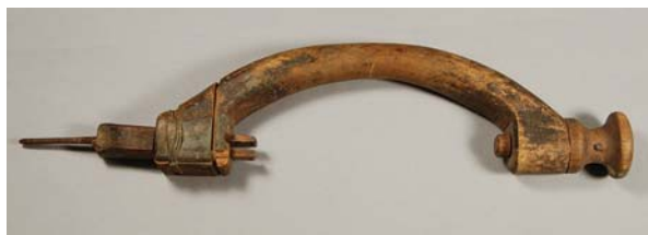
A hole by many names. The "piercer" goes by many titles, among them: wimble, brace, bitstock. No matter what you call it, it's for boring holes. This example is courtesy of Pilgrim Hall Museum, Plymouth, Mass.
