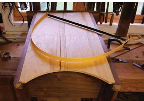
Re-curve. A drawing bow allows you to retain a curve for as long as you need it (in this case, for the front and the back). When you're done, simply release the strap, and the bow returns to flat for storing.
