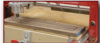
Milling the chair back stiles on the horizontal worktable.
