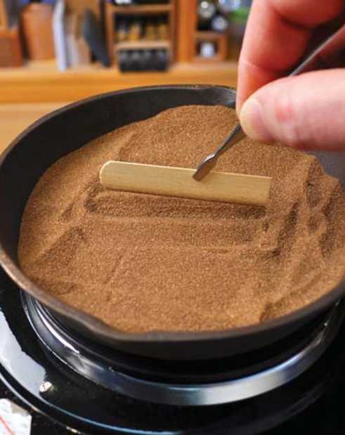
Toasted edges. Shading the edges of inlay pieces in hot sand imparts a three-dimensional appearance.
