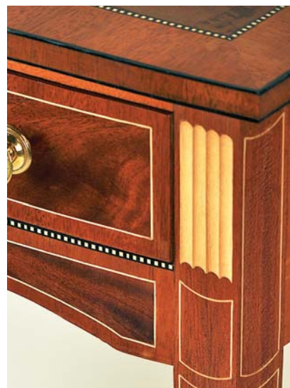
Period touch. Shop-made inlay, such as this bookend design on a table I built, was important in Federal-period furniture; it's a way to decorate using contrasting colors.
