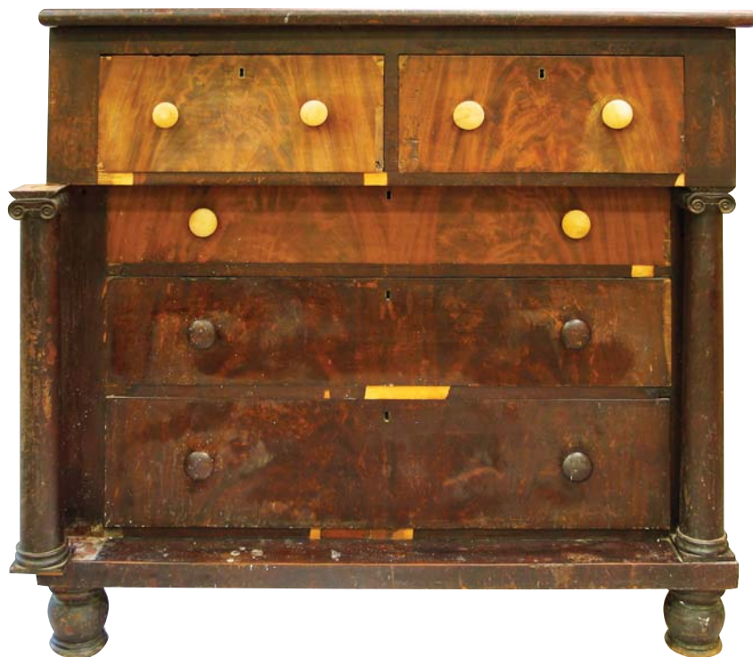
Veneer separation. All the light-colored areas between the drawers (and some on the drawers) of this Empire piece show places where veneer has peeled. It was glued vertically to the horizontal rails. As the glue aged and became brittle, it couldn't keep up with the contrary wood movement.
