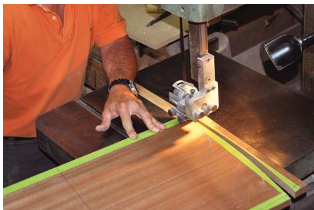
Easy on the eyes. Brightly colored masking tape makes it easy to see and cut the layout lines for the boat-shaped top.
