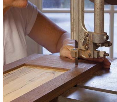
Careful now. The doors are the most visible part of the cabinet. Cut carefully to ensure the apex of your curve meets at the middle.
