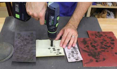
Spin it. A series of sandpaper grits is lined up on a flexible pad, and the drill spins the ebony into each grit.
