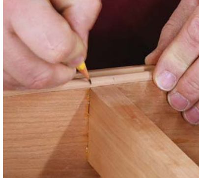
Double-arch mark. Hold the double-arch moulding in place to mark off the position of the drawer blades.
