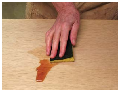
Wiping up a spill. Spills should be wiped up quickly, of course. This was a red-wine spill, which I partially wiped up after less than two minutes. After several light passes with #280-grit sandpaper, the mark was totally gone.
