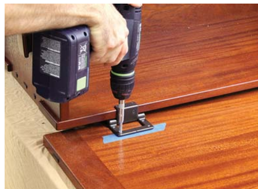
Swing & hold. Torsion hinges serve to hold the lid open without any additional support.
