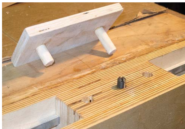
Two methods. I elected to use removable dowel blocks and a simple threaded set screw for my moving carriage.
