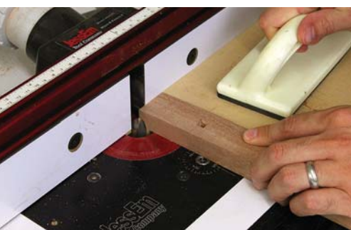
Back up. Scrap wood behind the handle blank makes it easier to control the work as the cove is routed in the end.
