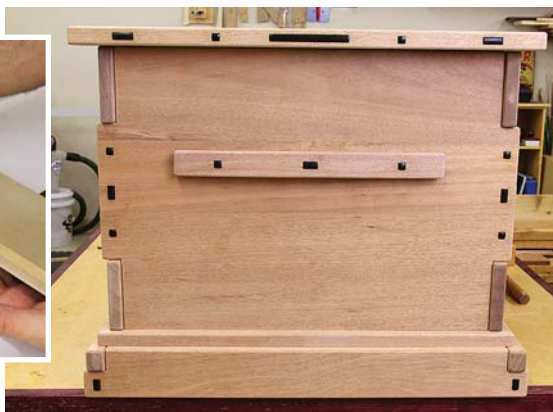
A pattern emerges. The dark plugs and bars add a decorative element and hide the screws.
