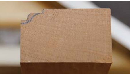
Make it easy. You'll get a cleaner cut off the router bit if you rabbet and chamfer the workpiece prior to running the profile on the stiles and rails.
