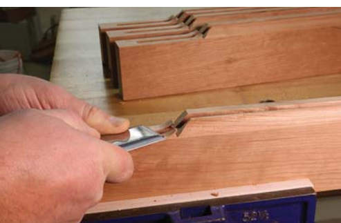
Clean it up. After jointing off the waste, use a sharp chisel to pare the shoulder to the miter.
