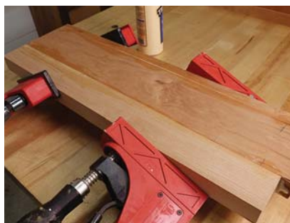
Add a little. Sometimes the materials just don't cooperate. In this case, the lumber for the bottom rails wasn't wide enough. I scabbed on one strip that will be covered by the base moulding at the glue line, and another for the sticking, in which the seam will fall at the fillet.
