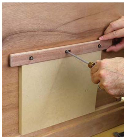
Hold up. A block of MDF supports the handle as it is screwed in place to ensure that the handle is positioned accurately.
