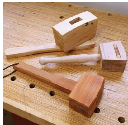
Variations. The overall shape of the joiner's mallet is common, but sizes and weights vary dramatically.
