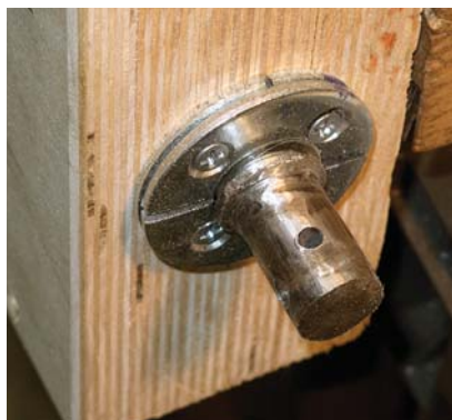
Ingenuity at work. The split garter is actually a pair of split washers in disguise. The end of the rod is modified to accept the hand wheel.
