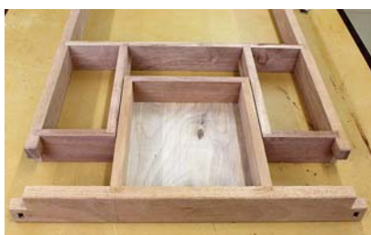
Under the end. The drawer should slide easily and the drawer front should nest snugly below the base front and back.
