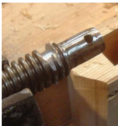
Get the job done. While a lathe makes this step effortless, careful use of a grinding wheel and file can accomplish the same end, although not quite as beautifully.
