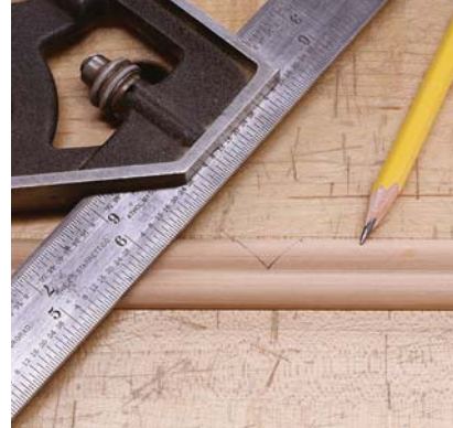
Bevel it right. Once the location marks are in place, draw the miters to ensure a proper cut.
