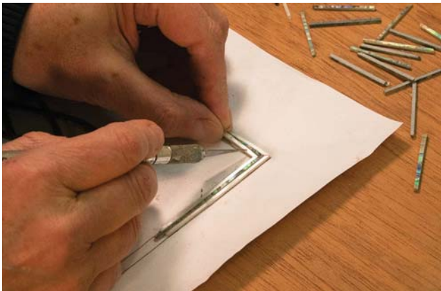
Take your time. Glue the three 1/16" strips of abalone and mother-of-pearl onto the master pattern in an alternating configuration.
