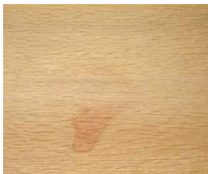
Ten-minute spill. While I was wiping, sanding and photographing, the remainder of the spill just sat on the wood; it left a distinct mark when I wiped it up 10 minutes later.
