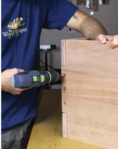
Simple assembly. Screws located under the ebony plugs hold the case together.
