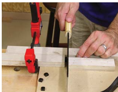
All the same. This jig is used to cut each plug to an identical length.
