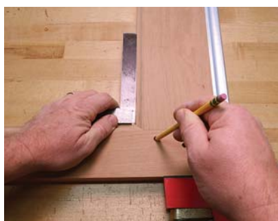
Transfer the mark. With the frame dry-assembled, it's easy to transfer the location of the peg holes to the tenons.
