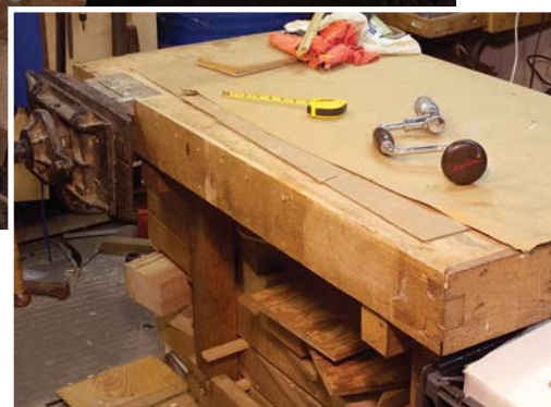
Perfect position. The front edge of my torsion-box benchtop (inset) is the perfect location for a tail vise with a movable dog. The finished vise (above) forever changed the way I work in my shop.
