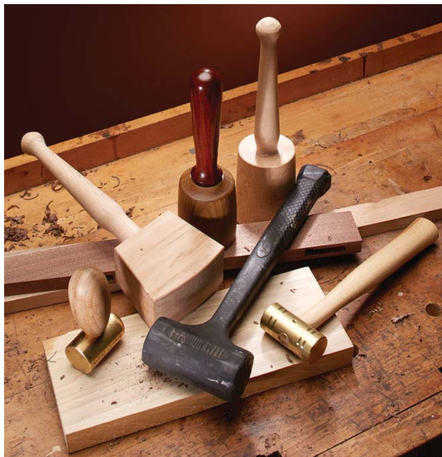
The better beater. Woodworking mallets come in all shapes and sizes, and in many different materials. The secret to choosing the right mallet for the task at hand is to evaluate the head.
