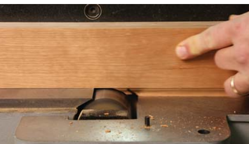
Waste removal. At the jointer, a single pass to remove the sticking waste is fast and accurate.
