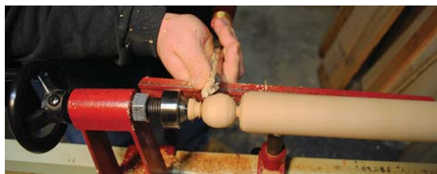
On the ball. The balls on the ends of the screws makes them easier to grab and create the clearance to get your threadbox started.
