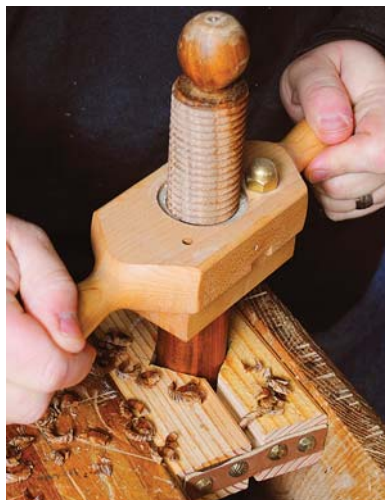
Saddle up. Two pieces of scrap with notches secure the round piece in the vise. The leather strap keeps them together.
