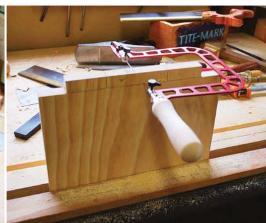
Cut then cope. A dovetail saw makes quick work of the cheek cuts, and a coping saw removes most of the shoulder waste. The rest is cleaned up with a chisel.
