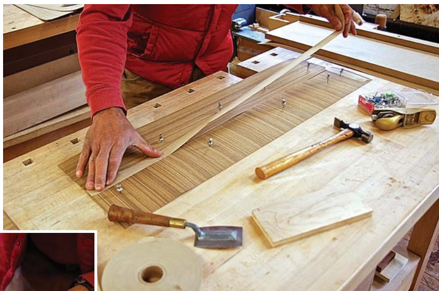
Then that way. After pinning the strips into place, dampened veneer tape is applied along the entire seam.
