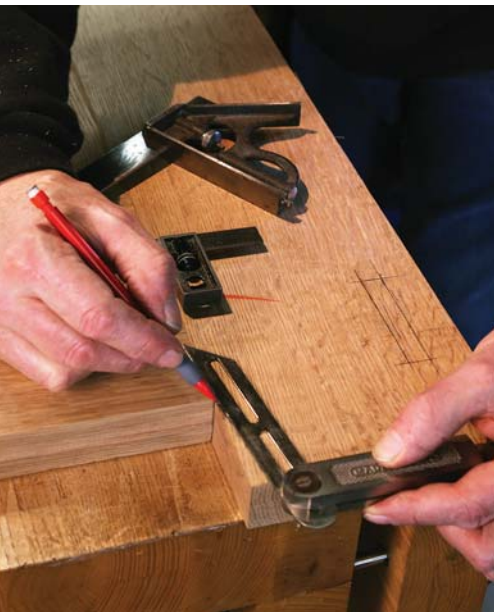
Tapered foot. Before gluing the side assemblies together, use a sliding bevel gauge to mark tapers at the bottom of all four stiles. The tapers start 3/8" in from the inside edge and terminate slightly below the bottom rails.
