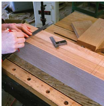
Four at one go. To make layout easier and more exact, group the stiles together and mark them all at once.
