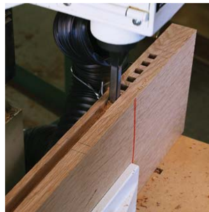
Get in the groove. Your already-cut \frac{3}{8} " groove provides an excellent alignment guide as you cut the mortises.
