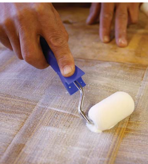
Down under. Yellow glue is applied with a foam roller to the back of the veneer and to the substrate.
