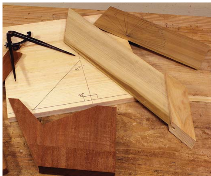
Unsquare squares. The angles for these tools are established with nothing more than a pair of dividers, a straightedge and some basic geometry.
