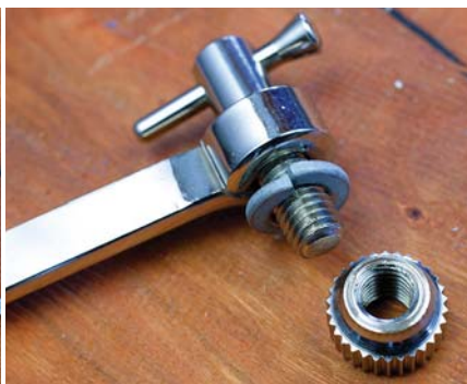
Not that. The current crop of Olson saws come with a plain washer between the handle and the saw frame. Remove it and replace it with a \frac{5}{16} " split washer (left). Then add a split washer between the screw at the toe and the frame (right).
