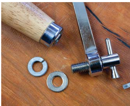
Not that. The current crop of Olson saws come with a plain washer between the handle and the saw frame. Remove it and replace it with a \frac{5}{16} " split washer (left). Then add a split washer between the screw at the toe and the frame (right).
