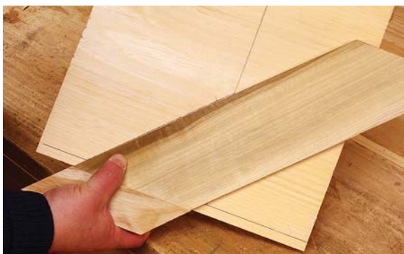
Test, adjust, repeat. Use the 45° line drawn on the board as a reference to true up the miter square.
