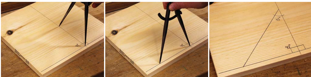
Triangle. Two equal legs joined by a square corner define the 45° right triangle.
