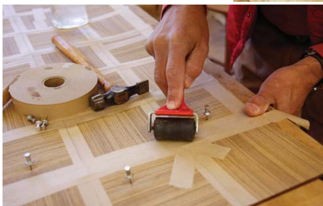
Then that way. After pinning the strips into place, dampened veneer tape is applied along the entire seam.
