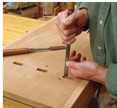
Square corners. A sharp chisel squares the rounded corners left by the router.
