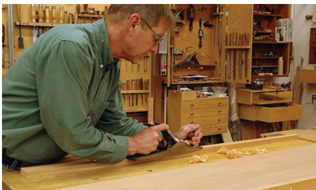
Downhill. After cutting the tapers on the legs with the band saw, remove any mill marks using a jack plane.
