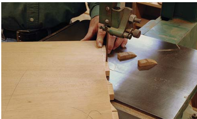
Three-step tenons. Cut the tenon shoulders at the router table, then define each tenon cheek with straight cuts using a handsaw. The waste in between is removed at the band saw.
