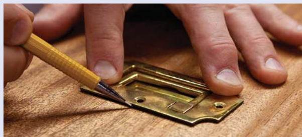
And trace. With the backplate flat against the work, trace around it with a mechanical pencil. Chop away the waste and fit the backplate until it is flush.
