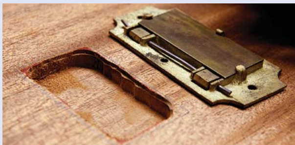
First recess. The deep recess is the same basic shape as the structure shown on the back of the pull.
