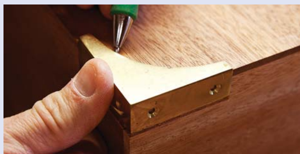
Now trace. With the two legs mortised, you can drop the corner guard in place and trace its shape on the wood. Chop the waste away and your corner guard should fit.
