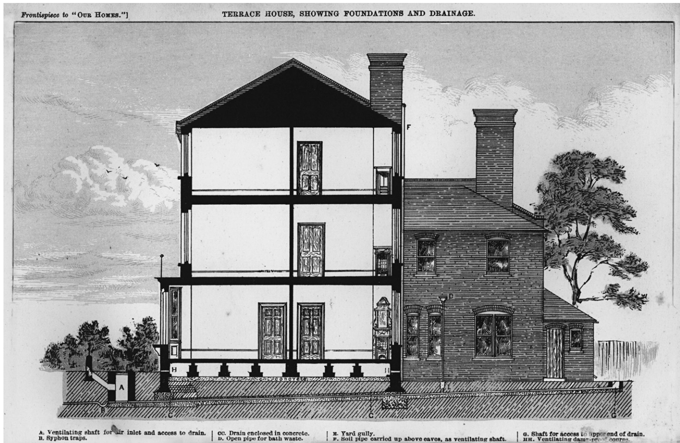
Figure 119 Terraced house, showing foundations and drainage.
