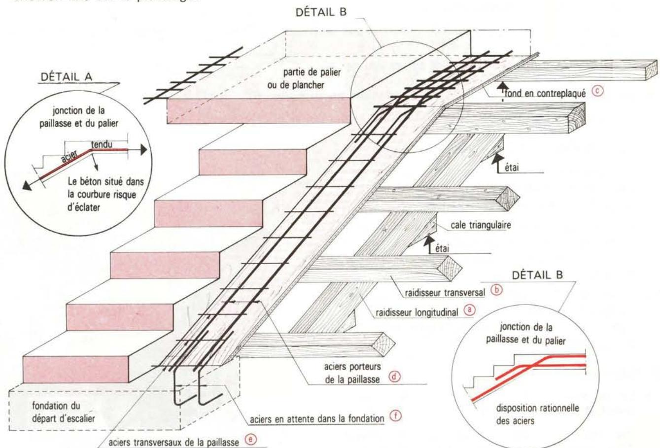
⑰ COFFRAGE DE LA PAILLASSE ET DISPOSITION DE L'ARMATURE
