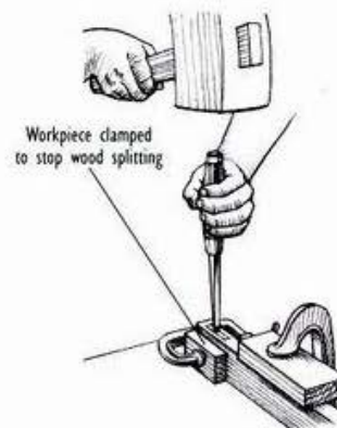
ABOVE: Always make sure that the workpiece is well secured.
