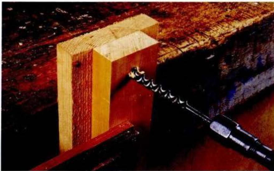
ABOVE: For maximum efficiency, the waste piece needs to run down to the floor.
