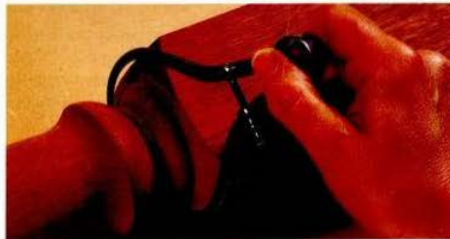
LEFT: To measure the outside diameter, hook the arms of the calipers around the workpiece so the workpiece is cradled, then open the arms until the workpiece just slips free.
