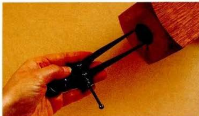
LEFT: To measure the inside diameter, slide the feet into the hole, undo the screw until the little feet are a snug fit then draw them out of the hole.
