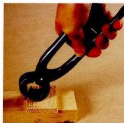
ABOVE: Lever the pincers down and over so the rounded jaws act as a fulcrum.
