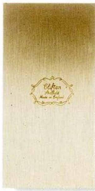
ABOVE: Scrapers are very useful for removing patches of rough grain in an otherwise smooth surface.
