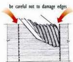
LEFT: Remove the waste with a series of backing-up cuts. Note that the bevel is on the underside.
