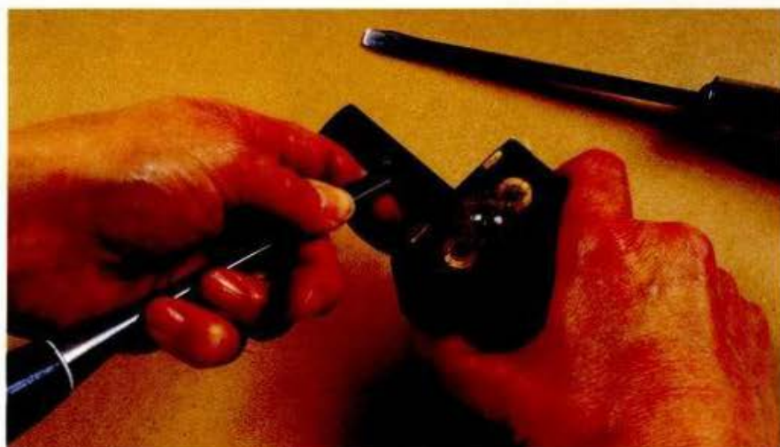
ABOVE: Adjust the two pins directly from the chisel.
