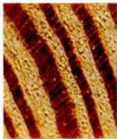
LEFT: End-grain pine with clearly defined annular rings – good for strength.
