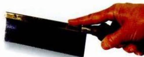
ABOVE: Extend the finger along the back of the saw to help guide the cut.
