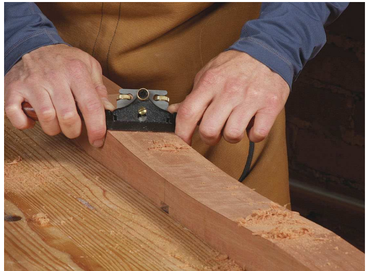
Clean up with hand tools. A spokeshave or card scraper works great on the curved bottom. Use a handplane on the tapers.
