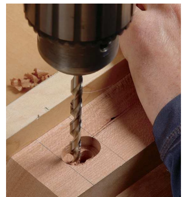
Drill slotted holes for screws. The screws attach the top to the base. Start with the counterbore, slightly overlapping three holes (left). Then drill the clearance hole the same way (right).
