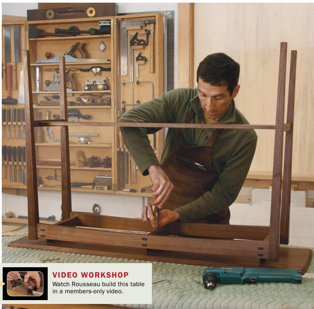
Inverted at the end. After gluing the legs to the aprons and preparing all the parts for finish, Rousseau attaches the top with three screws through each under-rail.
