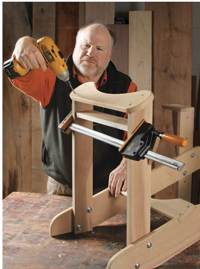
Attach the upper cradle. Use a temporary spacer board to ensure that the risers stay parallel when the upper cradle is attached.
