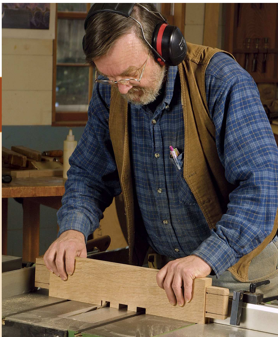
Before assembly, notch the stretchers. Use the tablesaw to notch the arched stretchers for the gridwork. For uniform results, use the same fence and stop setup for the two outside notches.
