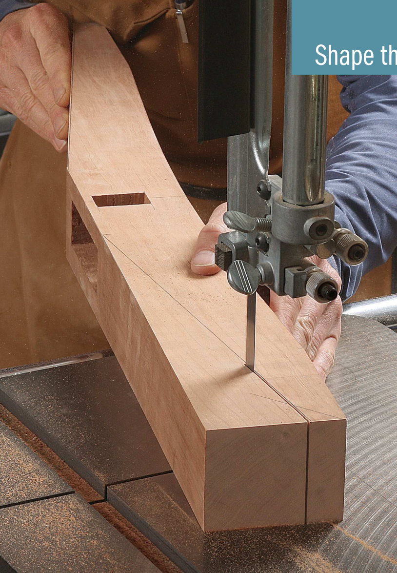
Shape the foot at the bandsaw. Cut the curve on the bottom and the tapers on the top.
