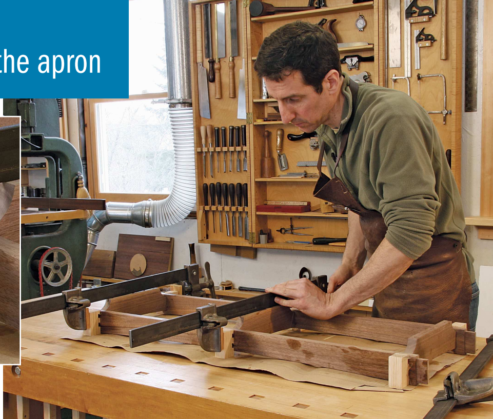
Clever clamping blocks. Rousseau makes custom clamping blocks that accommodate the proud through-tenons. He faces them with packing tape to keep glue from sticking.
