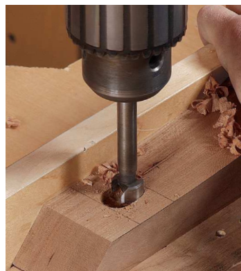
Drill slotted holes for screws. The screws attach the top to the base. Start with the counterbore, slightly overlapping three holes (left). Then drill the clearance hole the same way (right).
