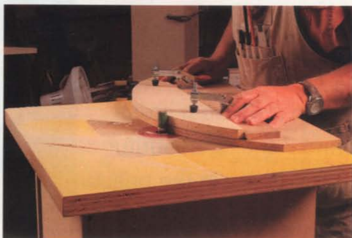
Pattern jig creates matching ribs. Fortune cuts his pattern oversize, then adds a fence and some toggle clamps to make routing the ribs quick, safe, and accurate.
