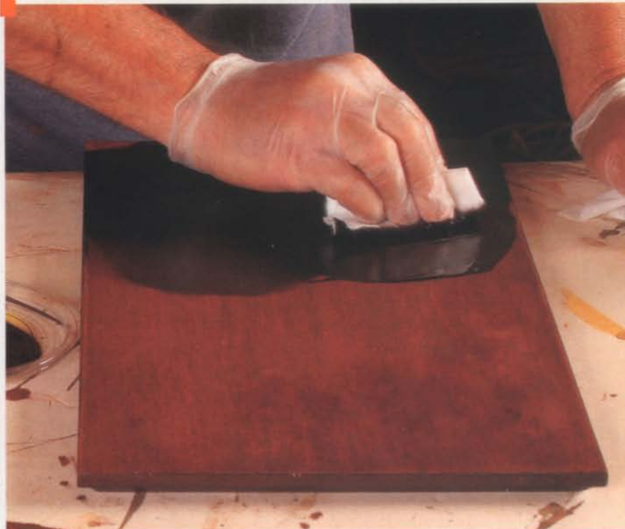
Another shot of color. Wiped on over the shellac, the Espresso gel stain becomes a glaze. Use a dry brush to remove pad marks.
