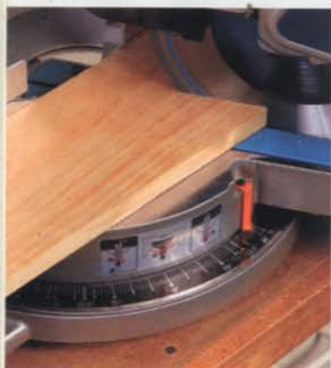
High visibility. Large, white-on-black markings make the bevel and miter scales easy to read.
