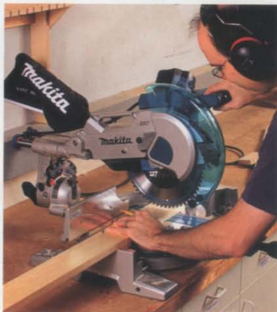
Dual slides. Pairs of top and bottom slides give the 10-in. Makita LS1016L nearly the capacity of a 12-in. sliding model. The maker says the design also improves rigidity for more accurate cuts.
