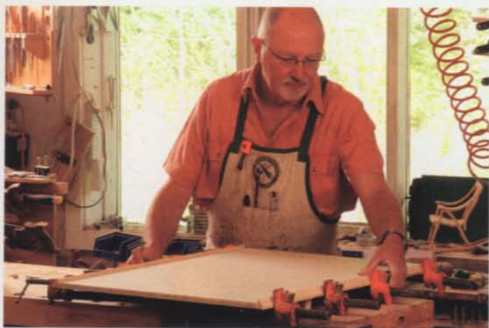
Beveled strips keep ribs aligned on the base. If not held in place on both sides, the ribs will slide out of alignment in the vacuum bag.
