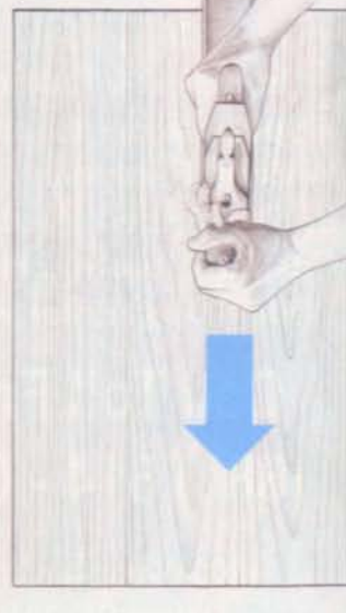
Now go with the grain. Clean up marks from the diagonal passes by planing with the grain.
