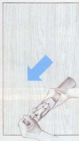
Flatten with a handplane. Even if the glue-up went well, there usually will be small steps between boards and a bit of cupping. To remove these defects, first plane diagonally to the grain.
