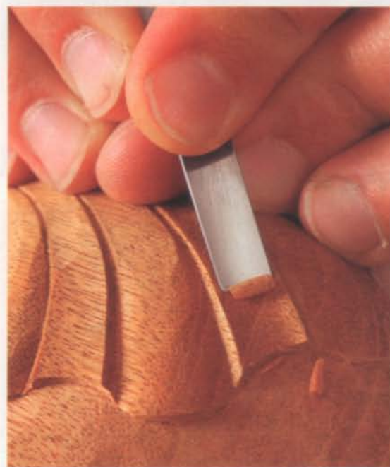
Shape the convex lobes. Use a gouge with the bevel edge faceup to round the sharp edges of each lobe. Begin by rounding at the edges of each lobe (left) and work toward the middle. Use narrower gouges as you work your way down the shell (right).
