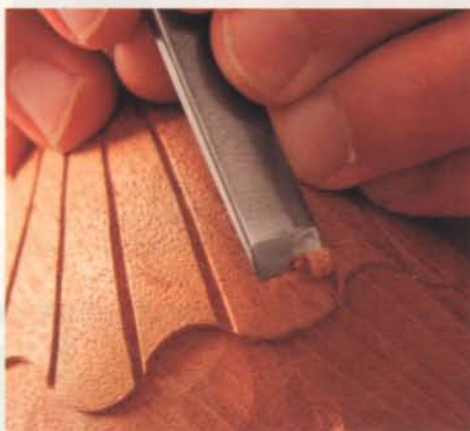
Shape the convex lobes. Use a gouge with the bevel edge faceup to round the sharp edges of each lobe. Begin by rounding at the edges of each lobe (left) and work toward the middle. Use narrower gouges as you work your way down the shell (right).
