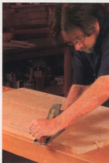
Flatten with a handplane. Even if the glue-up went well, there usually will be small steps between boards and a bit of cupping. To remove these defects, first plane diagonally to the grain.
