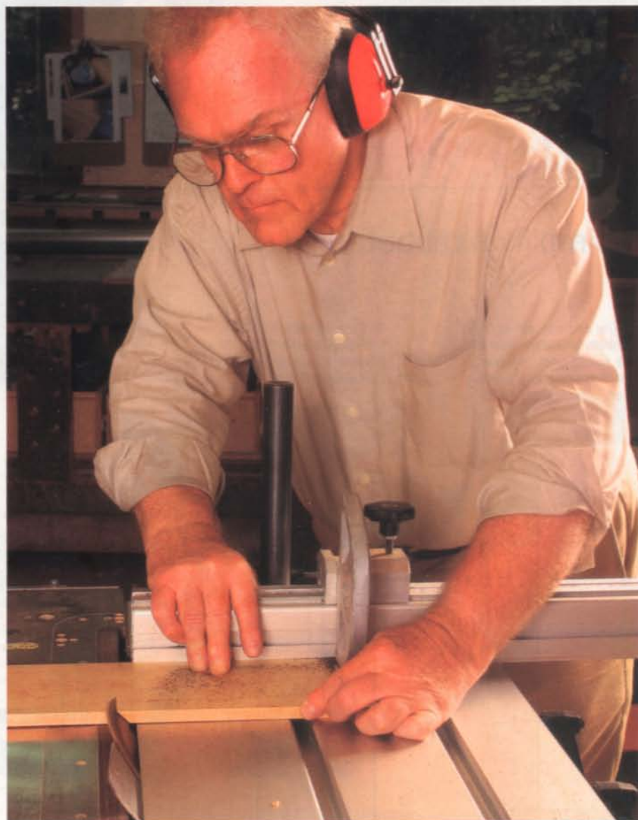
Cut the miters. Use a tablesaw or chopsaw to miter the sides of the box.
