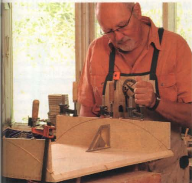
Outer ribs come first. Glued and clamped manually, these prevent the other ribs and spacer blocks from sliding toward the ends of the form.
