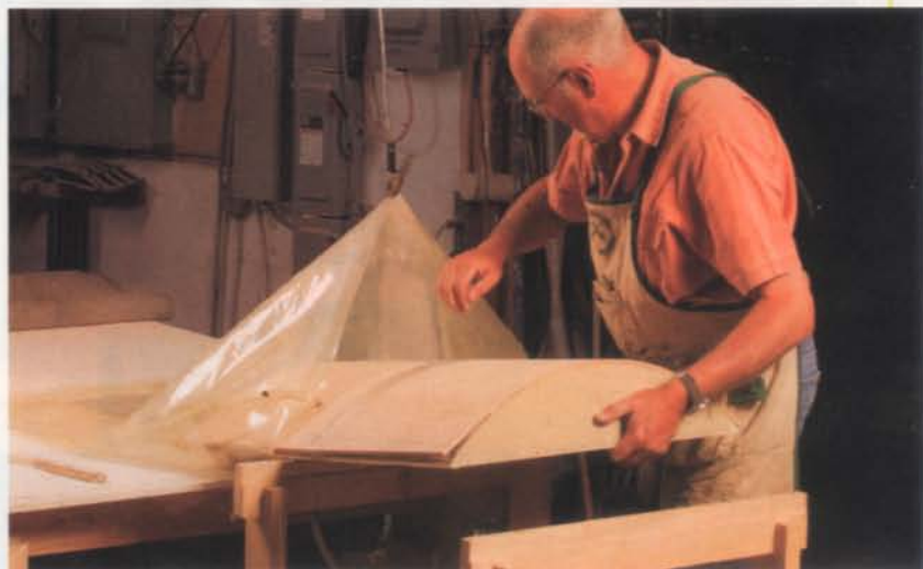
In the bag. The press applies uniform pressure from all directions, so there won't be any bumps in the form. Leave it in the bag overnight.
