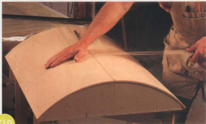
In the bag. The press applies uniform pressure from all directions, so there won't be any bumps in the form. Leave it in the bag overnight.
