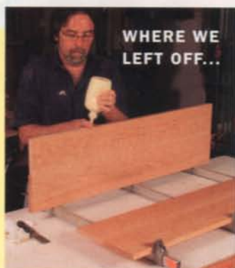
In Part 2 (FWW #208), we spring-jointed the edges and glued up the top.
