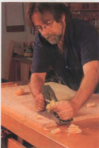
Now go with the grain. Clean up marks from the diagonal passes by planing with the grain.
