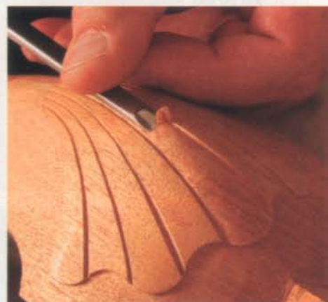
Shape the convex lobes. Use a gouge with the bevel edge faceup to round the sharp edges of each lobe. Begin by rounding at the edges of each lobe (left) and work toward the middle. Use narrower gouges as you work your way down the shell (right).
