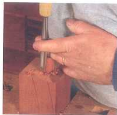
Round the tenons. Guided by a drilled template, round the square tenons using chisels and carving gouges.
