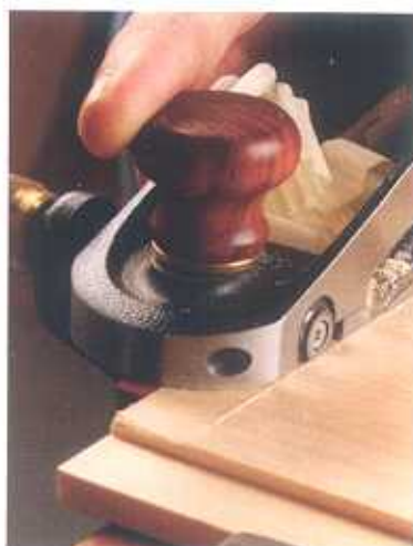
Zero tearout. The skew block plane is available in left- and right-handed models. Although it matters less with joinery where any tearout will be hidden, owning both versions means you'll always be able to plane with the grain.
