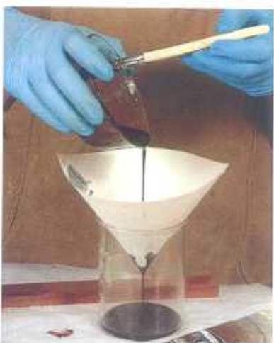
Mix the oil and pigments. Mash the pigments with a cheap brush to break them down and dissolve them in the oil.
