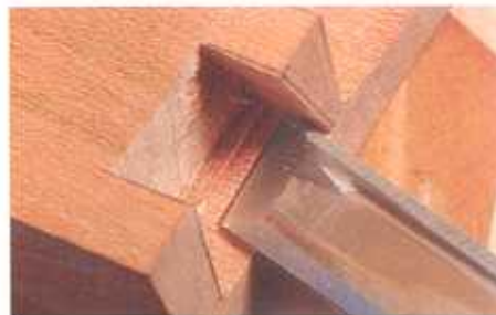
Dovetail corners. The tip of the skew easily shears away the end grain in a half-blind dovetail (far left), and pares the long-grain areas, too (left).
