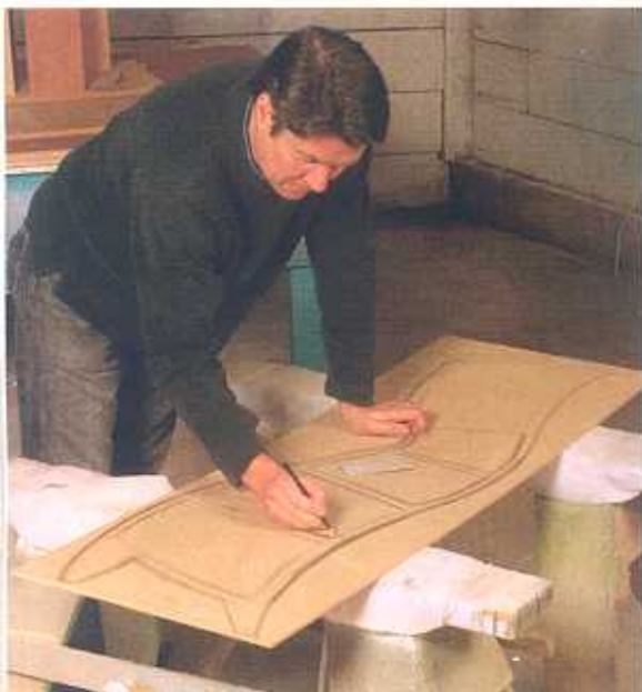
Refine the design at full size. Beaumont draws on 1/4-in.-thick MDF, using sandpaper as an eraser and working the drawing until it pleases his eye.
