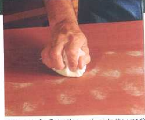
Fill the grain. Force the pumice into the wood's pores using a circular motion. Sprinkle on more pumice until the pores are filled.
