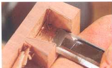
Between tenons. The chisel is adept at cleaning out waste between double tenons as well as for cleaning up the corners at the base of a tenon.
