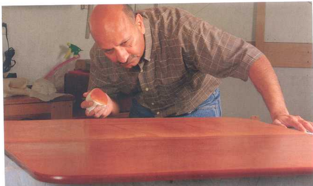
Pounce the pumice. Pour some superfine 4F pumice into a cotton bag and then knock the bag at even intervals on the workpiece.
