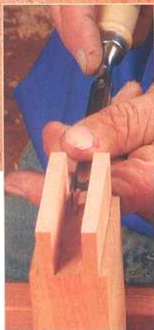
Between tenons. The chisel is adept at cleaning out waste between double tenons as well as for cleaning up the corners at the base of a tenon.
