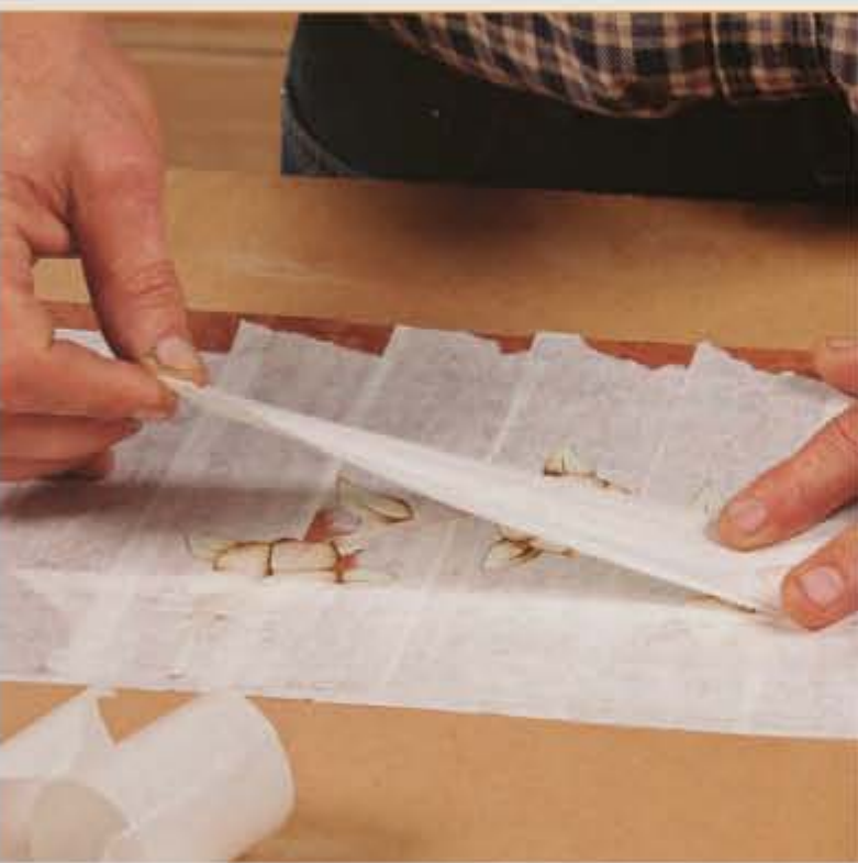
Tape the show face. Now gum tape goes on the show face to hold everything together through the glue-up process.
