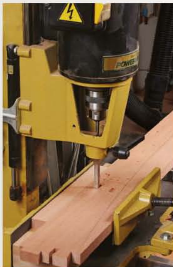
Finish the rail. Dry-fit it and scribe the arc, lining it up with the legs. Now lay out the double mortises for the drawer divider end caps. Simplify the mortising using a spacer between the rail and fence when making the second mortise (center). Rough out the curve on the band-saw, then rout the rail flush to the template (right).
