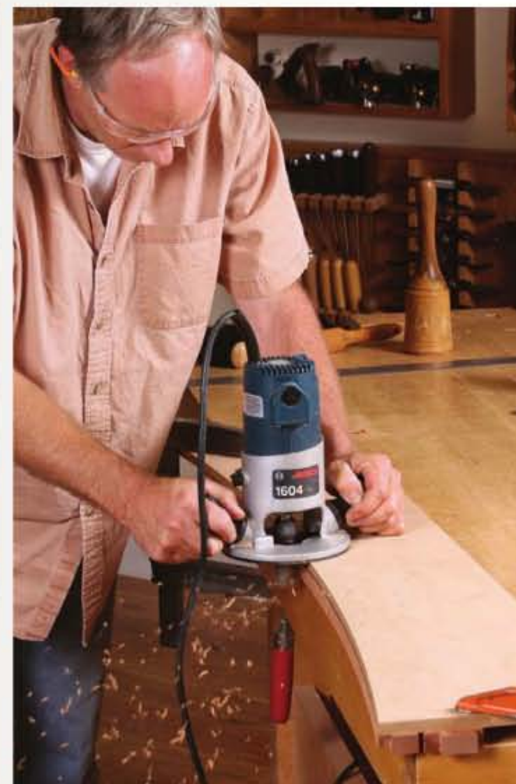
Finish the rail. Dry-fit it and scribe the arc, lining it up with the legs. Now lay out the double mortises for the drawer divider end caps. Simplify the mortising using a spacer between the rail and fence when making the second mortise (center). Rough out the curve on the band-saw, then rout the rail flush to the template (right).
