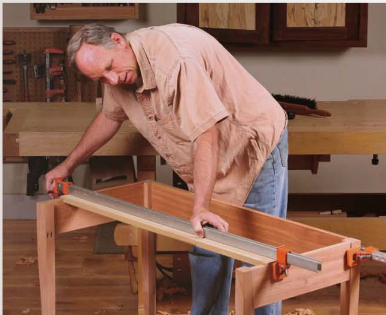
Dry-assemble the base. Clamp the sides to the back apron. A spacer up front keeps the base square. Place its front edge 3 \frac{7}{8} in. from the leg's front, as a reference for locating the top rail.
