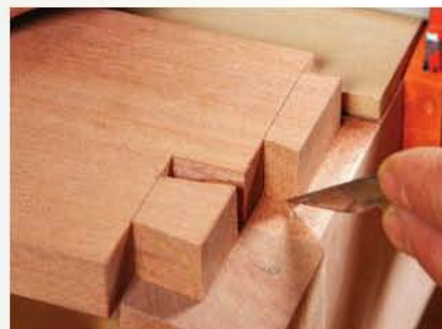
Double dovetail. After cutting two tails on the end of the rail, transfer their locations to the leg and apron. Make the sockets and fit the joint.
