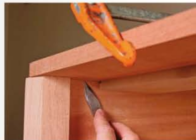
Mark the joint. Center the top rail, clamp it to the spacer, and mark a shoulder line by scribing around the leg and apron.
