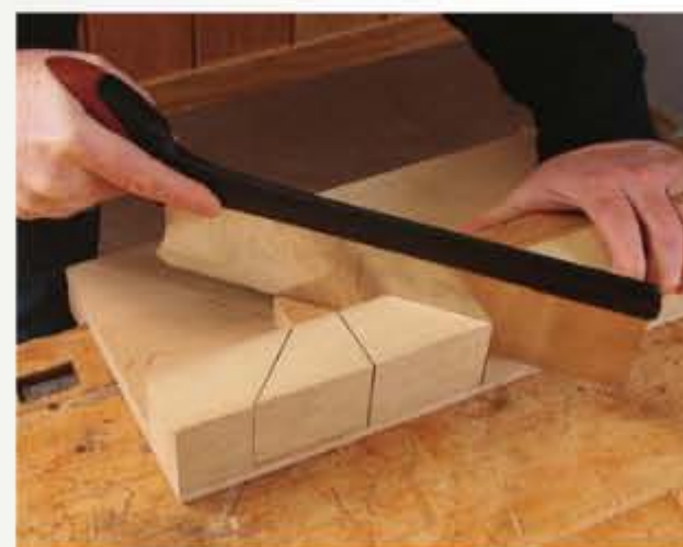
Hooked. With the help of a bench hook, a crosscut saw makes quick work of miters for frames. It also can make accurate 90° cuts.
