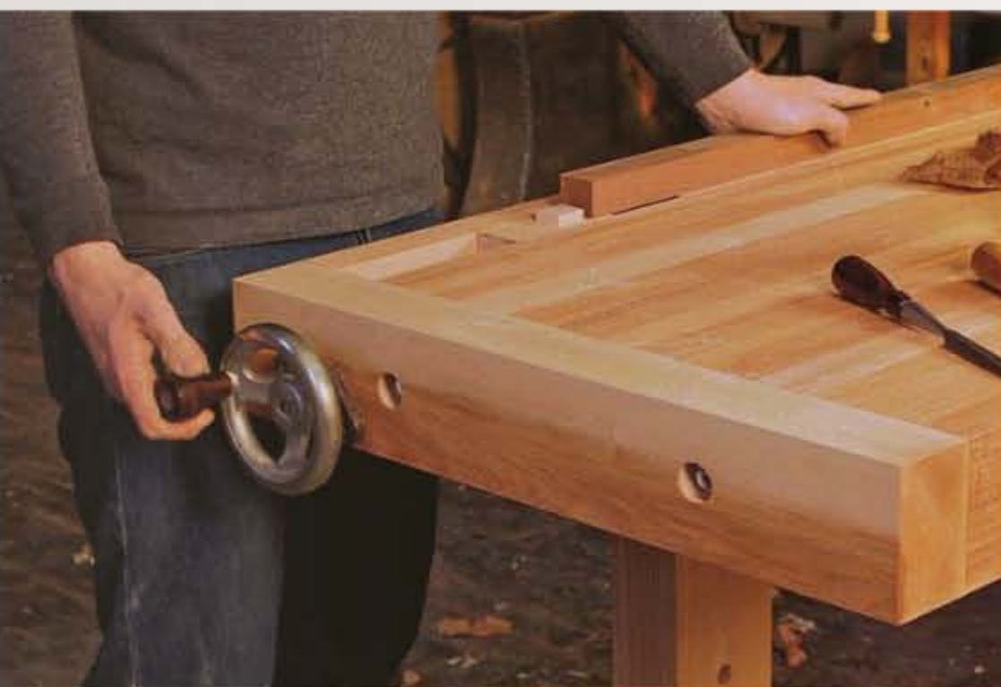
Strong grip, no flex. Benchcrafted's tail, or wagon, vise is integrated into the top, providing solid clamping power without any flex.
