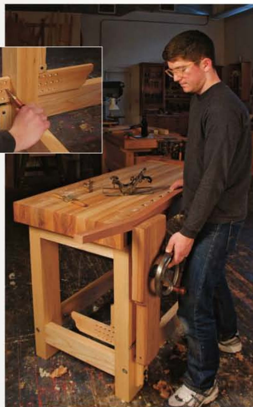
Bench vise with bite. After setting a pin close to the thickness of the workpiece to even out the jaw angle (inset), the glide leg vise has an unrelenting grip.
