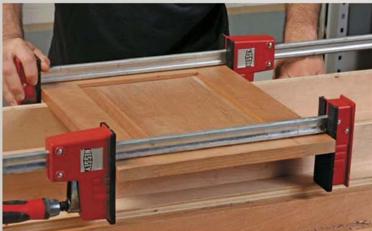
Clamp from above. Use the clamp bars like winding sticks to help you look for twist in the door frame. It's easier to see high spots under the bars.
