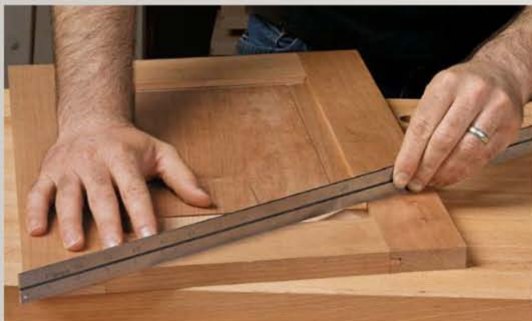
And a rule. Dry-fit the door and lay a straightedge over the surface to look for warping in the frame. Check it diagonally as well as across the joints.
