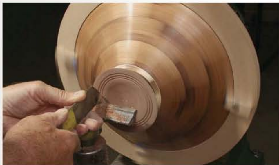
Works like a charm. The bowl spins true and holds fast, allowing Breese to face off the bottom, hollow its center a bit, and then turn a few nice details before sanding and finishing this last area.
