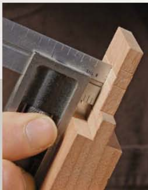
Check it with a square. Tenon cheeks and mortise walls must be straight and parallel with the faces, or the whole door frame can twist.
