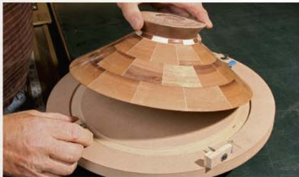
Reverse turning. You need to flip the bowl around to finish off the bottom. A vacuum chuck will hold it nicely, or you can make a simple faceplate as shown. Breese turned a channel in MDF to fit the rim of the bowl exactly, then screwed on small wood tabs to hold it in place.
