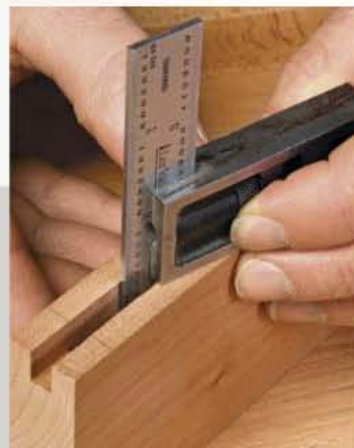
Check it with a square. Tenon cheeks and mortise walls must be straight and parallel with the faces, or the whole door frame can twist.
