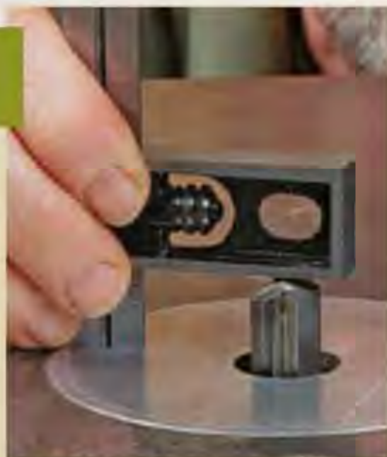
Set heights. Place the blade of the square on end to set router-bit heights.
