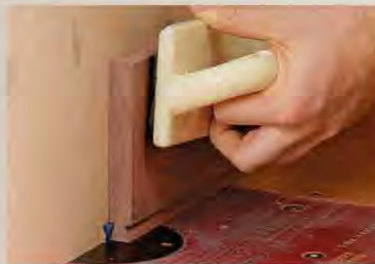
Better keys in bigger pieces. Rout the key on the bottom of a larger piece to stay safe and get a clean cut. Raise the bit a little from its earlier position. Also, bury it in a sacrificial fence if possible.
