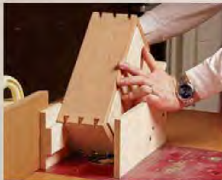
Use a sled for the slots. A simple jig, registered against the fence, holds the box at 45° and makes it easy to cut the dovetail slots.
