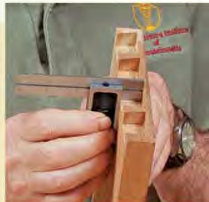
Work in small spaces. Use the rule to check inside half-blind dovetails.
