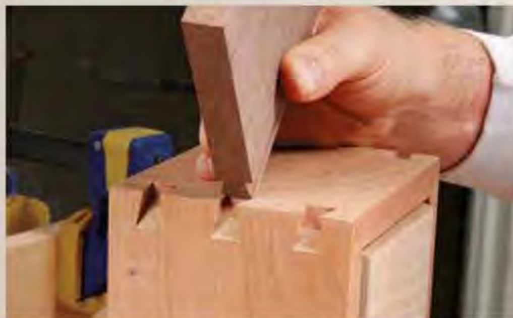
Adjust the fit. If the key is too thick, move the fence and recut one side. When it fits, rip away the key stock, and crosscut keys as needed.
