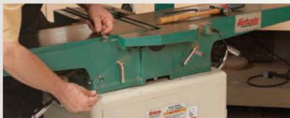
A pair of shims at the bottom lifts a sagging table.
