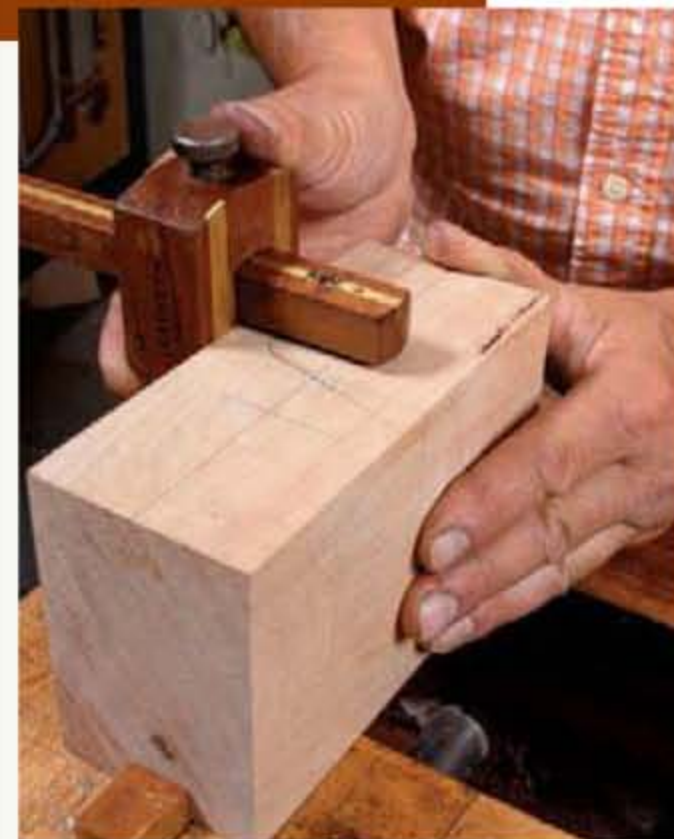
Scribe the walls. Use a marking gauge to scribe mortise walls equidistant from each side.
