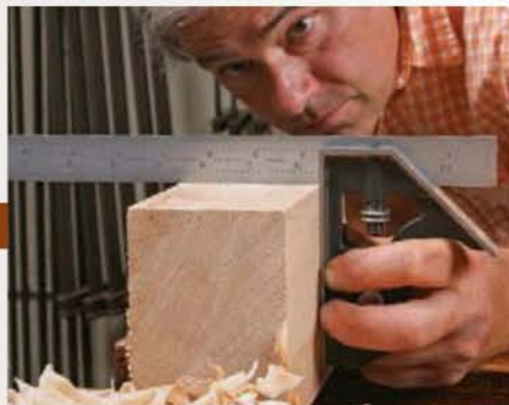
Square an edge. Rotate the block and plane the edge flat. Use a combo square to check that it's 90° to the face. If not, plane the high side.
