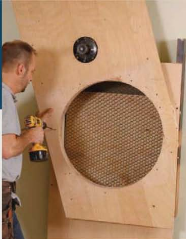
Add the motor. Screw the motor-mounting plate to the exit ring. The front of the motor and its pulley protrude through the plate.
