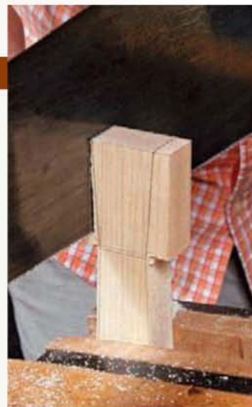
Flip it to finish the job. Turn the workpiece upside down to saw the flare at the bottom of the handle.
