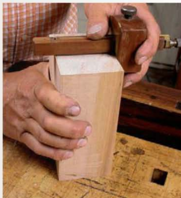
Scribe the rest. Set a marking gauge to the final dimensions and run it along a flattened side to mark one parallel line all around the block. Then plane down to that scribed line, stopping as close to it as possible.
