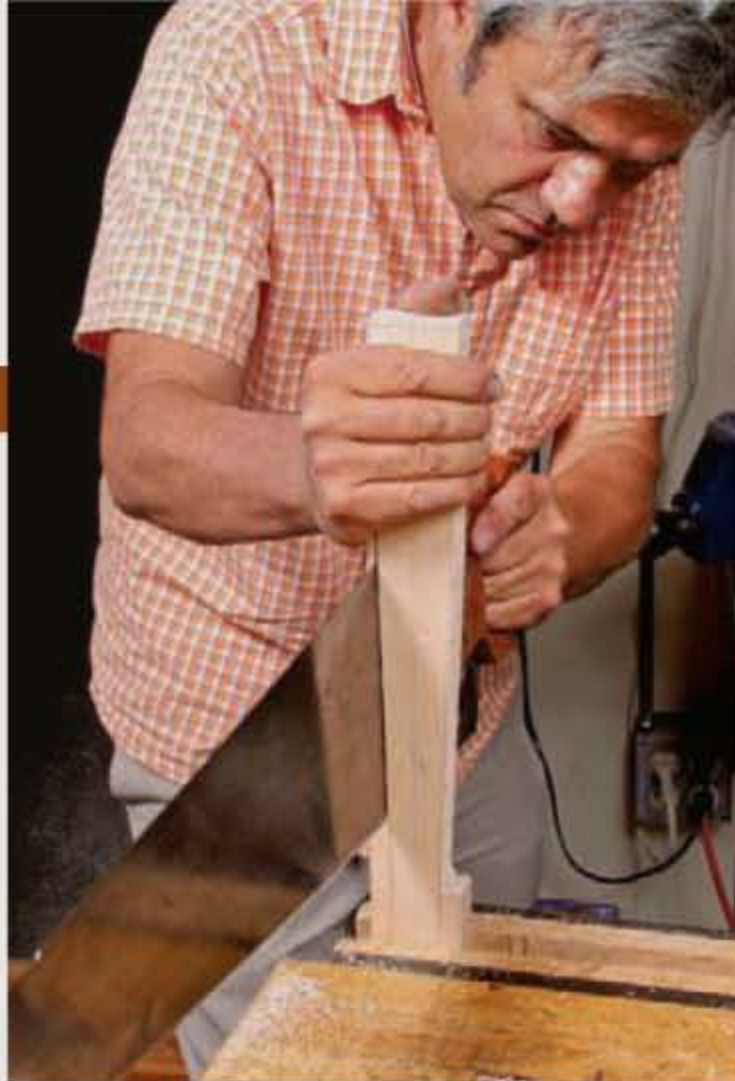
Saw the tapers. Make a small crosscut at the narrowest part of the handle and then saw down into it, keeping to the waste side of the line.
