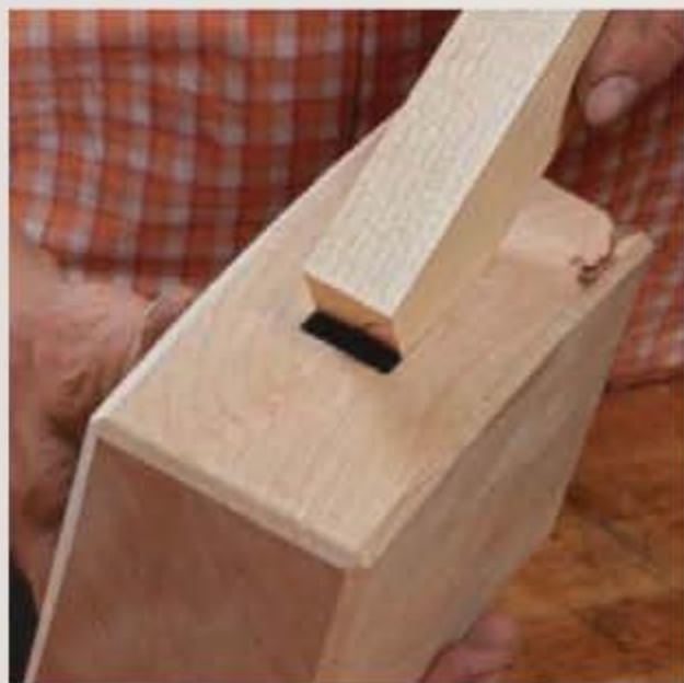
Thickness first. Start with an oversize, square handle and plane the sides until it fits snugly.
