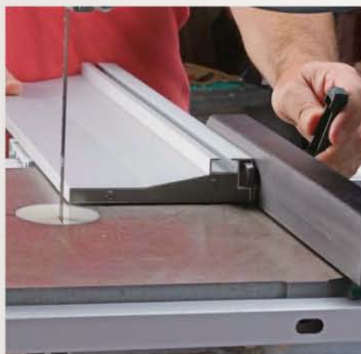
Quick changeover. The fence extrusion switches in seconds to its low-profile mode (left), or comes off altogether (right) for added rip capacity.
