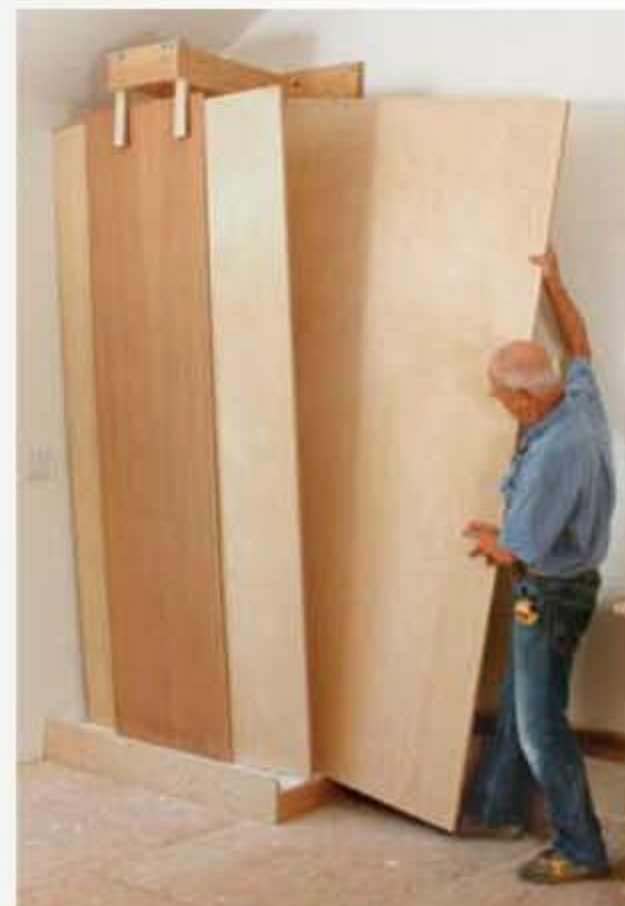
Take your pick. The restraining bars let you leaf through the stack to find a sheet and remove it easily without removing others.
