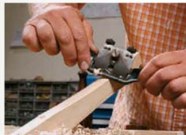
Contour the grip. Last, shape the grip with a spokeshave so that it feels comfortable to hold.
