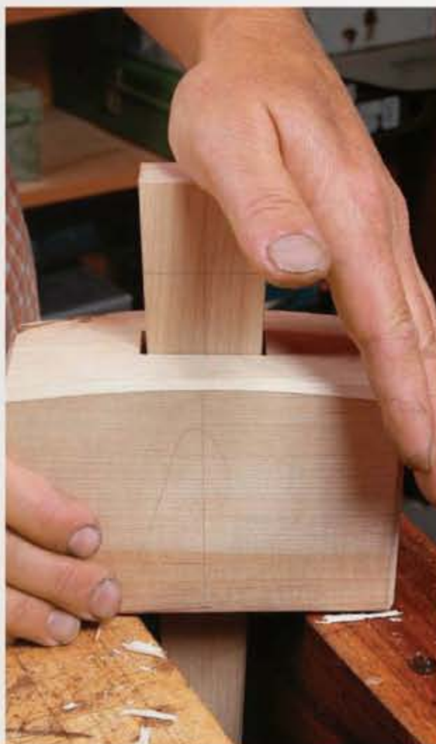
Taper until it's gapless. Dry-fit the handle and keep planing the tapers until it fits perfectly. The handle should seat in the mortise without any play and the end of the handle should protrude roughly 1½ in. from the top of the head.
