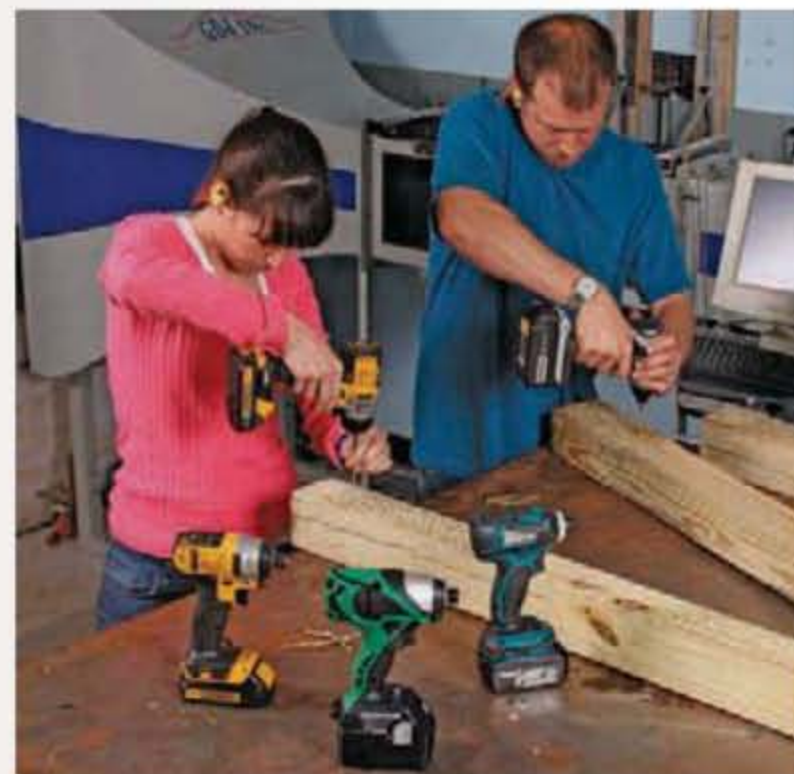
Drive till you drop. To gauge battery life, students measured how many 3-in. screws each driver could sink into pressure-treated pine on a single charge.
