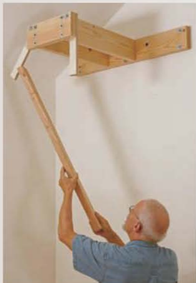
Safe storage for sheet goods. The restraining bars lift out of the way for loading. A lipped platform secures the sheets at the bottom.
