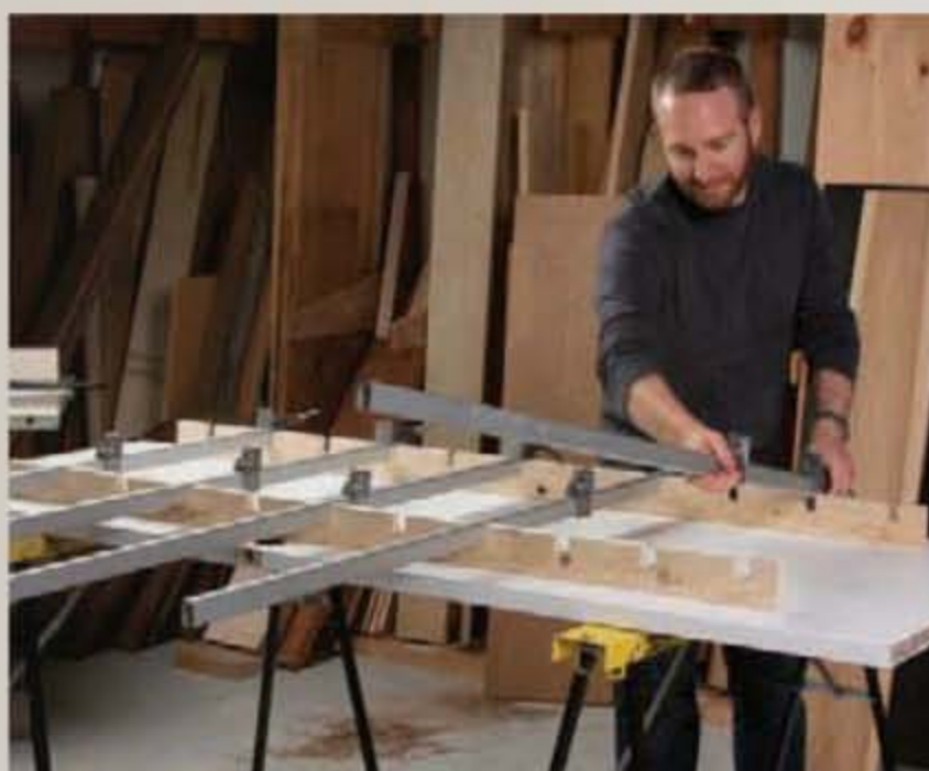
New life for an old door. The table should be long enough to glue up panels for case sides or tabletops. A hollow-core door is perfect because it is stable and lightweight.
