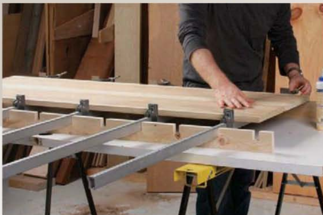
Quick-to-make clamp holders. Dadoed wood strips keep clamps in place for panel glue-ups.
