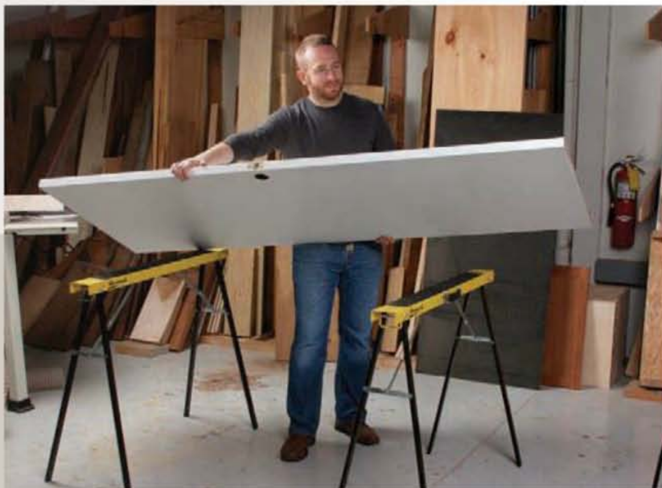
New life for an old door. The table should be long enough to glue up panels for case sides or tabletops. A hollow-core door is perfect because it is stable and lightweight.
