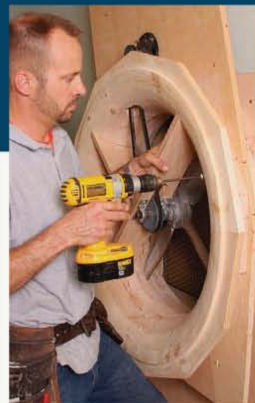
On goes the fan. Attach the bellmouth and fan to the motor-mounting plate with long screws.
