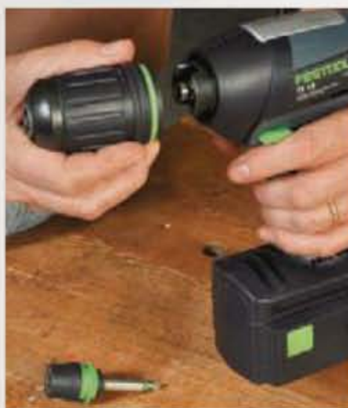
Double override. To override the impact function, add the override adapter to the Centrotec chuck or simply install the keyless chuck (shown).
