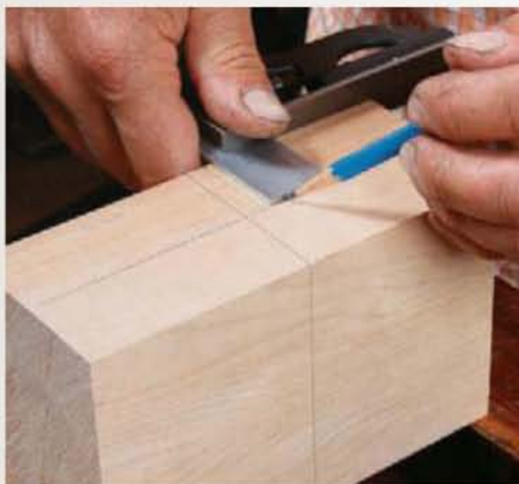
Start with centerlines. Mark them carefully and carry them around the head. Then lay out the ends of the mortise, plus the extra distance for the taper.
