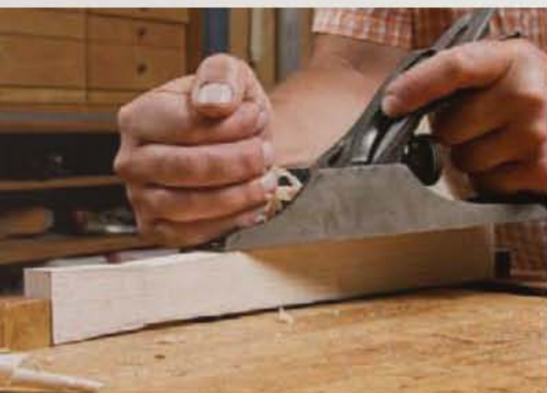
Take long, even strokes. Plane in toward the narrow part of the handle, stopping before the sole of the plane gets lifted by the bottom.
