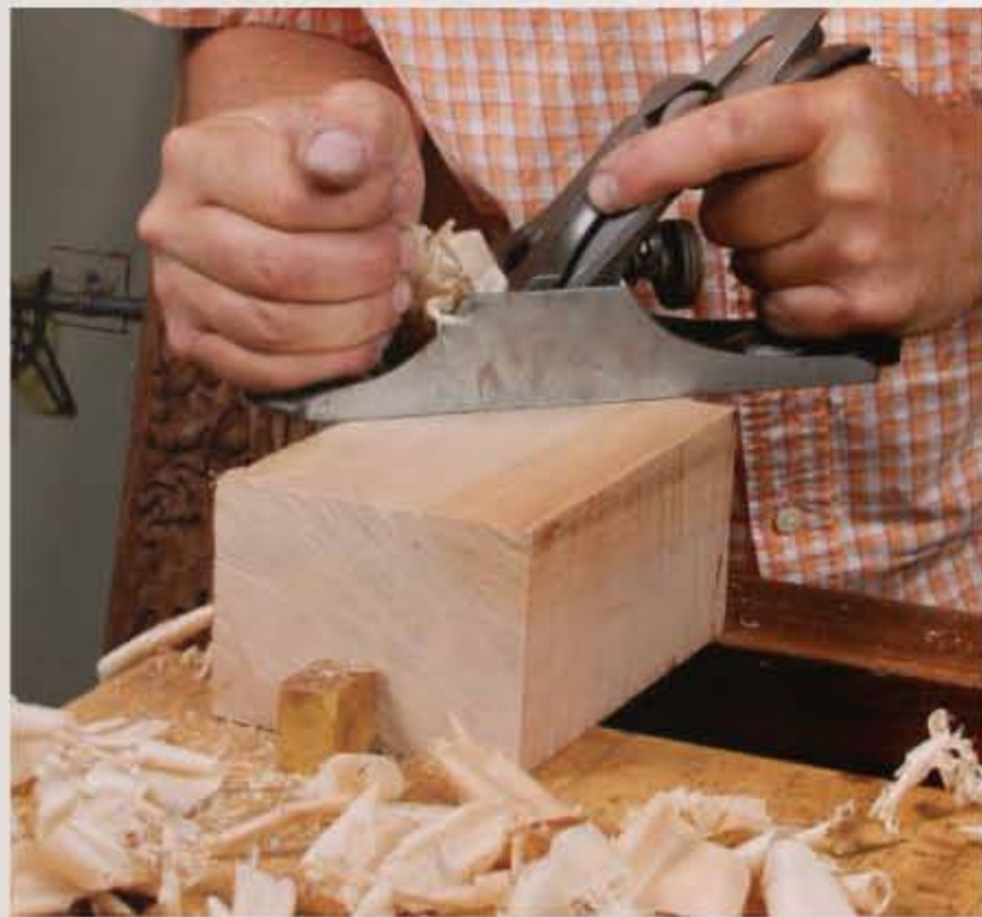
Flatten one face. Plane from side to side, taking even swipes. Check the face with a straightedge to make sure it's flat.
