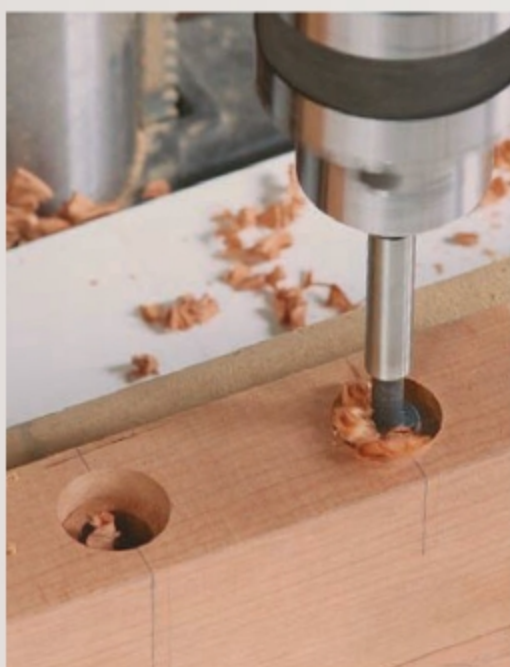
Two holes for a stepped mortise. Drill the larger hole first and then center the smaller bit in the dimple left by the larger one. Use a Forstner bit for both. Square them up, again starting with the bigger mortise before the smaller one.
