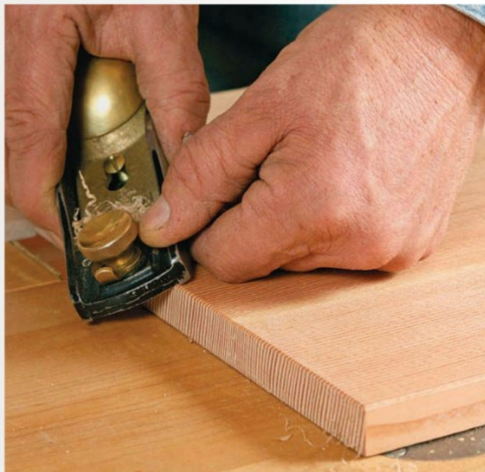
Finger guides. Tuck them underneath the sole of the plane and skew the plane toward the end grain for consistent, tearout-free chamfers.
