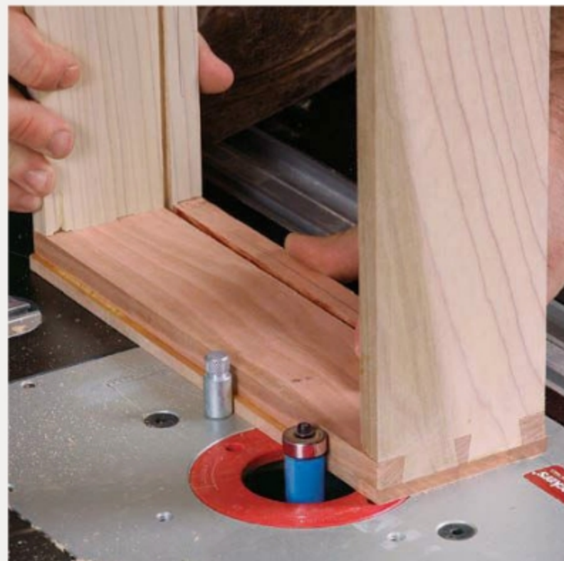
Just rout it flush. Routing is faster than a handplane and makes it easier to keep the edge square to the face. Do the ends before the long edges, and use a pin in your router table to help you enter the cut safely.
