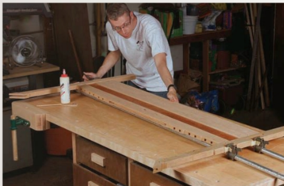
Glue the posts to the lower rails. The bottom panel is pre-finished and floats in the grooves (as does the top panel).
