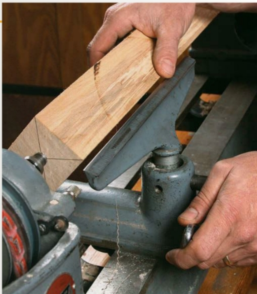
Keep it close. Move the tool rest about 1/8 in. away from the workpiece, and keep it at about the height of the centerline.
