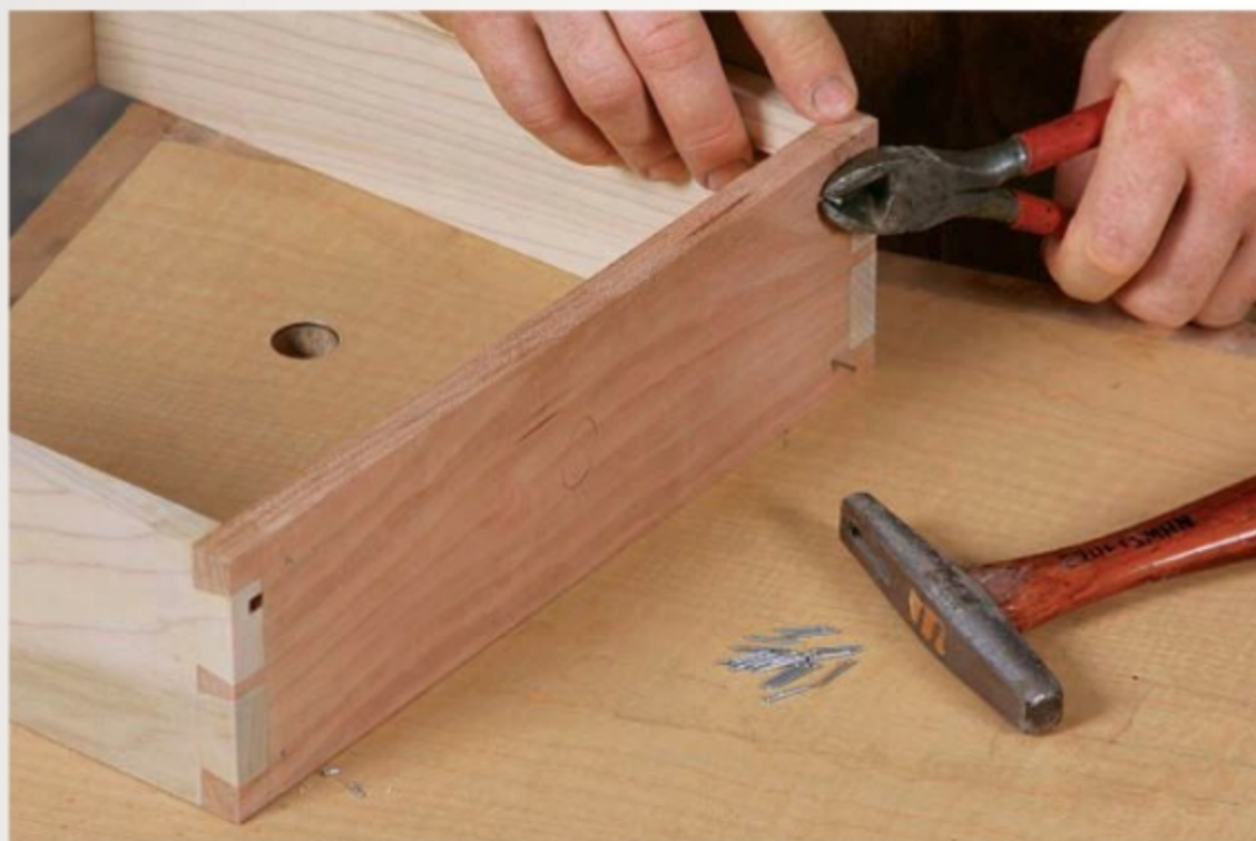
Brads lock it in place. Cut them off short and they'll stick into the front and prevent it from creeping under clamping pressure.
