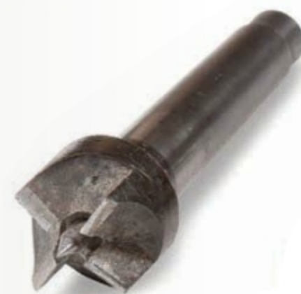
Tap the drive center. To mount a spur center, remove it from the lathe and pound it into the end of the workpiece to create a pattern of indents.
