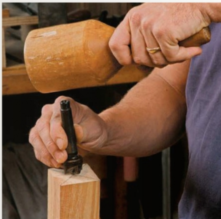
Tap the drive center. To mount a spur center, remove it from the lathe and pound it into the end of the workpiece to create a pattern of indents.
