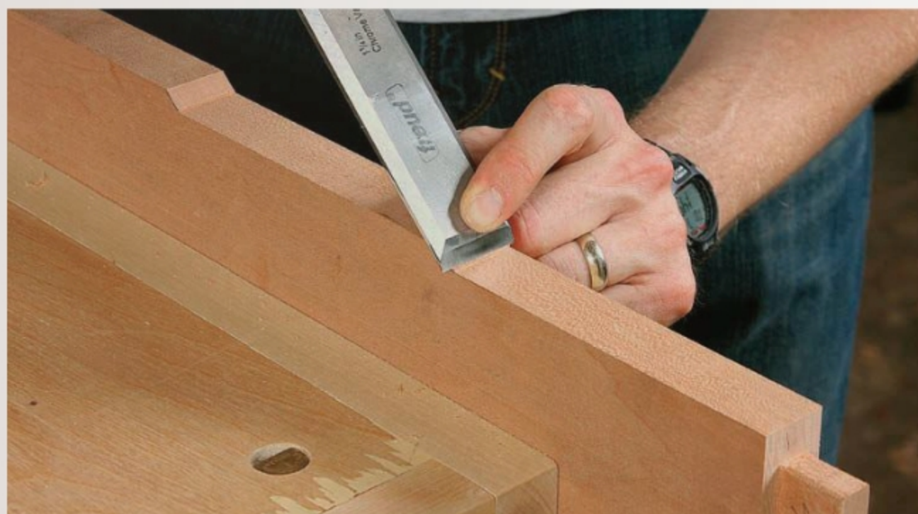
Clean up with a chisel. It's the best tool for the small transition. For the horizontal surface, use a block plane, switching to the chisel near the corner where the plane can't reach.
