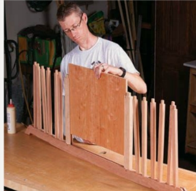
Put the spindles and panel in the top rail first. It's far easier to get the tenons into the stepped mortises now than trying to do it after the spindles' bottom tenons are locked into the mortises on the middle rail.
