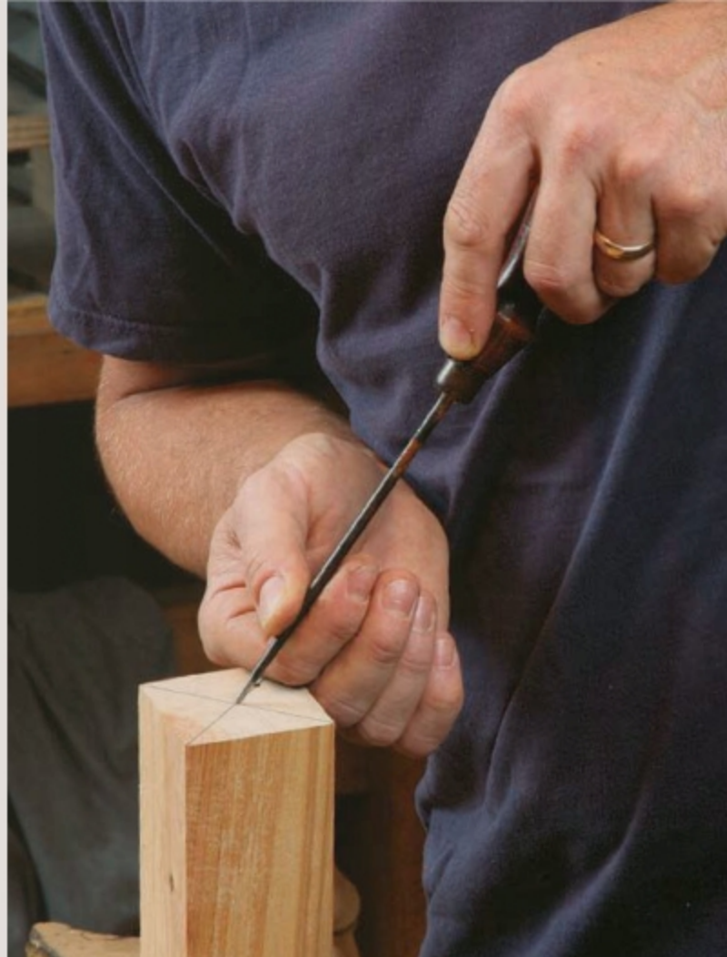
Punch the intersection. The indentation left by an awl helps locate the drive and tail centers.
