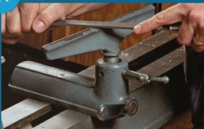
Remove dings and divots. Tools will glide more easily over a smooth, straight tool rest, so file it smooth and polish it with diamond plates or sharpening stones. Then coat it with wax.
