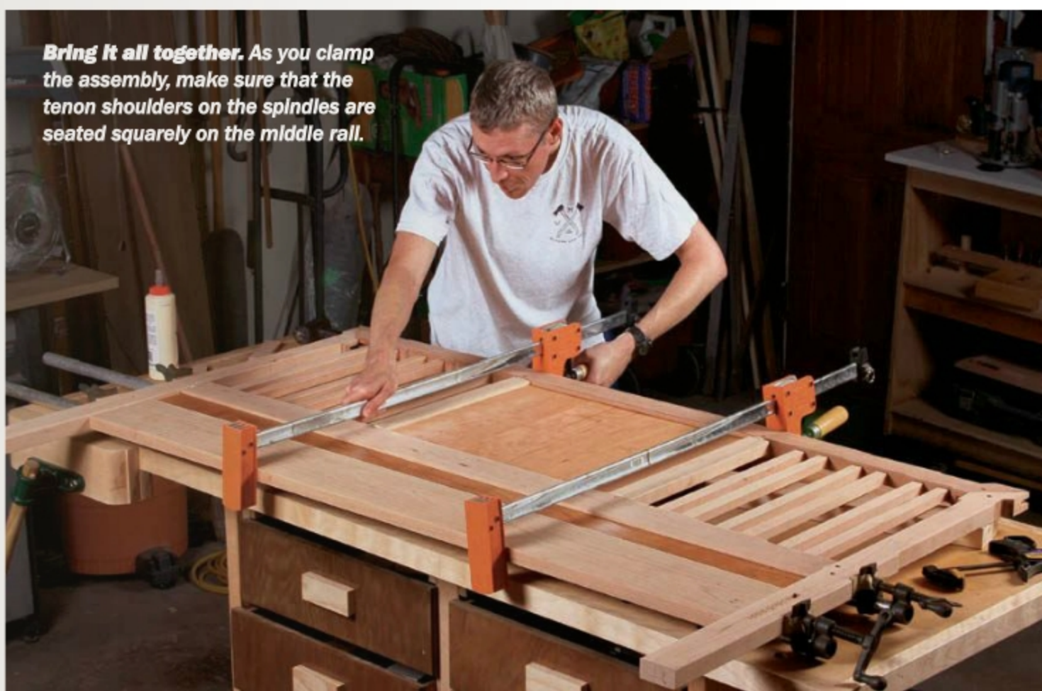
Glue the posts to the lower rails. The bottom panel is pre-finished and floats in the grooves (as does the top panel).
