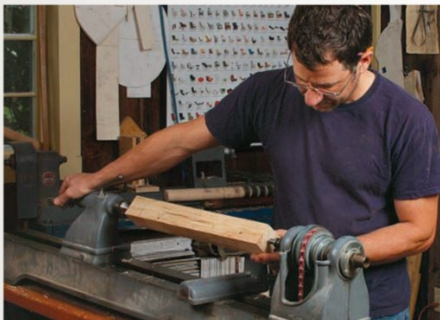
Line it up. The awl and spur marks will register the piece when you seat it between the drive and tail centers. Line everything up and then tighten the tailstock to secure the blank.
