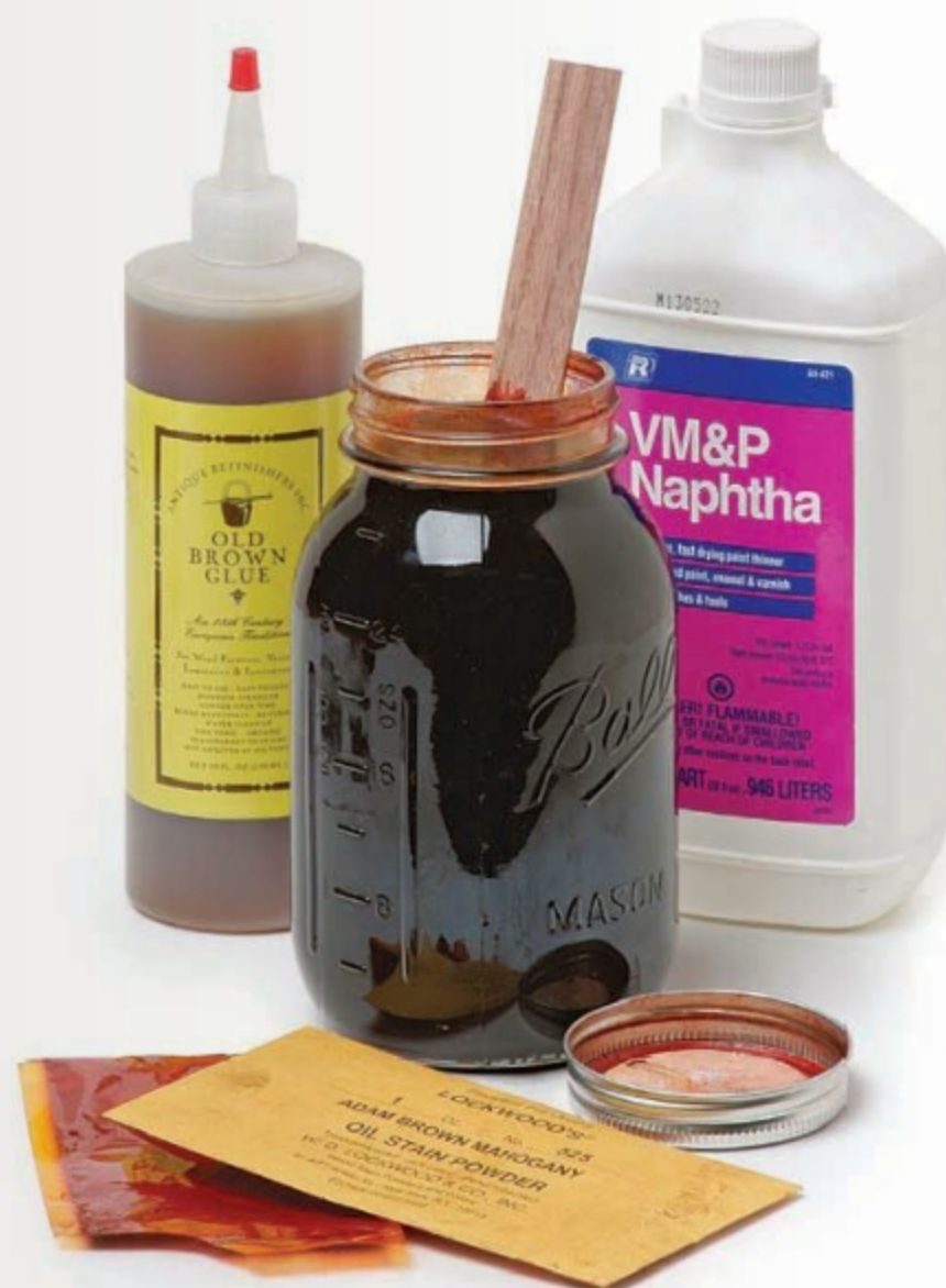
Oil-based is safe bet. The hide glue beneath veneered curves won't bubble or come up if an oil-based dye seeps through.
