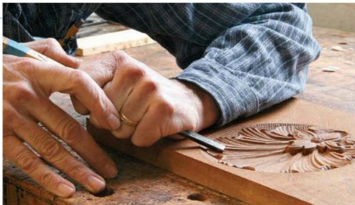
Lower is better. On his V-tool—and many others—Breed grinds down the steep factory bevels to create a long, curving underside that allows him to use the tool at a lower angle, thus increasing control.
