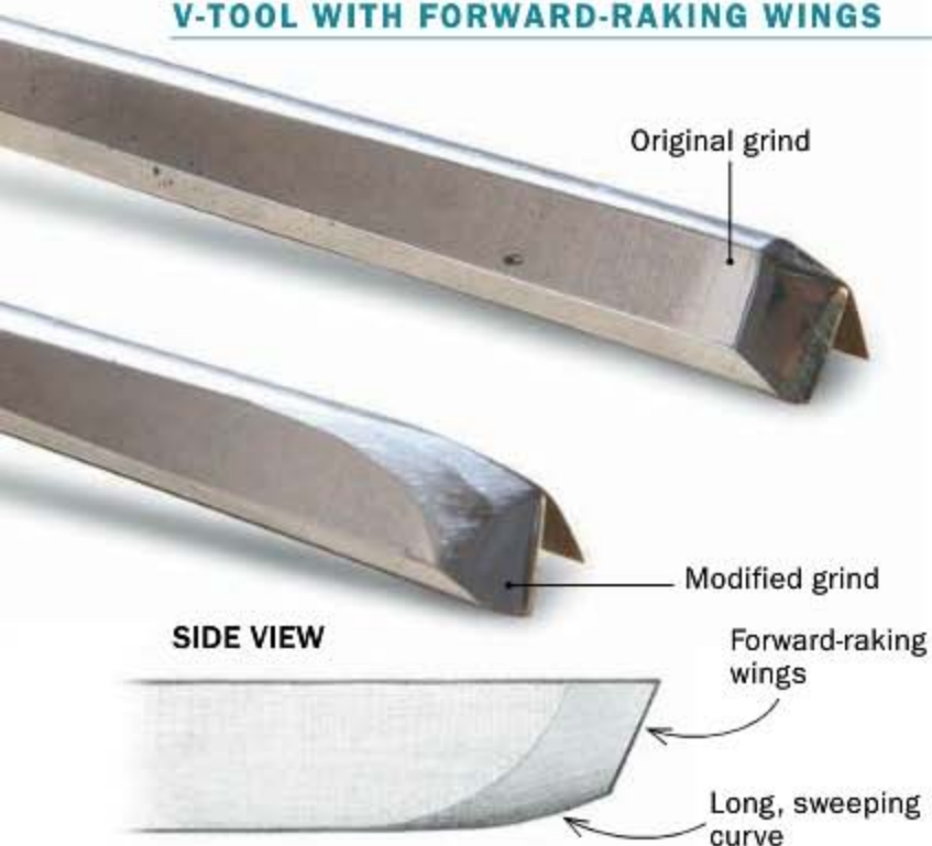
Lower is better. On his V-tool—and many others—Breed grinds down the steep factory bevels to create a long, curving underside that allows him to use the tool at a lower angle, thus increasing control.
