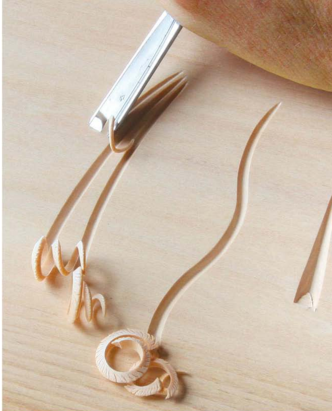
Revved up V-tool. Breed custom-grinds many of his carving tools to improve their performance. His modified V-tool cuts cleanly across the grain with minimal pressure.
