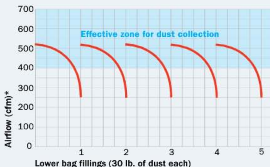
Test pipe doesn't lie. We measured airflow (in cubic feet per minute, or cfm) as we filled and emptied the lower bag many times.
