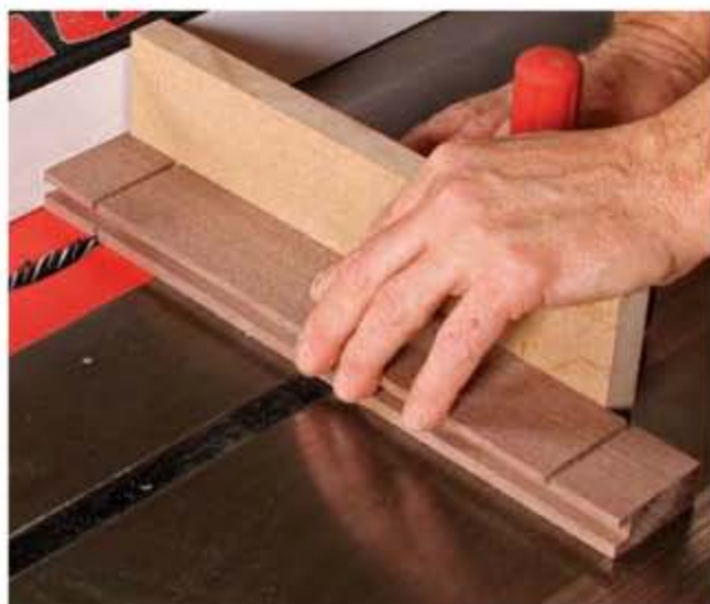
Cut the shoulders. Latta uses a miter gauge that's adjusted perfectly square to the blade. The rip fence serves as the stop.
