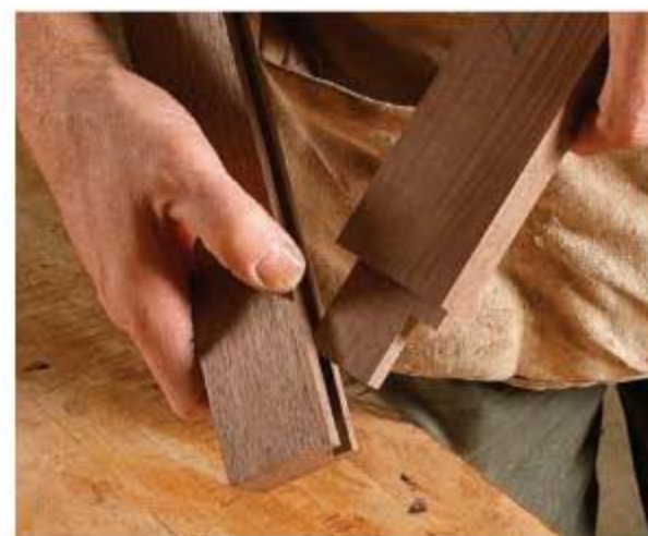
Too tight is just right. When machining the tenon, you want it to barely fit the mortise. Let it acclimate overnight, then fine-tune the fit with a rabbet or shoulder plane.
