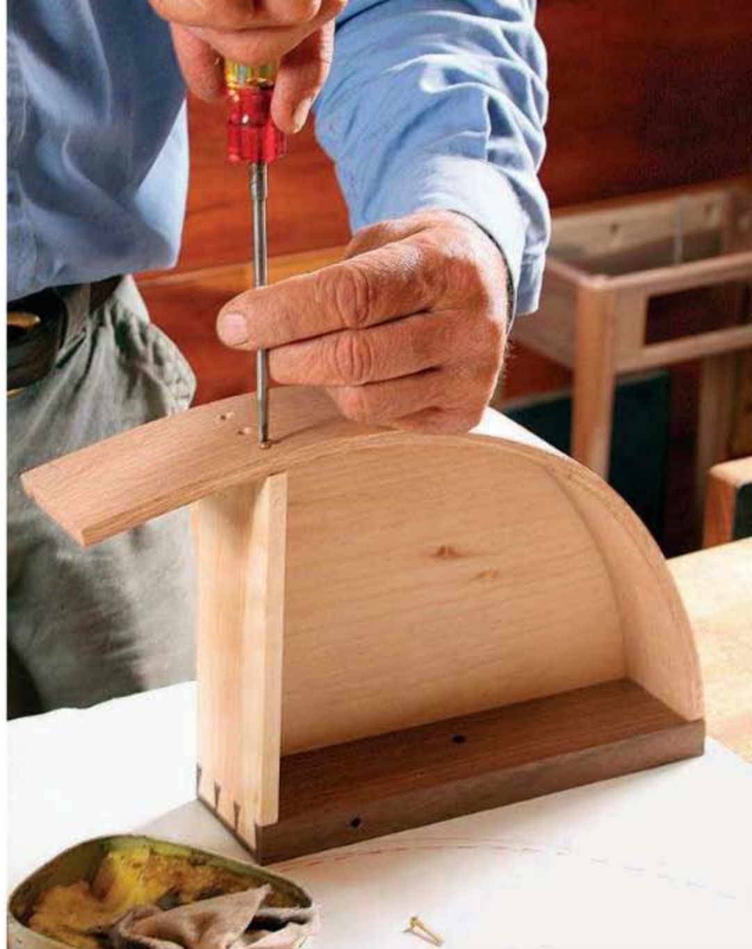
Rear reinforcement. Once the drawer box is glued up, screw the curved side to the straight side.
