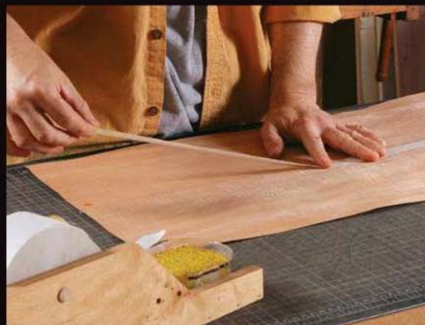
Then veneer tape. On the show face of the joint, Thibodeau applies a non-perforated paper tape with a water-activated gum adhesive (above). Let the sheet dry under a piece of MDF before removing the blue tape on the glue face (below).
