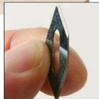
Cuts clean strips. Insert the stringing cutter, and you can slice your own stringing. The fence makes it easy to cut consistent widths.
