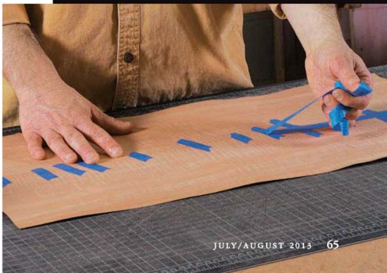
Then veneer tape. On the show face of the joint, Thibodeau applies a non-perforated paper tape with a water-activated gum adhesive (above). Let the sheet dry under a piece of MDF before removing the blue tape on the glue face (below).
