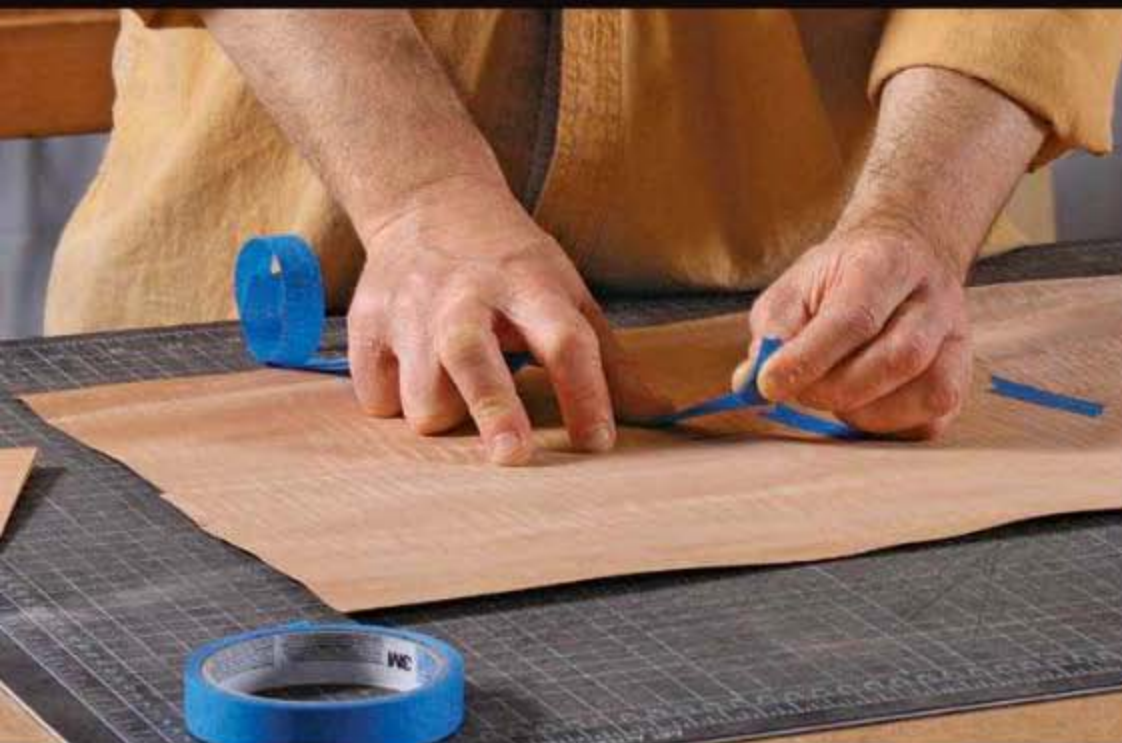
Blue tape first. Blue painter's tape has a little stretch to it. Pulled taut across the seam, it retracts slightly after being pressed down, helping to pull the joint tightly together.
