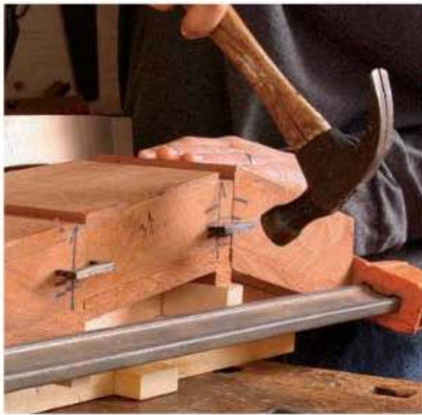
These dogs pinch. Faia spot-glued and clamped the parts, in sequence, on top of the supports and used pinch dogs to hold the components tightly together for shaping.
