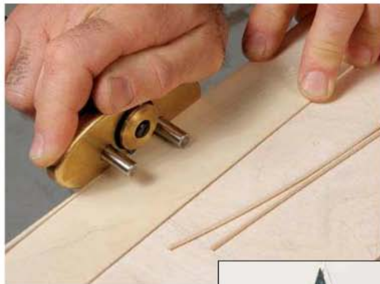
Cuts clean strips. Insert the stringing cutter, and you can slice your own stringing. The fence makes it easy to cut consistent widths.
