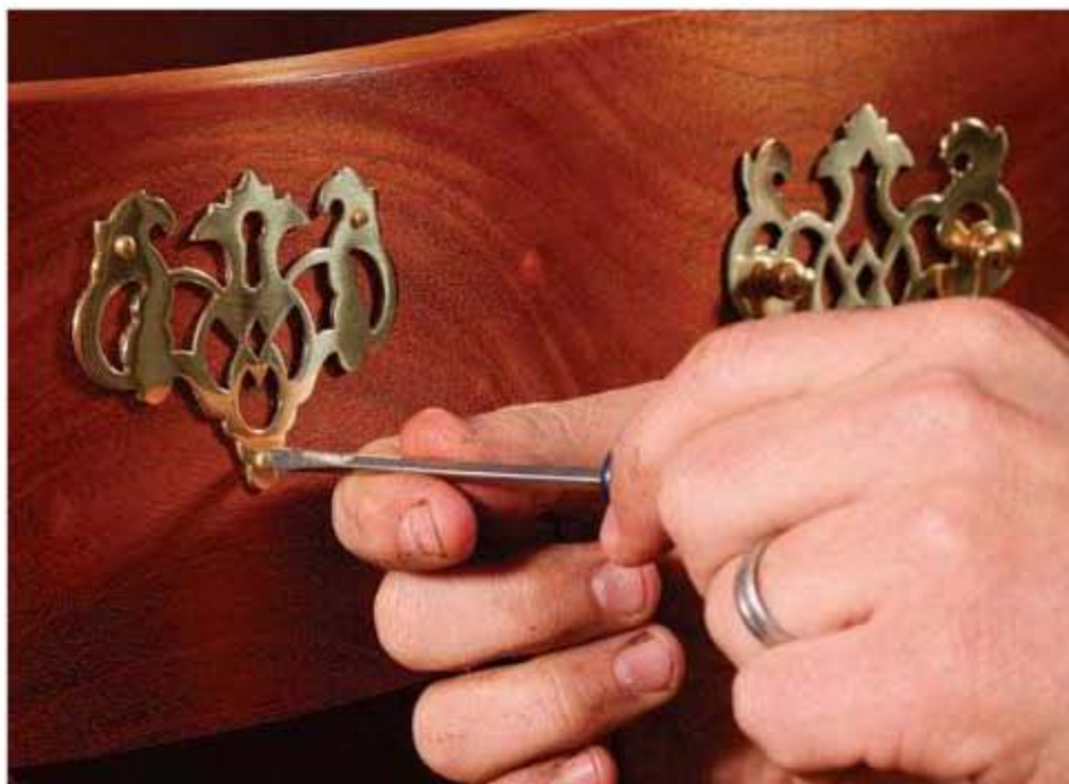
Pulls must be shaped to the case. Faia had to shape the brass hardware to fit the front. He placed each piece on a curved pine block and tapped it into shape using a deadblow mallet. And the pilot holes had to be perpendicular to the curve at each location, or the screw heads wouldn't sit flush.
