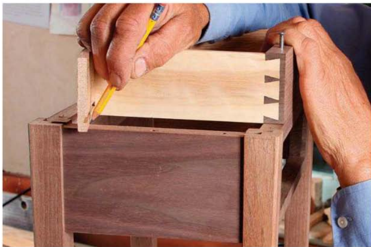
The side apron is the stop. To ensure that the drawer front is flush with the rails, place the drawer on top and insert the pin. Align the front flush, and mark the curved side where it meets the side apron. Cut the side with a handsaw and then trim the cut with a block plane until the drawer front is flush when it's closed.
