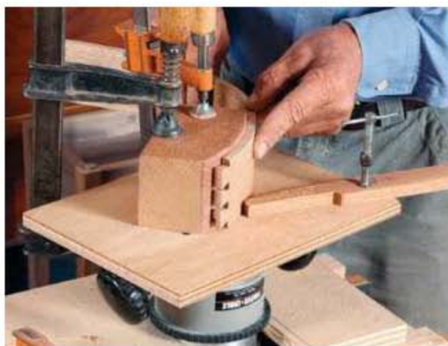
Rear reinforcement. Once the drawer box is glued up, screw the curved side to the straight side.
