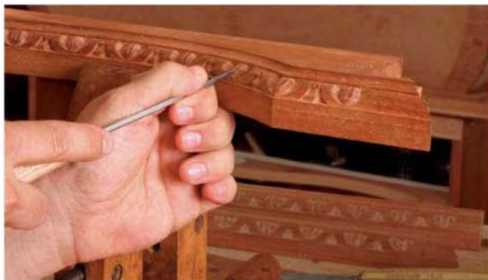
How do you like your eggs? Faia carved the egg-and-dart molding so that the corners would meet perfectly in the center of an egg. "It was time consuming," he said, "but in a piece of this magnitude, the details are everything."
