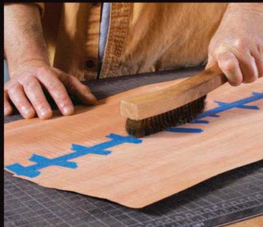
Burnish it. Thibodeau uses a brass brush to press the tape down firmly and ensure that it won't loosen.
