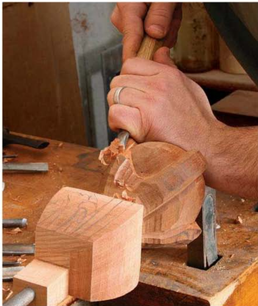
Boston ball and claw. With the side toes raking back, Boston feet are unique to the region. Faia borrowed the leafage pattern on the knees and transition blocks from an original piece at the Museum of Fine Arts Boston.
