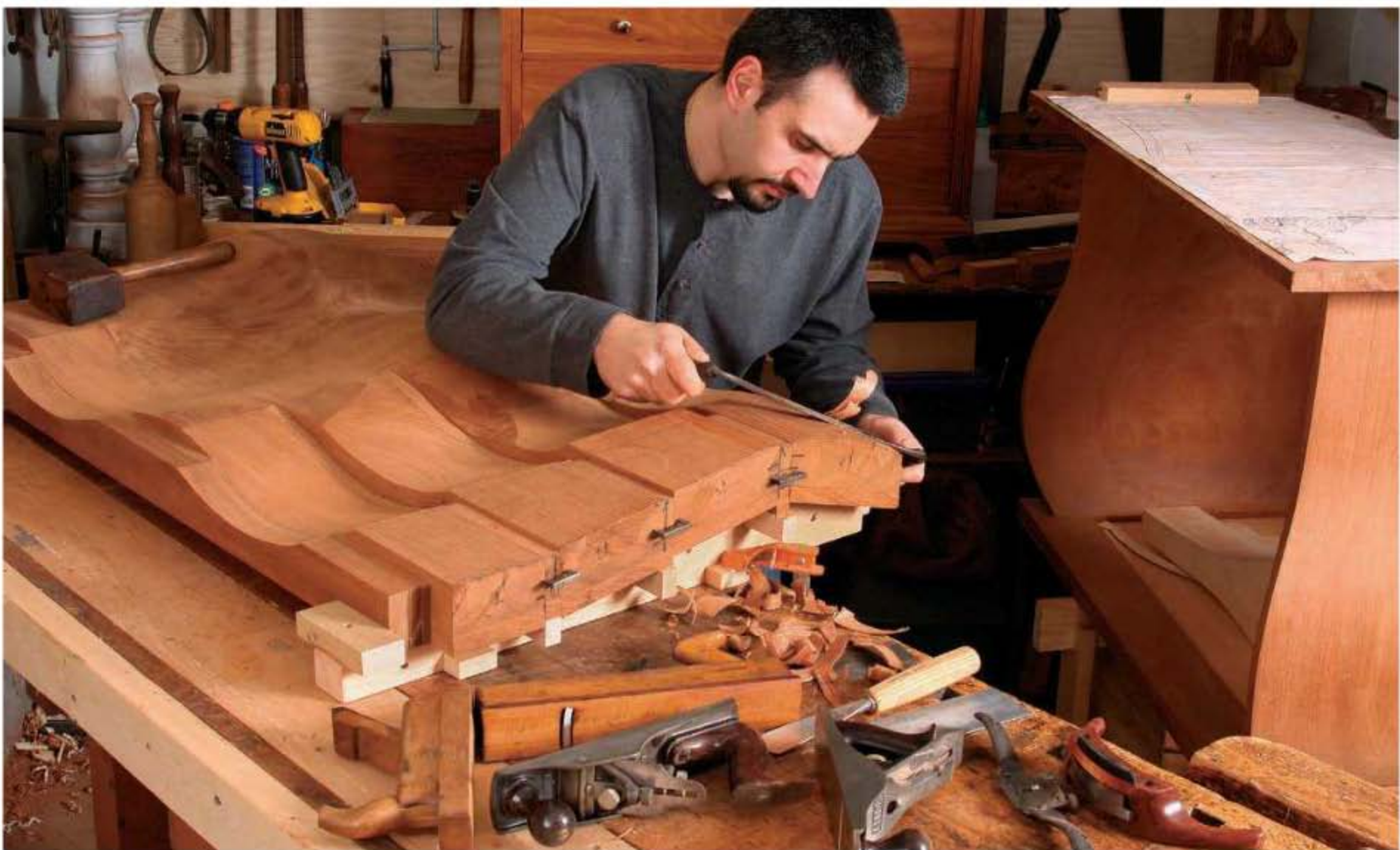
Heavy handwork. As with the case sides, waste material was hogged away with hand tools. The arsenal included a drawknife, chisels, a travisher, spokeshaves, and other handplanes. He started with the flatter sections at the outside of the drawer fronts.
