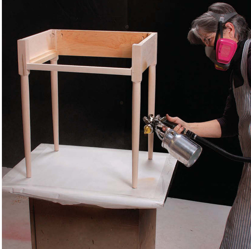
Work one side at a time. Spray the inner surfaces of the legs, using a medium-width spray pattern a little wider than the legs.
