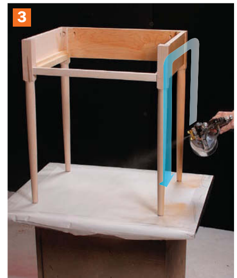
Work one side at a time. Spray the inner surfaces of the legs, using a medium-width spray pattern a little wider than the legs.
