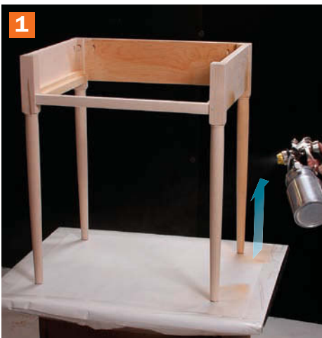
Then spray the outer face in one pass. Masaschi starts at the bottom of a leg, goes up and across the apron, then down the other leg with a continuous, smooth motion. Then she returns to the apron to spray any remaining dry spots.
