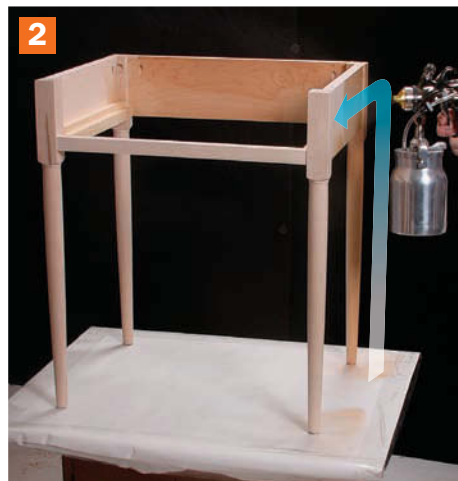
Then spray the outer face in one pass. Masaschi starts at the bottom of a leg, goes up and across the apron, then down the other leg with a continuous, smooth motion. Then she returns to the apron to spray any remaining dry spots.
