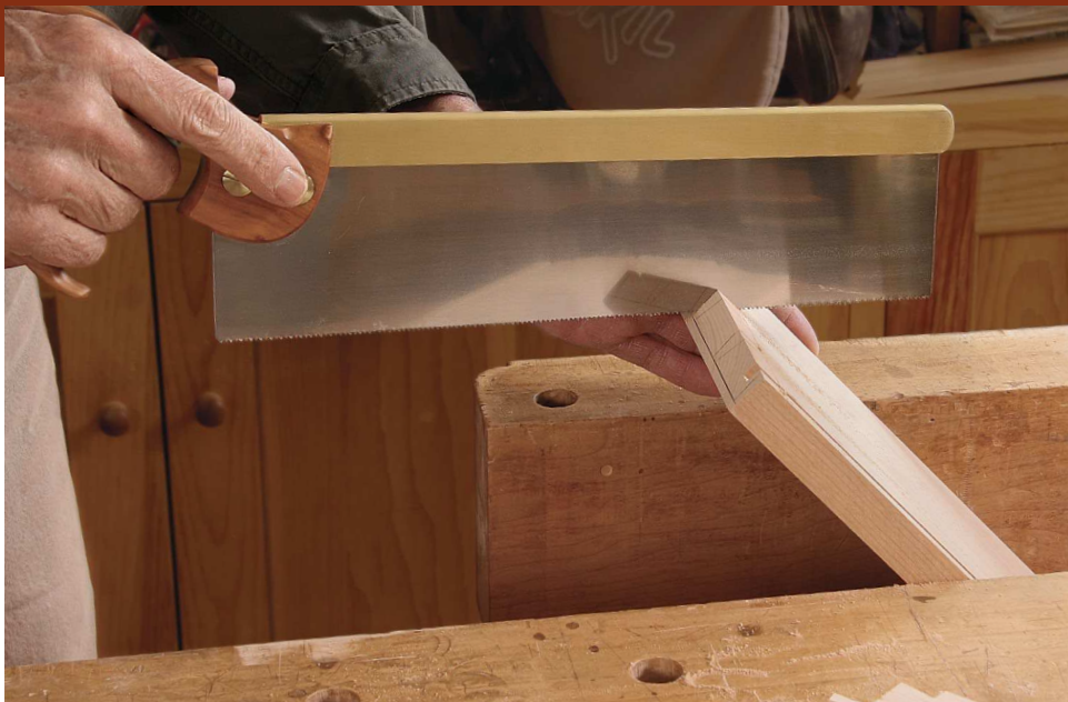
Careful kerfing. With the drawer front at 45° in the vise, saw along the cheeks of the pins until you reach the two scribed lines.
