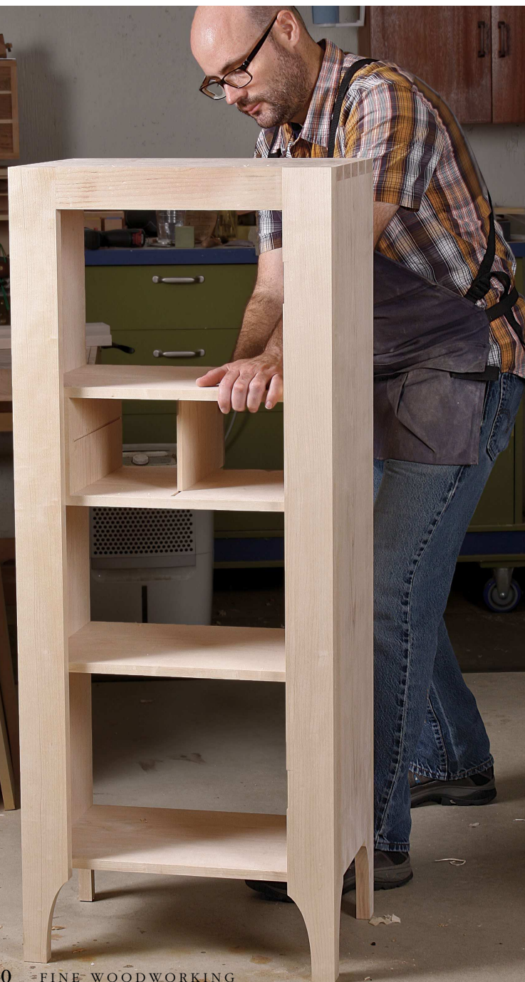
Ready for drawers. The left vertical divider slides up to the back of the face frame to close off the space between the divider and the cabinet side. The right divider stops \frac{5}{8} in. short of the shelf's front edge, creating space for the pulls. The horizontal divider stops flush with the right divider.
