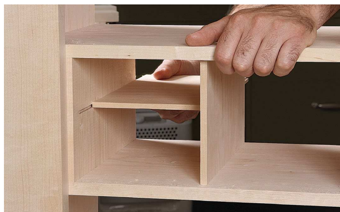
Ready for drawers. The left vertical divider slides up to the back of the face frame to close off the space between the divider and the cabinet side. The right divider stops \frac{5}{8} in. short of the shelf's front edge, creating space for the pulls. The horizontal divider stops flush with the right divider.
