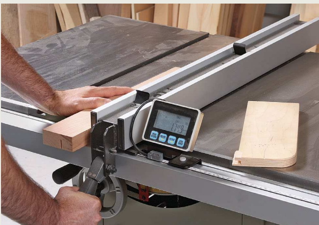
Digital fence readout. The distance from the blade to the fence is displayed to a thousandth of an inch, and it's accurate.
