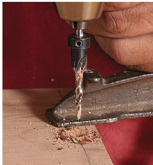
Countersink last. For flathead screws, use a countersink bit to cut a conical recess for the screw head.
