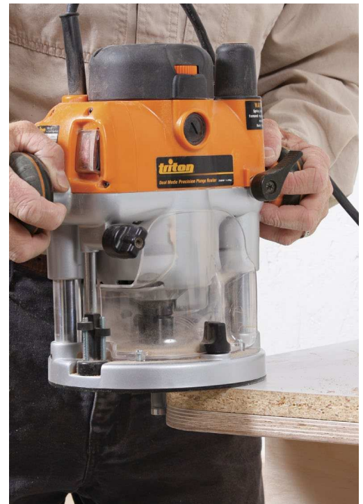
Add the countertop. After roughing out the corner radius of the countertop, screw it to the subtop from below, then rout the chipboard top flush to the subtop.
