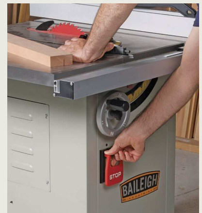
Long reach for the power switch. Located beneath the height adjustment wheel, the switch requires you to lean over too far.
