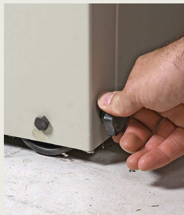
Built-in mobile base. Four wheels in the cabinet allow you to move the saw forward and back. The wheels lock with a few turns of a thumbwheel.
