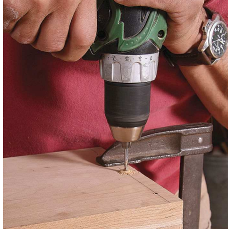
Pilot hole first. With the workpieces aligned and clamped, drill through the top board and into the bottom one with a bit sized to the root diameter of the screw.
