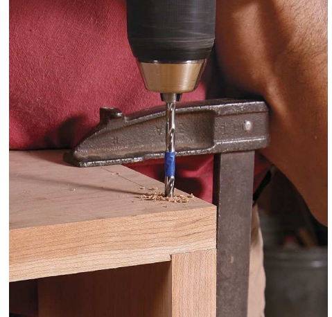
Clearance hole next. Drill into the pilot hole, using a bit just larger than the screw's thread diameter. A depth stop or gauge (in this case, tape) prevents drilling into the bottom board.
