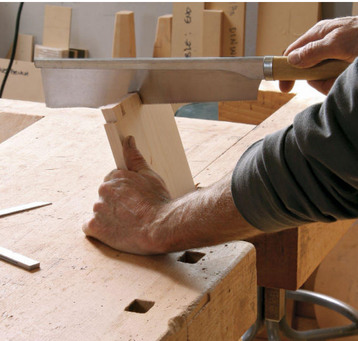
Handsaw follows bandsaw. Wurtz uses a handsaw to establish the angle at the bottom of the sockets. With the drawer side angled in the vise, a few strokes finish the work the bandsaw started.
