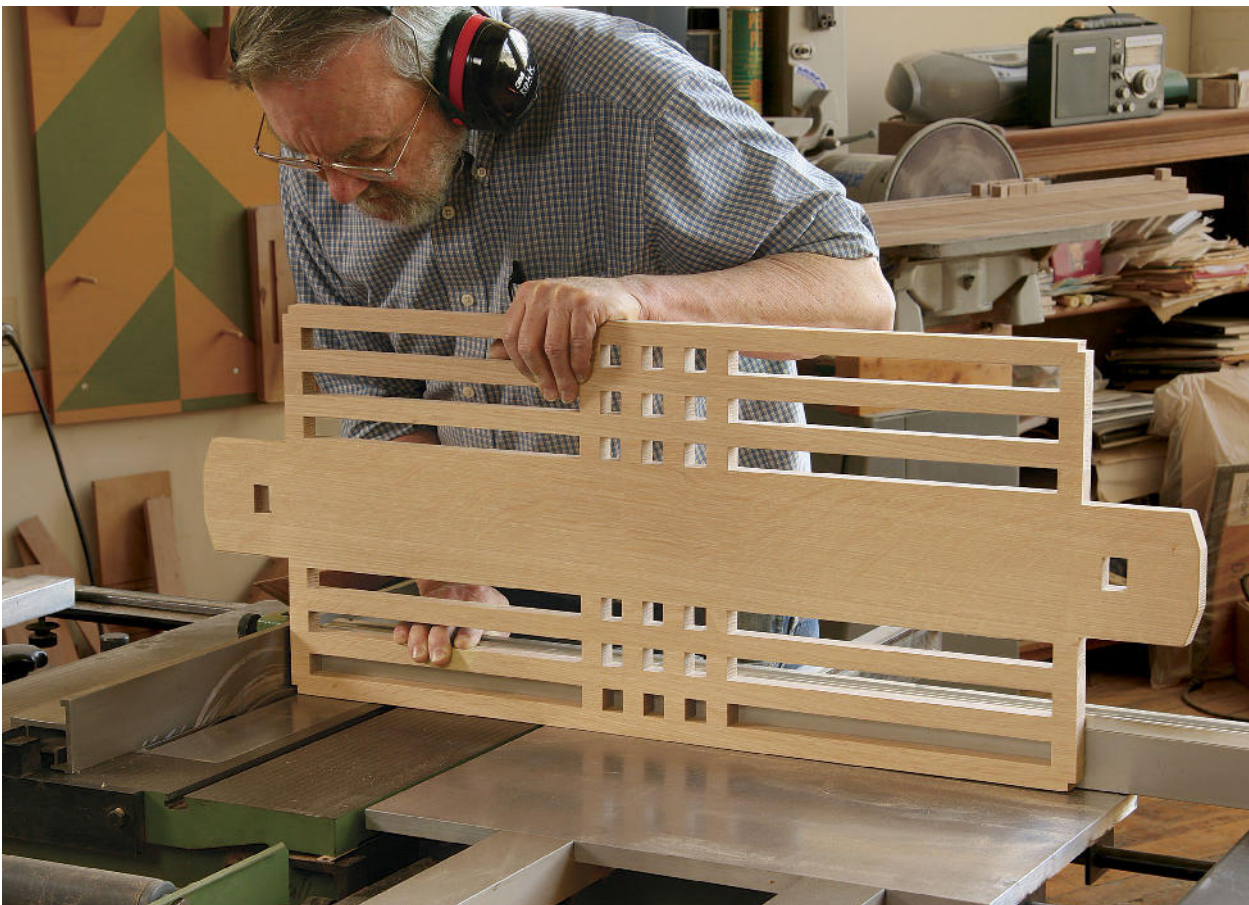
Notch the shelf. The shelf, which is fully housed in the dado in each end panel, is notched at the corners to hide the dado. Rodel cuts the \frac{1}{4} -in.-wide notches with a few passes of the saw.
