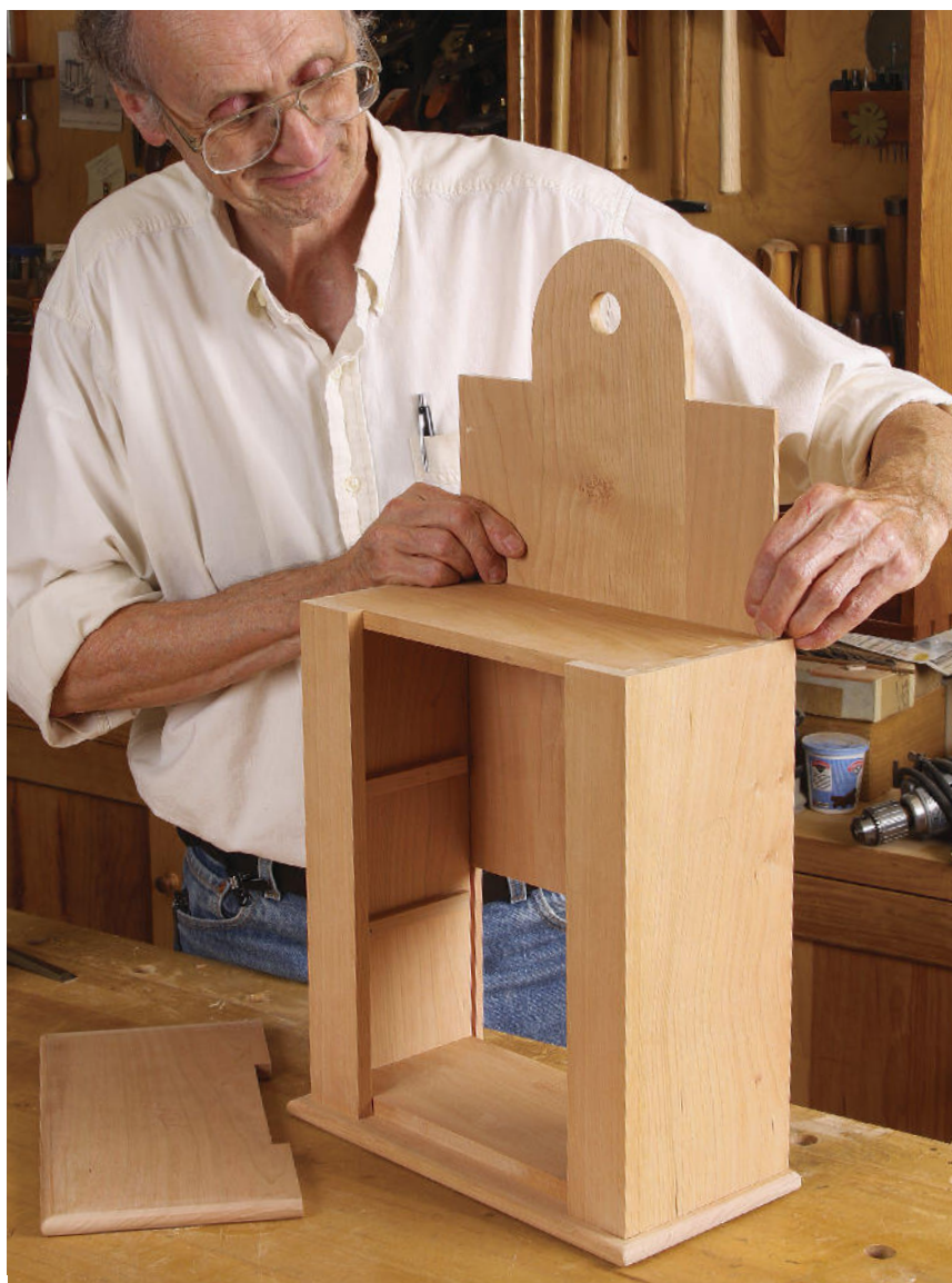
Secure the back. Slide the back into place, then add the top (above right). To attach the top, drive screws up through the case top. Then fix the back, screwing it to the case top (right) and case bottom.
