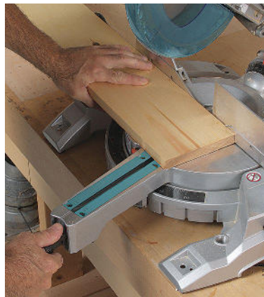
Convenient adjustments. Located on the front of the table, the miter lock is never far from your hand, and provides plenty of leverage to swing the saw for miter cuts in either direction.
