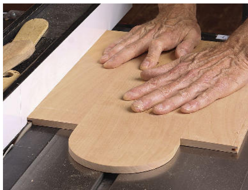
Two tongues. Two passes on the tablesaw—one with the back standing on edge—create the tongues on the sides of the back.
