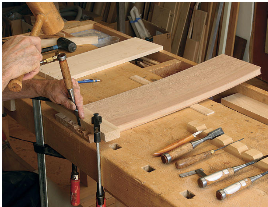
Flip the guide block. To chop the half-blind pins, use the same beveled guide block, but inverted. Support the far end of the drawer front on a scrap.
