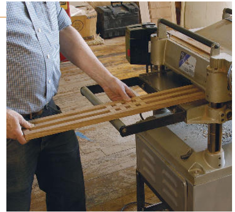
A little off the top. When the side assembly is cured, send it through the planer (or a thickness sander) to create a uniform surface.
