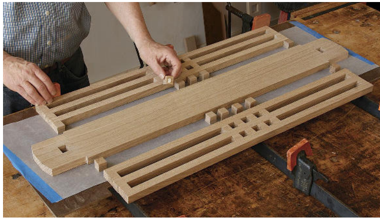
Finalize the grid. When gluing on the two gridded side panels, be careful to align their ends with the shoulder of the notch on the center board. Before this glue-up, make the angled cuts on the ends of the center board.
