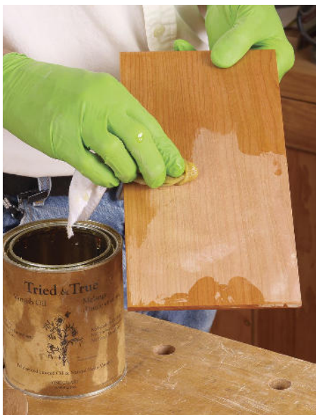
Diminutive frame and panel. After applying finish to the \frac{1}{4} -in.-thick door panel, drop it into place as you assemble the door frame.
