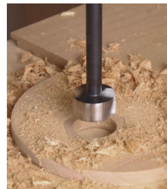
Circle session. A Forstner bit in the drill press cuts a clean hanging hole in the back.
