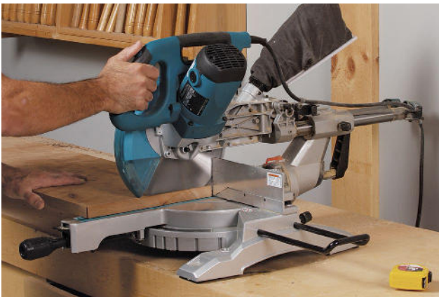
Wide boards are no problem. You can cut clear through boards up to 12 in. wide with the blade set for a 90° cut. Angled for a 45° miter, the saw can still get through boards 8½ in. wide.
