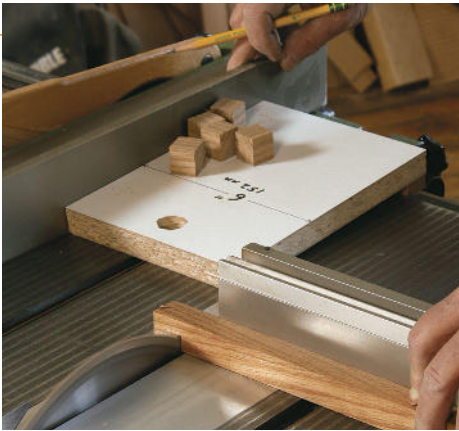
Block factory. To make the gridded side panels of the shelf, Rodel cuts \frac{3}{4} -in.-wide strips. Then he cuts blocks from the strips, using a scrap against the rip fence as a stop.
