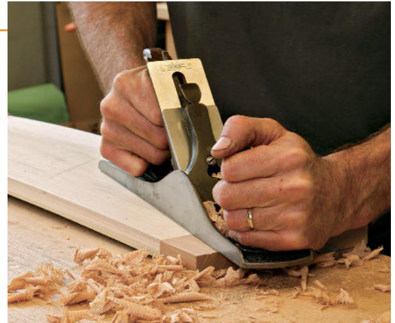
Solid ends on a core of plies. Use biscuits to attach the solid end blocks to the core of poplar plies (left). After the glue-up, plane and scrape the blocks flush to the core (above).
