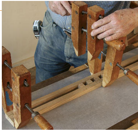
One at a time. Rodel builds the grid one row of blocks at a time on a sheet of waxed paper taped to Masonite. After 15 minutes he'll add another strip and set of blocks.
