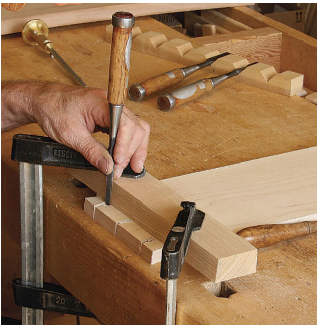
Beveled block guides the chisel. An angled guide block ensures the correct slant of the chisel as well as a clean baseline.
