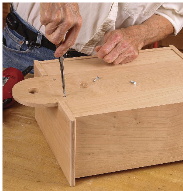
Secure the back. Slide the back into place, then add the top (above right). To attach the top, drive screws up through the case top. Then fix the back, screwing it to the case top (right) and case bottom.
