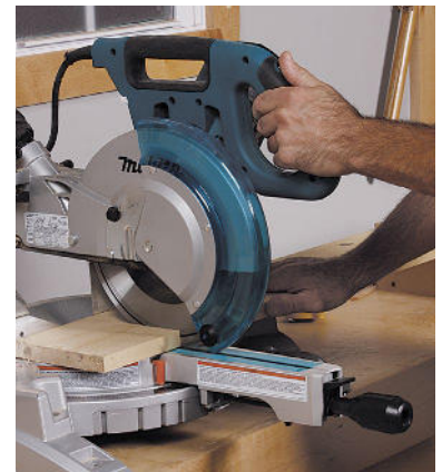
Right for lefties, too. Oriented vertically and clear of the blade housing, the handle is just as easy to operate with your left hand as it is with your right.
