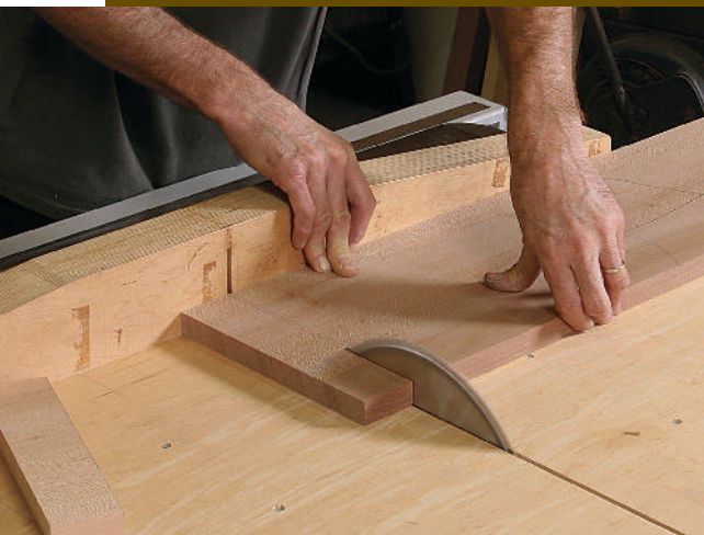
Crosscut the end blocks. Before resawing the show wood into veneers, crosscut the plank to produce the solid blocks for the ends of the drawer front.
