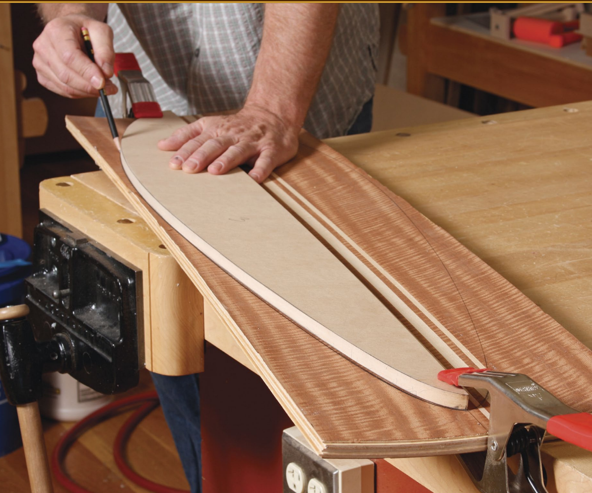
Lay out the deck. After putting a centerline down the blank, trace the outline onto the blank. Gochnour uses a half-template made from MDF to ensure both sides are symmetrical.
