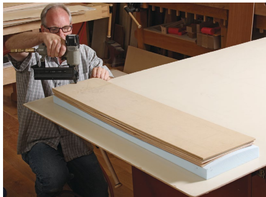
Stake the plies. To keep the packet from shifting, place a \frac{1}{4} -in. MDF platen on the stack and secure each end of the packet with a brad nail to the form.
