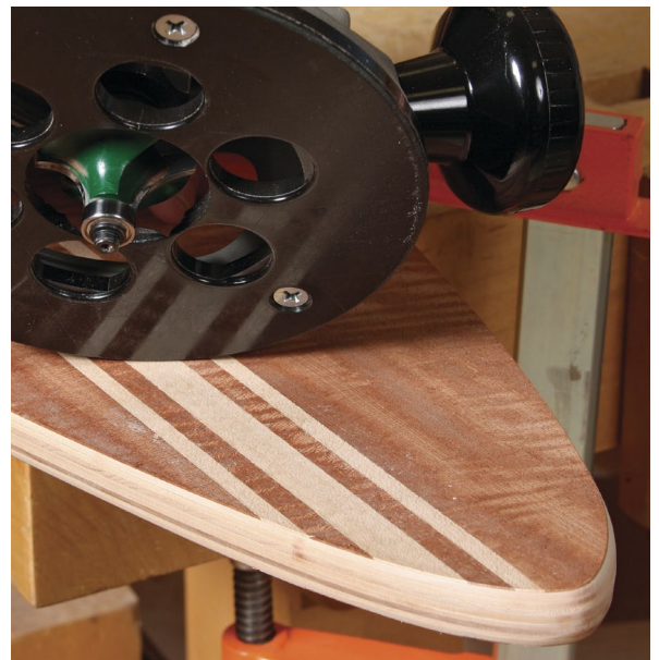
Cut it to shape. Cut the deck shape from the blank at the bandsaw (left), leaving the pencil lines. Then use a spokeshave or sandpaper to level the edges to the traced lines. Ease the top and bottom edges of the deck with a bearing-guided roundover bit (above).
