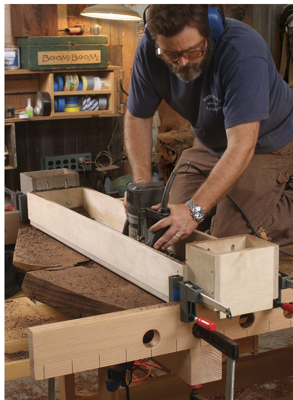
Aggressive and durable. With Infinity's new planer bit in your router, you can hog off an impressive amount of wood quickly, speeding up the job of flattening a slab.
