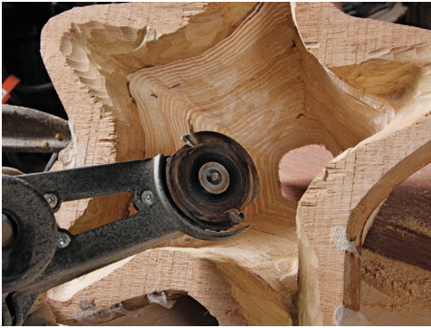
Start with a mini grinder. The tool hogs away material to bring the walls to rough shape.
