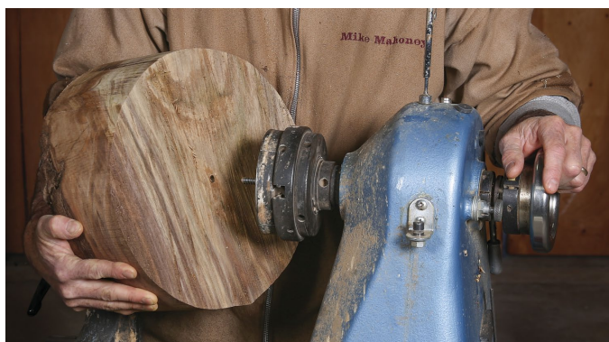
Mount the blank on a screw center. This is the simplest and safest way to mount a rough blank, but it's important that the blank be in solid contact with the chuck. Use the tailstock, too.
