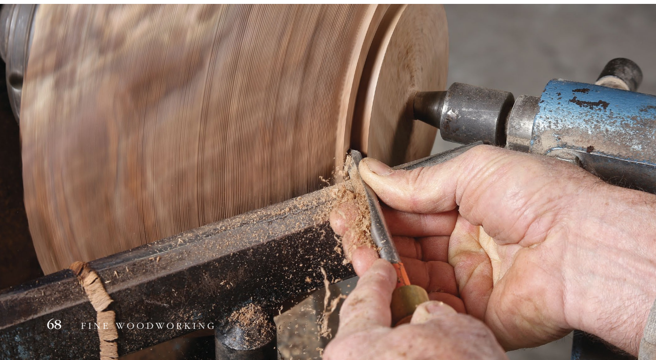
Mount the blank on a screw center. This is the simplest and safest way to mount a rough blank, but it's important that the blank be in solid contact with the chuck. Use the tailstock, too.
