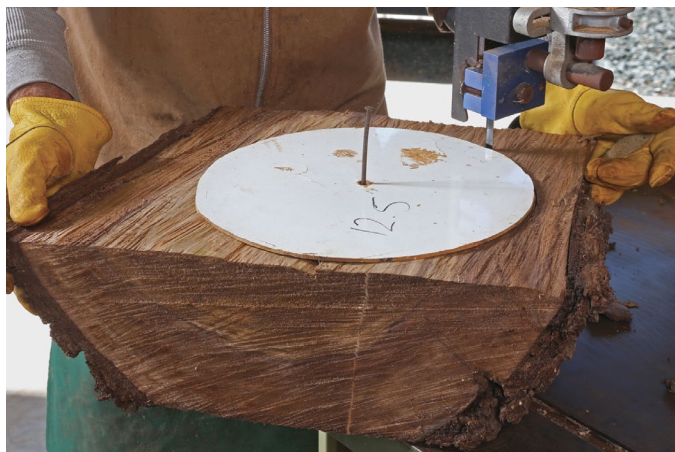
From log to round blank. Mahoney always begins with green wood cut from a section of trunk or branch. At the bandsaw, he roughs out the bowl, following a plywood template secured with a nail.
