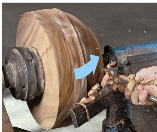
Mount the blank on a screw center. This is the simplest and safest way to mount a rough blank, but it's important that the blank be in solid contact with the chuck. Use the tailstock, too.
