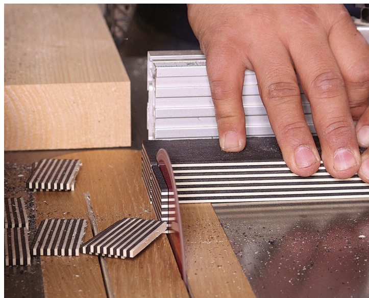
Chips from a brick. After ripping the brick to width, crosscut \frac{1}{8} -in.-thick chips from it. Use a zero-clearance insert, a stop block, and the miter gauge.
