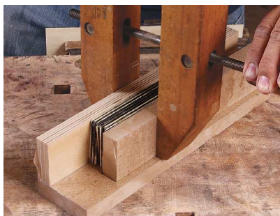
Simple jig for glue-ups. Roman coats the outer layers of veneer with liquid hide glue, then uses an L-shaped MDF jig to keep the parts aligned when clamping.
