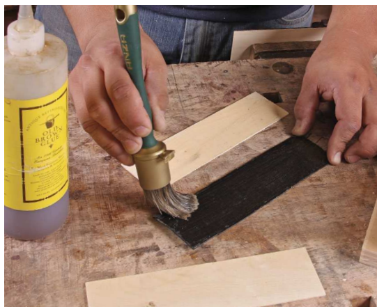
Simple jig for glue-ups. Roman coats the outer layers of veneer with liquid hide glue, then uses an L-shaped MDF jig to keep the parts aligned when clamping.
