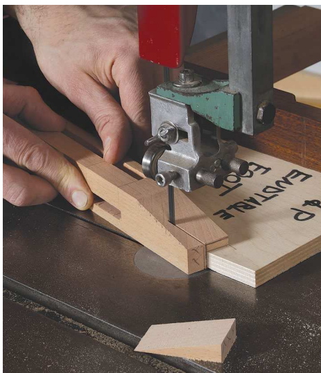
Take care of the feet. Cut the tapered feet at the bandsaw. A simple jig ensures consistent cuts.
