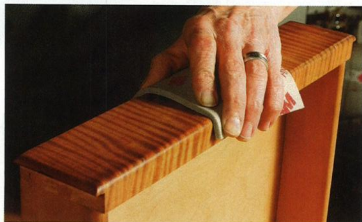
Sanding sponges. Less flexible than the other products, sanding sponges are good for gentle curves and can be washed out after use.
