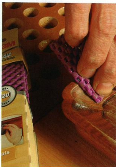
Foam mesh. 3M's Sandblaster is a drawer-liner type of foam mesh coated with abrasive. It can be folded over to reach into tight corners or wrapped around curves.
