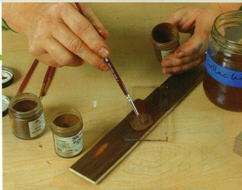
Practice patch. Make a similar burn-through on a scrap of the same plywood. Mix touch-up powders with thinned shellac to match the color of the face veneer and hide the sanded-through spot.
