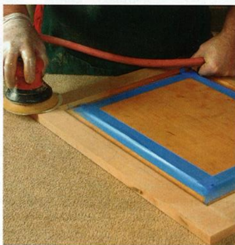
Protect the finish. After the frame has been glued together, you probably will need to flush-sand the joints. To avoid damage from the sander, tape off the nearby sections of panel.
