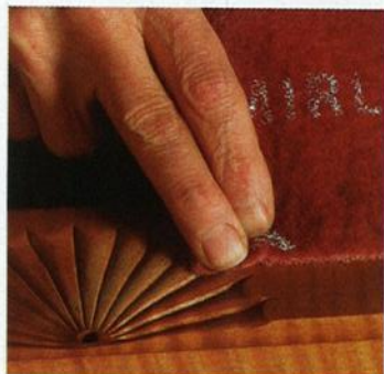
Abrasive pads. These pads come in a variety of grits and are thin enough to get into carvings.
