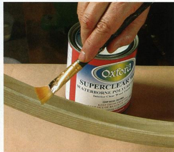
A choice of brushes. When applying a water-based finish to narrow surfaces, use either a foam brush or an artist's brush with man-made bristles.
