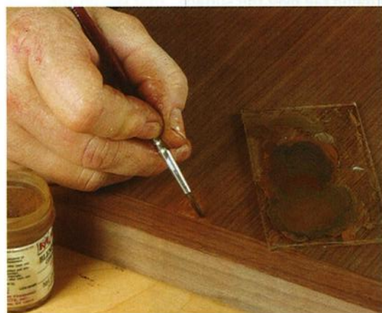
Practice patch. Make a similar burn-through on a scrap of the same plywood. Mix touch-up powders with thinned shellac to match the color of the face veneer and hide the sanded-through spot.
