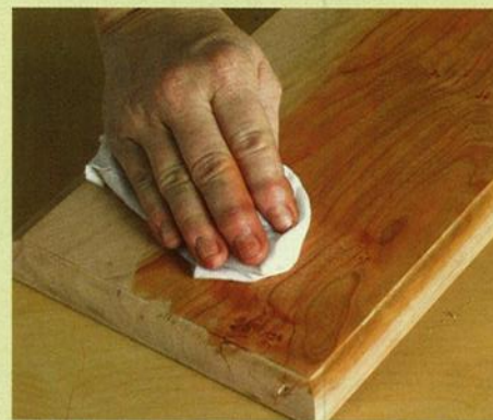
Check your work. Wipe on mineral spirits before applying the finish. This will reveal any lingering scratches or patches of tearout.
