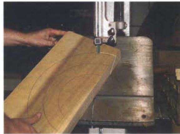
Carefully cut the semicircles from each half with your band saw table set at 45°.
