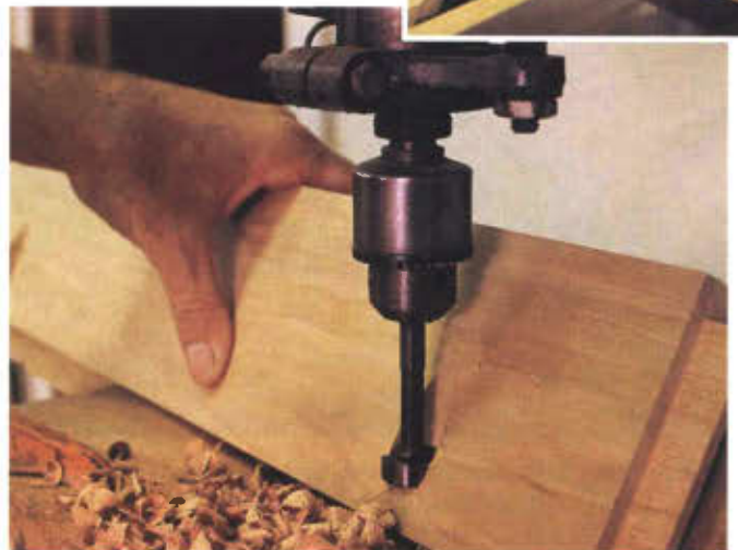
4. Drilling pin-hole for gate (left). 5. Below, detail of the angled screw pockets being drilled in apron for top attachment. 6. Inset shows jig used in making finger joints for gate joint in apron.
