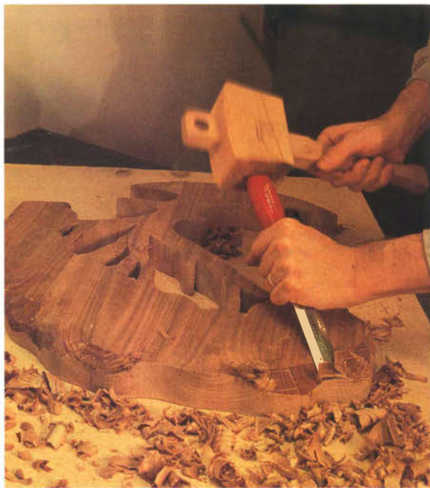
(Photo 4) Using a mallet and ¾" carpenter's chisel to knock the edges off the tree canopy and rough-out the canopy edges.
