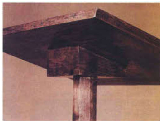
Above, top and lip with beveled edge. Below, connecting box assembly with top and column.
