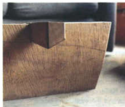
(Above) The sturdy base rest is only 16" long, but it easily handles the top's weight. (Below) The longer, 18" arm is set into the massive plank to support the top.
