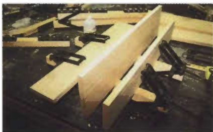
1. Preparing to glue-up solid material for the drawer fronts.
