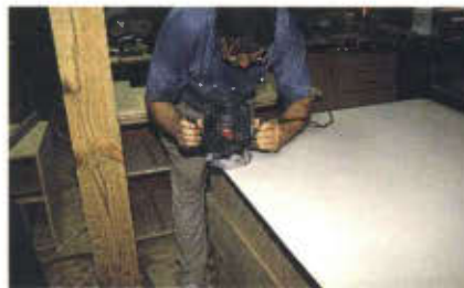
25. Laminate trimming bits fit in almost any good router.
