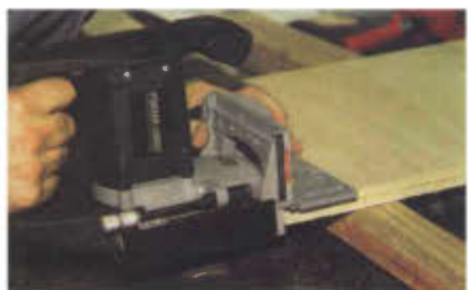
3. Cutting biscuit slots on one side of the corner.
