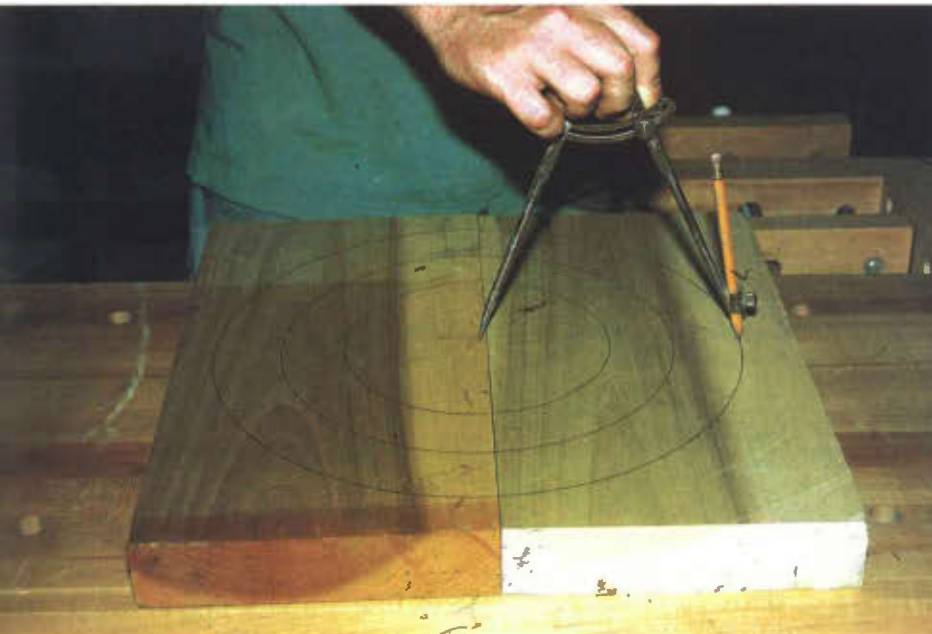
Using a compass, draw concentric circles on a single square. The number of circles depends on how deep you want to make your bowl.
