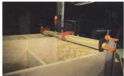
6. Glue-up requires a number of clamps, though not nearly as many if the entire job were straight glue and biscuits.
