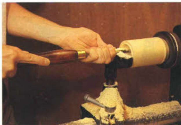
Finishing hollowing using the 1/2" scraper.
