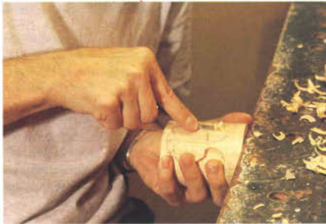
Paring down the background using the edge of the workbench as support.
