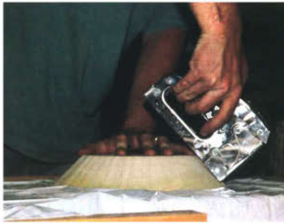
(Photo 3) Stapling the glued circles on the outside face allows an adequate gluing process and easy gluing on the stacked rings.
