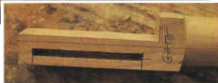
11 & 12. Before and after views (above and right) of cutting away the excess material from the gate leg so it will close accurately against the apron rail.
