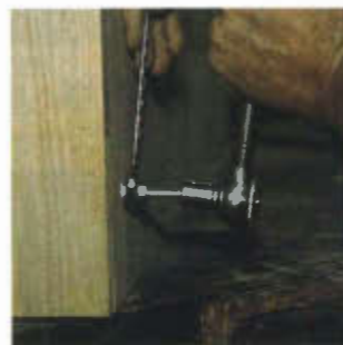
12. I had trouble getting the brass inserts in with a large screwdriver, and didn't have the tool meant for doing the job. Using a 2½" x ⅝"-18 hex head bolt and two nuts, plus two washers, makes a driver tool that works beautifully, smoothly and quickly with two wrenches.
