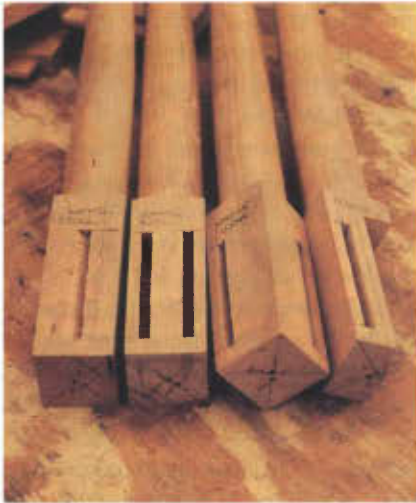
10. Mortises shown ready to receive apron tenons.
