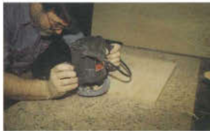
14. Edging the drawers using a roundover bit.
