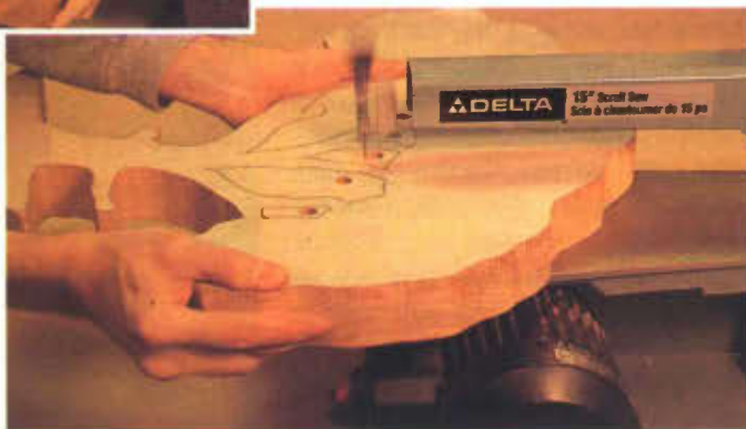
3 Using the scroll saw to cut the waste out from between the branches.
