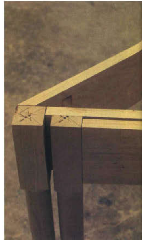
Photo at right shows finished assembly of gate leg and apron in closed position. The next step is staining and finishing.
