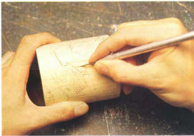
Incising stop-cuts around the detail before paring background.
