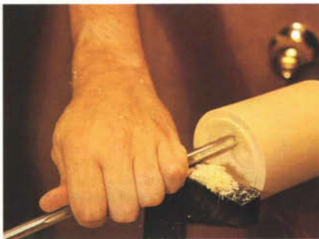
Hollowing, using the 1/4" gouge.
