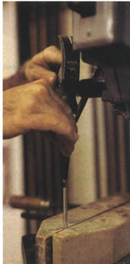
14. Flaring the top of your home-made pin for hinging the finger-joint gate.
