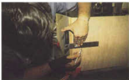
2. Laying out the corner for biscuit joints.
