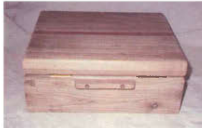
Photo 8. The lid support strip is shown attached to the rear of the box.
