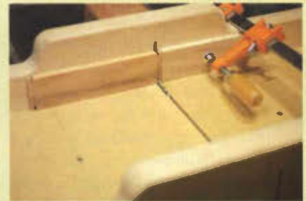
Photo 12 The length of the tenon was milled by cross cutting on the table saw. A gauge block clamped in place assured accurate, repetitive cuts.
