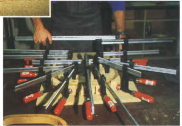
Photo 6. The eight strips fully glued and clamped around the bending form. In the foreground, a previously bent part is out of the form. Note that it holds its shape with no perceivable spring back!
