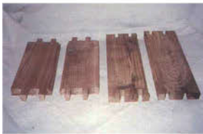
Photo 1. The side pieces are shown with dovetails already cut. These joints make the humididor more visually appealing.
