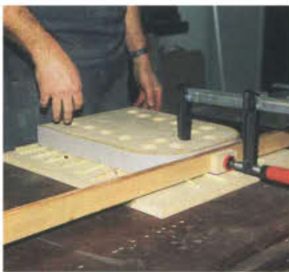
Photo 2. After marking the approximate center of the glued up stack of strips, set the center of the stack at the top of the form and set the first clamp here. Make sure all the pieces are pushed down flat.
