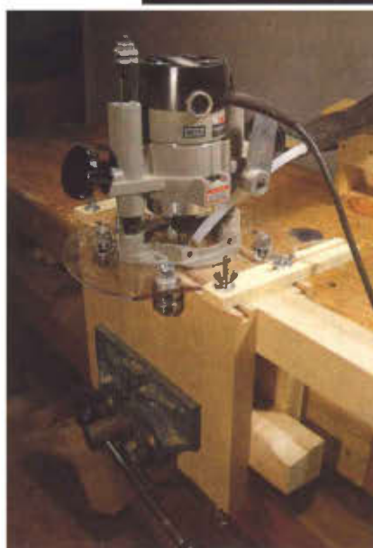
Photo 1 Andy has his slat mortising jig set up and ready to run. Using this and the vice-mounted jig at left, he milled 80 mortises in just 32 minutes.
