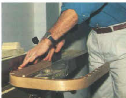
Photos 7 and 8. With the jointer fence moved to the left for safety, the top edge of the part on the form (the edge you could clean the glue from) is jointed flat and square to the side. When jointing, use special caution keeping your fingers on top of the work only. First run the part with the machine turned off to get a feel for the turns and placement of your hands.
