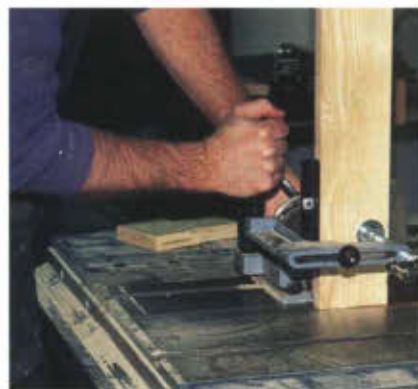
Photo 12. The table apron tenons were cut using a mortising jig and table saw. A filler block is necessary when tenoning the apron with the drawer front cut out.
