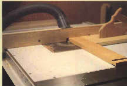
Photo 11 Using the push block on the router table helped move the work over the router bit and added a good margin of safety. It also prevented tearout when the knife exited the cut.
