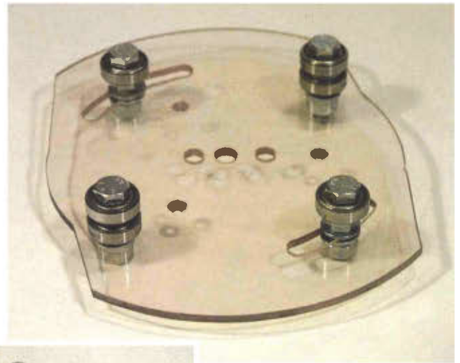
Photo 8 (above) The completed shoe for the vice-mounted jig with two fixed bearings, two adjustable bearings, and other holes for router bit, mounted holes and vacuum holes.
