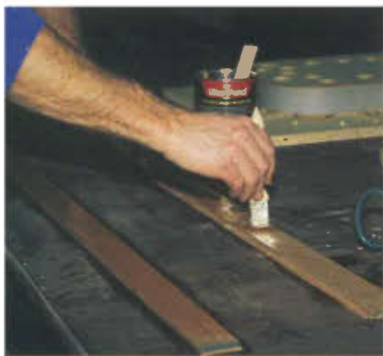
Photo 1. When applying glue to the eight strips to be bent, keep them in a stack after brushing on a moderate amount of glue. By stacking, you slow the drying of the glue, providing more time for clamping on the form.
