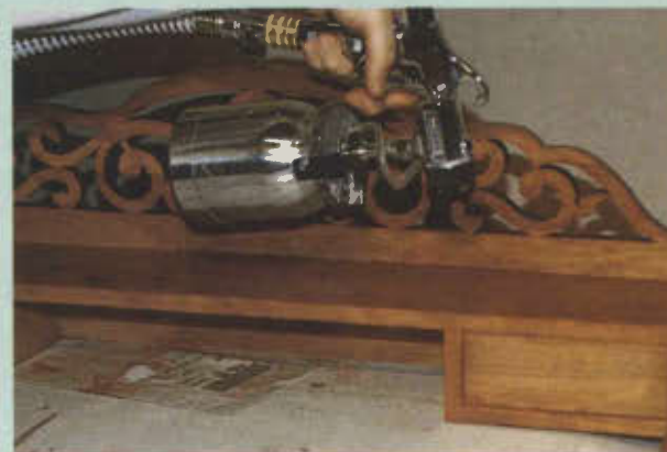
Using an HVLP sprayer simplified finishing. The adjustable spray pattern helped when spraying intricate details.
