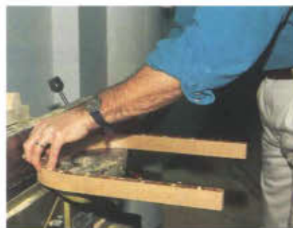
Photos 7 and 8. With the jointer fence moved to the left for safety, the top edge of the part on the form (the edge you could clean the glue from) is jointed flat and square to the side. When jointing, use special caution keeping your fingers on top of the work only. First run the part with the machine turned off to get a feel for the turns and placement of your hands.
