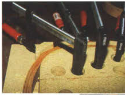
Photo 5. Return to the top of the bending form and work from the center out setting clamps around each corner. Clean top glue squeeze as you go while removal is easier.
