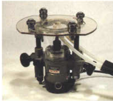
Photo 8 (above) The completed shoe for the vice-mounted jig with two fixed bearings, two adjustable bearings, and other holes for router bit, mounted holes and vacuum holes.
