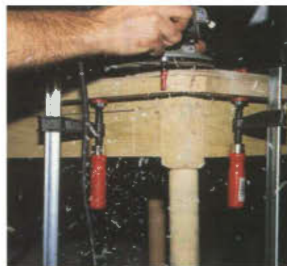
Photo 15. Next, clamp the template in place and trim with a top-mounted bearing flush bit chucked in the router. Avoid tear-out by climb cutting the end grain.
