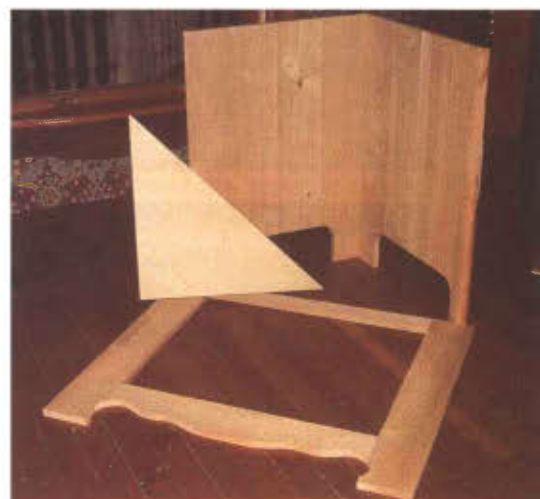
Photo 1. The lower cabinet is shown with the two back pieces attached, and the bottom and face frame loose.
