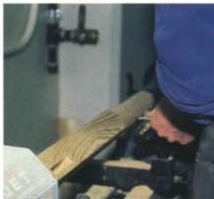
Photo 11. After mortising, each of the four legs were turned to a cylinder beginning at a point just below the junction of the leg and apron.
