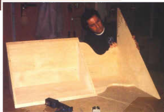
Photo 8. The counter top for the lower cabinet is attached to the upper assembly. Edge detail and sanding should be completed before assembly to the upper section.
