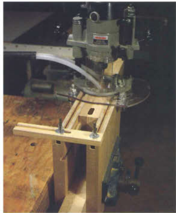
Photo 5 The leg mortising jig tightened in the vice for stability with the piece to be mortised held in place.
