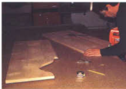
Photo 6. The scroll work curves between the upper and lower cabinets. It should be cut and sanded prior to assembly.
