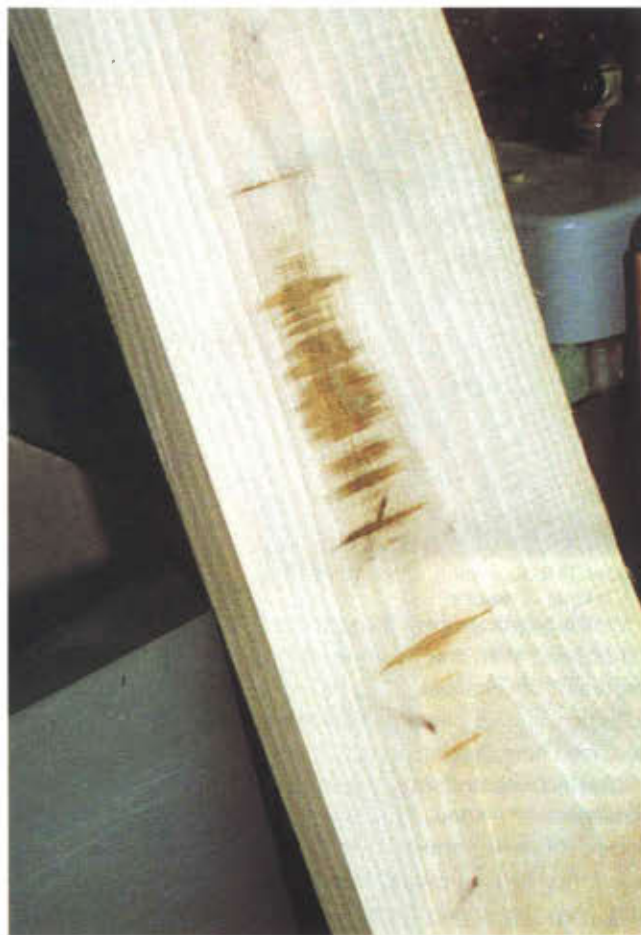
Photo 5. Subsequent passes on the jointer have flattened one face, leaving some rough surface that will clean up during planing.
