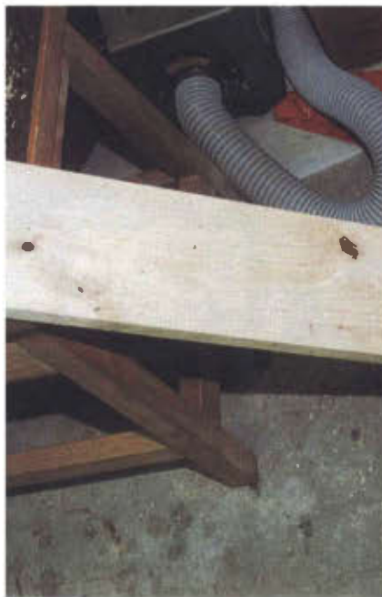
Photo 8. With one face planed nearly smooth, it's time to flip the board and plane the jointed face.
