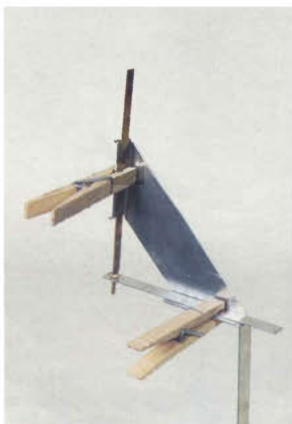
Figure 7. Don't cut part to length until they have been joined.
