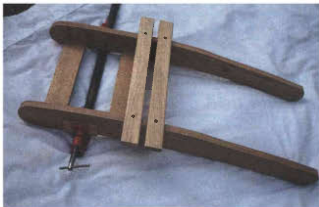
Photo 8. Start attaching the slats 15¼" down from the non- tapered edge.
