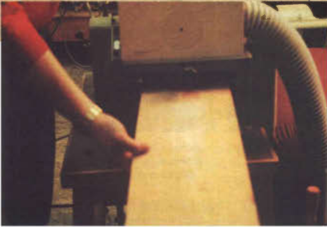
Photo 6. Since the board was jointed with the cup side down, the first passes through the planer will skim the "crown" on the opposite face.
