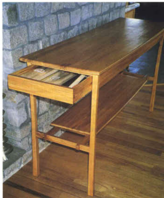
The end drawer fronts are integral to end skirts.
