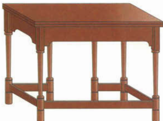
In this front perspective, we see a double thickness top. The leaf, resting on the table top, hinges at rear.
