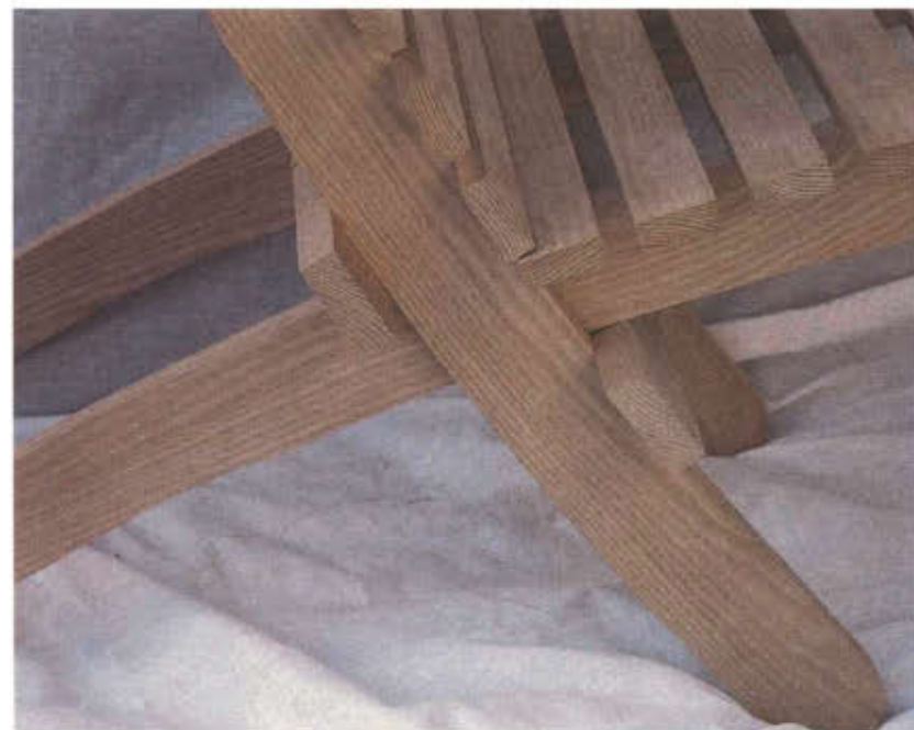
Photo 10. Placement of the lower and upper sup- ports will be impor- tant for the overall strength of the chair.
