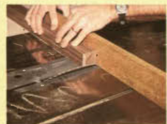
Photo 8. Trimming the bevel on the leg bottoms using the table saw was quick and easy.
