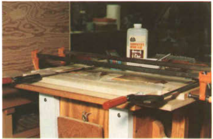
Photo 2. A two-sided square frame worktable makes gluing the raised panel sections easier and more accurate. Notice the wax paper used to keep the side panel from being glued to the frame.
