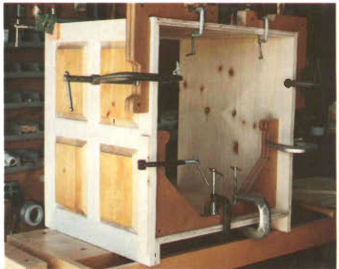
Photo 3. The base cabinets are glued-up after all dados and grooves are cut. Note that the base cabinets' bottoms are set up from the bottom 3" using a dado on the inside panel and base support on the outside panel assembly. All other cabinet carcasses will have the bottom flush to the sides lower edge.
