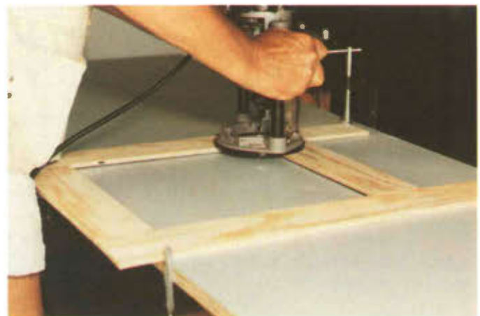
Photo 4. A routing jig is used to cut the drop-in bases for the top. This process is performed after the laminate has been glued in place, but before the two thicknesses of the top have been glued together.
