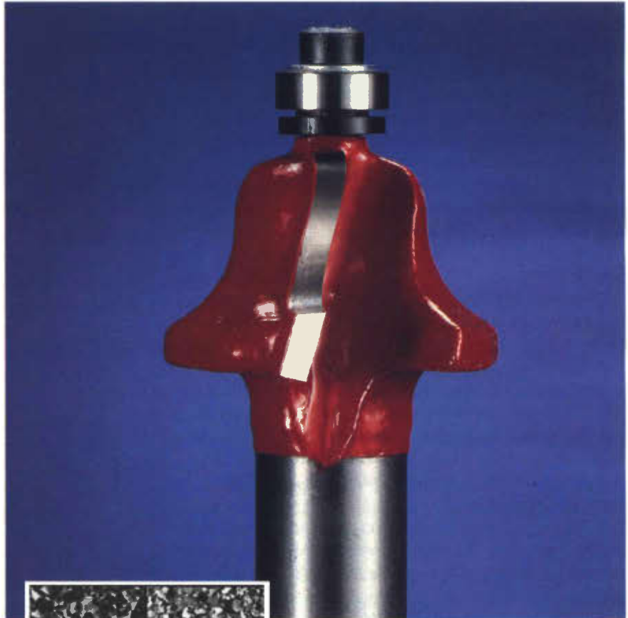
Photo 2. The shear angle of a bit is the angle that the cutting edge makes with the shank of the bit. The bit shown above employs carbide tips angled to slice through wood fibers similar in principal to using a hand plane at an angle to the direction of motion. The slicing action becomes even more important when cutting cross grain. Bits without shear or with too little shear chop the wood and are more likely to produce tear-out and chatter marks. (Information and photo provided by Freud.)
