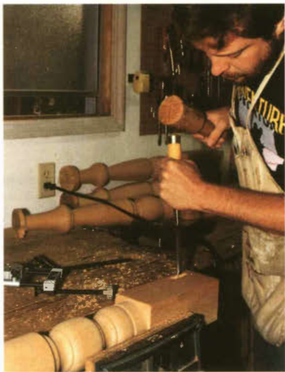
Photo 3. After chain drilling the through mortises, the author finishes the joint by squaring the corners and flattening the cheeks.
