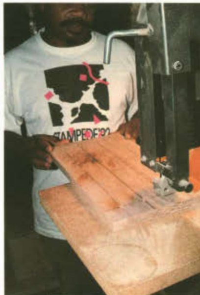
Photo 3. The cuts on the top are done with a bandsaw, cutting first along the length of the tongues, and then dividing the tongues by length. The entry cut at the bridge is later glued back together.
