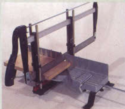
Photo 1 Blades on the Nobex miter saw are tensioned in a frame, much like a bow saw. Replacing blades and providing correct tension is an easy procedure.
