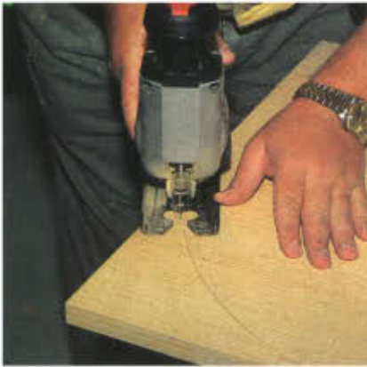
Photo 1 Use a jigsaw to cut the radius on the sides. Pay attention to tear out by cutting from the inside of each piece.
