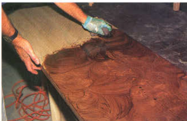
Photo 14 Grain filler, stained to the desired color, is ragged on in a circular motion. After it flashes, or starts to dry, it is first rubbed off against the grain driving it deep into the open pores. Next, the filler is wiped with the grain to remove any excess remaining on the surface.
