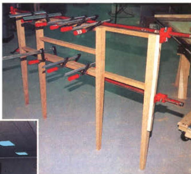
Photo 4 (left) The step out drawer section, leg and rail assembly is glued with dowel joints and clamped. The diagonal clamp is used to pull the assembly square while the glue dries.
