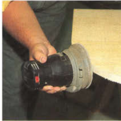
Photo 2 Sanding the radius with a random orbital will remove the jig saw marks, but make sure you don't round over or lose the square edge.
