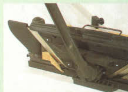
Photo 6 The final cut should always result in see-through shavings that curl away. This will leave an edge that requires no further attention before assembly.
