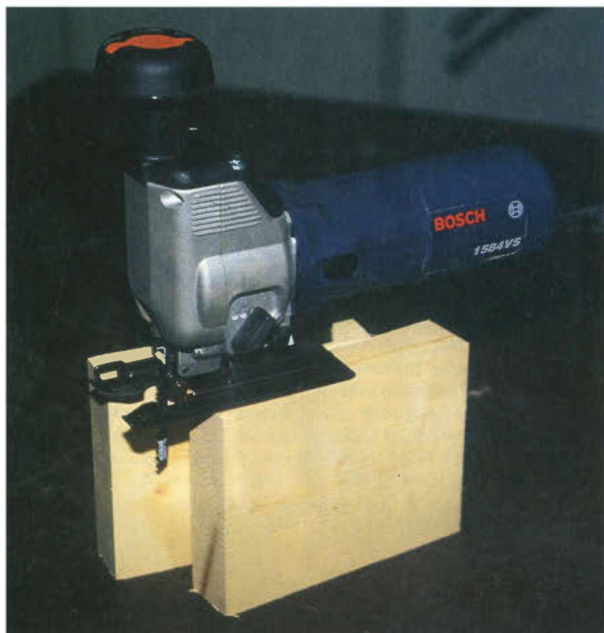
The sabre saw's fairly tight radius of turn makes it a highly maneuverable alternative to the band saw, and a fair competitor for much scroll saw work.
