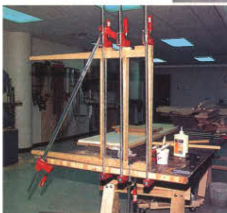
Photo 4 (left) The step out drawer section, leg and rail assembly is glued with dowel joints and clamped. The diagonal clamp is used to pull the assembly square while the glue dries.
