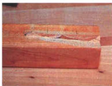
When the joint failed, the wood broke and took some of the biscuits with it.
