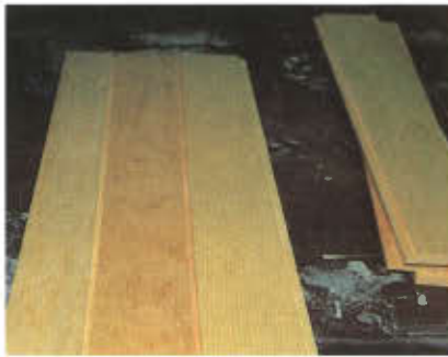
Photo 4 The \frac{1}{4} " spacing shown on the back panels is accomplished by rabbeting a \frac{1}{4} " x \frac{1}{2} " rabbet on opposing long edges.
