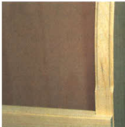
Photo 5 By using a portion of a roman ogee bit, a delicate detail is added to the radiused edges of the sides. A cove bit with a guide bearing will work nicely, too.
