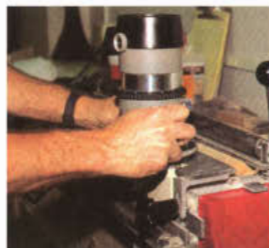
Photo 9 Half blind dovetails routed on a jig were used for drawer construction. Another method would be to rabbet the front and back to receive the sides.
