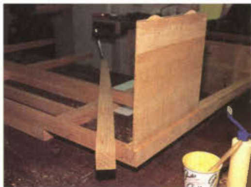
Photo 6 (above) The cabinet sides are glued to the legs using biscuits to align. The side setback from the leg is created by simply adding a 1/4" spacer under the biscuit joiner fence when cutting the side slots.
