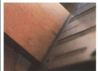
The joiner has three marks — a centerline and two at the outer limits of either side of a cut. The board in the photo probably doesn't need the mark, because most of us could align its center by sighting on the three marks on the joiner.
