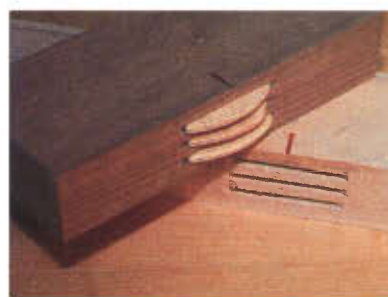
The joiner can be used for making stacked biscuit joints. By the time this is glued together, almost nothing will take it apart without destroying the wood first.
