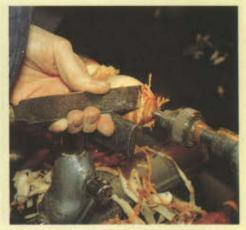
With both ends roughly shaped, turn the tailstock end down further to produce a small stub, which can be removed.
