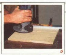
Now, using a clamped straight edge, route the ¼" wide by ¼" deep dados that will later accept the ends of the two shelves. It's imperative that, during the design process, you plan the angles and curves in such away that the shelf ends enter the dados at an approximately 90° angle. You can do this by using the same radius point for all of the arcs.
