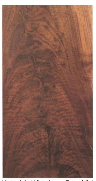
A fine example of crotch Black walnut veneer. The veneer is sliced from the tree at the intersection of a main branch to the trunk. It is typically used as the panel for door frames in cabinetwork. (Crotch veneer courtesy of Constantine's.)
