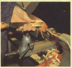
4 Use the rolling, swinging action to shape the egg (which is only an enlarged bead), bringing the handle up as you near the center.
