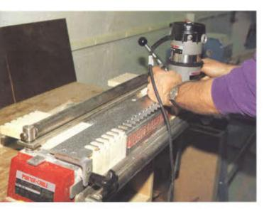
**Photo 5** Drawer sides were joined to the front and back using  $\frac{1}{2}$ <sup>n</sup> half blind dovetails cut on a dovetail jig.
