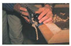
Photo 12 Because the panel raising bit left a tenon, the bevel profile was finished usina a bench plane.
