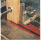
Photo 2 A table saw tenoning assessory is a safe and accurate method for cutting tenons. Since the leg and apron are flush, a precise set-up is important.
