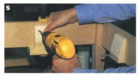
Photo 4 "L" or corner brackets are used to support the removable display tray. To accurately postion them, clamp a block under the apron, set them in place and fasten to apron. Photo 5 Nesting blocks keep the tray in postion. They are tapered for easy placement and removal of the display tray.
