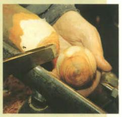
14 Cupping the egg in your left hand, cut the egg off with the long point of the skew, which you can control with one hand.
