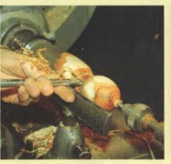
10 Use a fingernall gouge to remove wood from the waste to the chuck side of the egg. This gives access for parting off.
