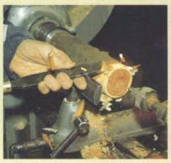
With the log reversed on the chuck you can rough it out with or without the tailstock.
