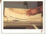
Set your table saw to the appropriate cut (the fence setting will depend upon the thickness of your material; you want to leave a '4" thick rail), and (gingerly!), using multiple cuts and raising the blade about an inch at a time, slice the two curved backstops free of their board. Another, even simpler, method would be to start with '4" stock. Draw the arcs, cut them out on a band saw, and sand the edges smooth.
