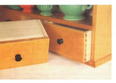
**Photo 6** The drawer bottoms are %" thick but are beveled to slip into a %" groove, a traditional drawer construction method.
