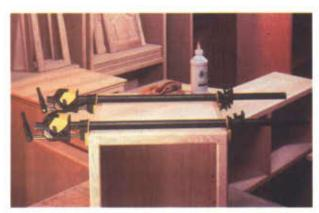
The clamp also features a "Flip Handle" that can be finger adjusted in the extended position at either end, eliminating awkward repositioning. The clamp also features an eight-pitch screw instead of the usual six-pitch design, allowing for finer adjustment and powerful pressure. The clamps may also stand freely, which may eliminate the need for a clamp stand.
