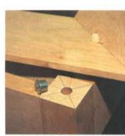
Photo 13 Dowel centers were used to locate the mating holes which position the top on the base.
