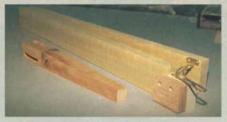
be sure the arms are milled straight and square. Before attaching the hinge, make any necessary preparations for the lid support. Be sure to chose a support that'll lock in place easily. We used a Brainerd™ Standard lid support, and cut a notch in one arm opposite the hinge end to properly attach it. On the ouside of that same
