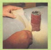
Photo C After bandsawing to the line traced from the tempiate, a spindie sander cleansup the kerf marks from sawing the shape of the arm support.
