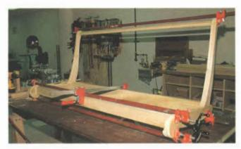
Photo 12 The frame is glued and clamped.
