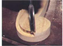
**Photo 7** After the ½" x ½" rabbet is routed into the two ends, the start and stop points must be squared using a chisel.
