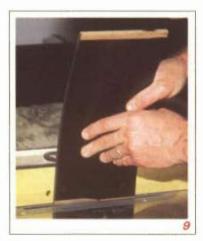
Rabbet the ends of the shelves to match the 'A" dados by carefully removing material from the undersides of the shelves, leaving a 'A- X 'A" tongue.
