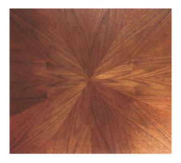
hole is advisable, but wax lubricants are unnecessary. The wood resists glue staining well, and both resin and epoxy glues present few complications.
