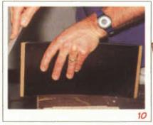
10 Use a rasp to ease (slightly!) the edges and nip the corners of the shelves to help them start into the pre-cut dados.
