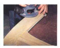
**Photo 8** A %" roundover bit is used to soften the edges of the end pieces.
