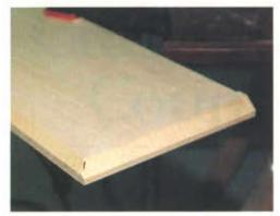
Photo 2 Before assembly, the plain maple bottom is edged with curly maple then chamfered using a router.
