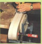
Photo D The two seat ends are shown clamped together while a random orbit sander does final sanding on the two pieces.
