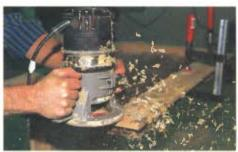
Photo 11 Most of the top edge profile was cut using a panel raising router bit. Cut the profile in three passes since you're removing substantial material.
