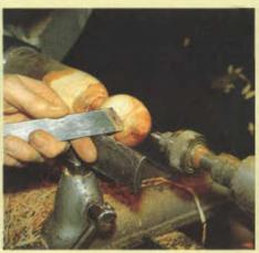
11 Having pulled back the tailstock, you can clean up the end. On a cleaning cut, use the long point — It's easier to feather in.
