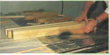
Photo 3 The table leg inside faces were tapered on the table saw using an adjustable tapering jig (see Make Your Own Adjustable Tapering Jig). The easy to make jig (about 30 minutes) produces safe, accurate cuts. You'll use it on many future projects, too!
