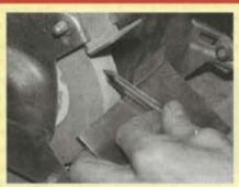
2 As you roll the gouge over, swing It round, keeping the degree of roll and swing constant.
