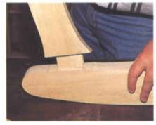
Photo 5 Pinch dogs were used to pull the joint tight. Though this leaves small holes in the work surface, it avoids the difficulties involved in clamping curved and angled surfaces. These inexpensive tools are extremely handy in many situations.
