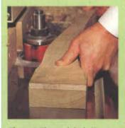
Photo A The straight knife set flush in a ball bearing rub collar is shown in use on the shaper. Note hand position behind work.
