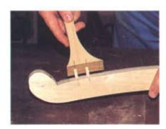
**Photo 6** The arm and arm support are attached using ½" dowels.
