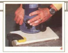
While waiting for the shelves to dry, go ahead and cut the maple sides to size, matching the angles (see PullOut plans) along the top and bottom. Use a router and roundover bit to add a little interest to the outer edges of the two sides.
