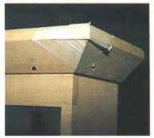
Photo 4 A simple method for "clamping" the crown when gluing is using masking tape—just pull it tight over the joint.
