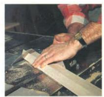
Photo 3 The crown compound miter is cut on the table saw. Tilt the blade to 30° and the miter gauge to 35°.
