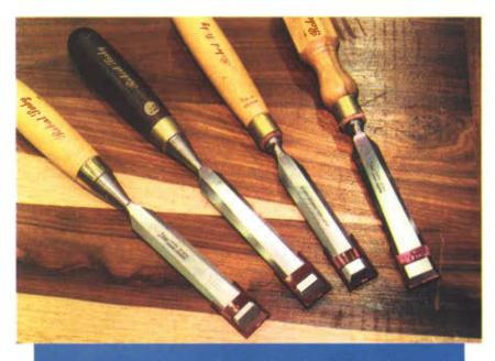
Photo 5. Choose bevel edge chisels when cutting in corners of less than 90°. Above, Robert Sorby brand chisels offer a range of handle styles in bevel edge chisels.
