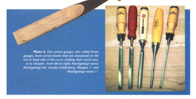
high carbon steel for longer life. Examining the %" equivalents, I see that the Stanley is 12mm, and the Marples is 13mm. The Marples is approximately %" longer than the Stanley which has "carving tool round" handles. The Marples is a squared-off round. Their circumferences are identical—3%" (which produces a working diameter of about 30mm, just shy of 1%").
