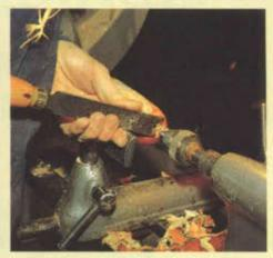
5When working at the end of the blank it certainly helps to have the tailstock up, to keep vibration to a minimum.
