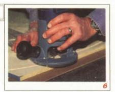
Guing the same router jig setup used for the forms and a ¼" straight router bit, mark and cut, to a depth of a ¾" to ¾", the outer edges of the two curved back rails. Leaving them, at this stage, as simply two sets of curved, parallel grooves in the maple board.
