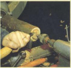
1 It's best to turn the egg in a chuck, so work a stub at one end between centers first, using a parting and beading tool, for the chuck.
