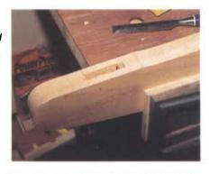
Photo 4 Before gluing, the back and seat end pieces are dry fit. Looks like the mortise and tenon are a good fit!
