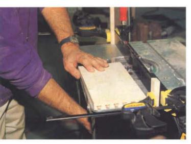
**Photo 7** A stopped groove was required on the inside of the drawer front to receive the bottom. It was cut with a router.
