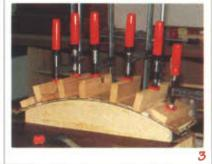
Don't skimp on clamps, the more the better for this sort of job. Allow the clamped fiberboard to sit overnight before removing it from the forms.
