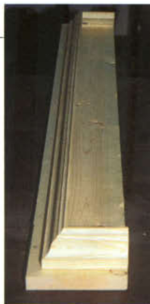
Photo 2 The crown molding pieces are shown attached to the mantel top.
