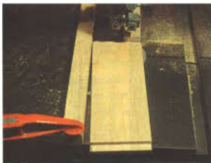
Photo 6 I used a fence with a drywall screw screwed into it to establish the correct angle for the shoulder cut into the angled tenon.
