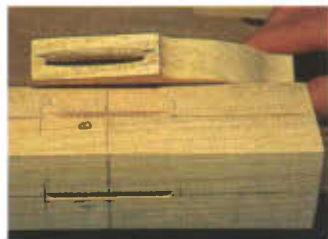
Photo 2 Biscuits were used to join the braces to the post. Depending on your biscuit joiner this may be tricky, and dowels may be a better option.
