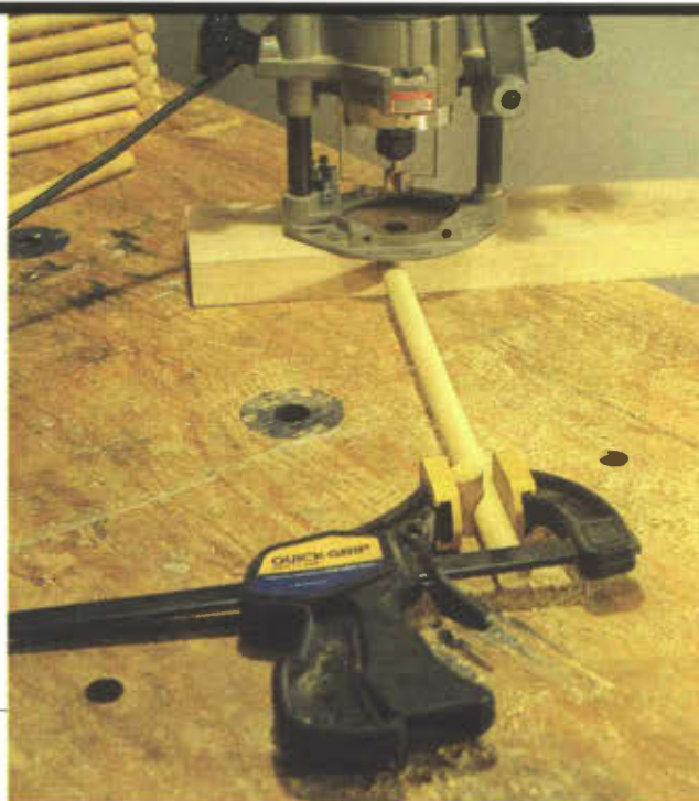
Photo 6 I cut the half-moon joint with a special jig that mounts on the base plate of the router. I routed parallel joints by holding the log in the correct position vertically.
