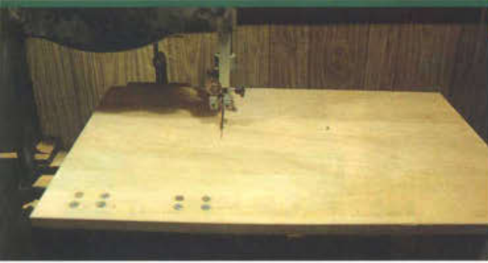
Photo 9 The best way to cut the circular tops is with a circle-cutting jig on the band saw. As you can see, the jig is simply a sheet of plywood with a \frac{3}{4} " cleat screwed on the bottom that rides in the band saw's miter gauge slot. Advance the jig into the saw blade while the band saw runs until the teeth just meet the centerline of the jig, which runs from the left to the right of the photo. To find the pivot point for the 14"-diameter top, simply drive a nail through the jig on that line, 7" to the right of the saw blade.
