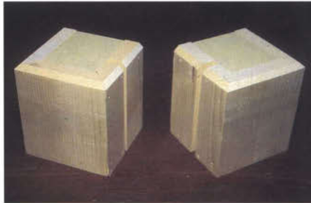
Photo 4 The assembled plinth blocks will be left and right, determined by the location of the groove cuts.
