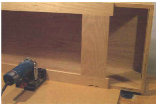
Photo 7 I use a combination of biscuit joinery and drywall screws through the upper and lower carcase members to secure the face frame to the jelly cupboard carcase. Here I'm cutting the biscuit joints in the jelly cupboard face frame. See "Three Pocket Joints" to learn how I cut pocket joints for the drywall screws.
