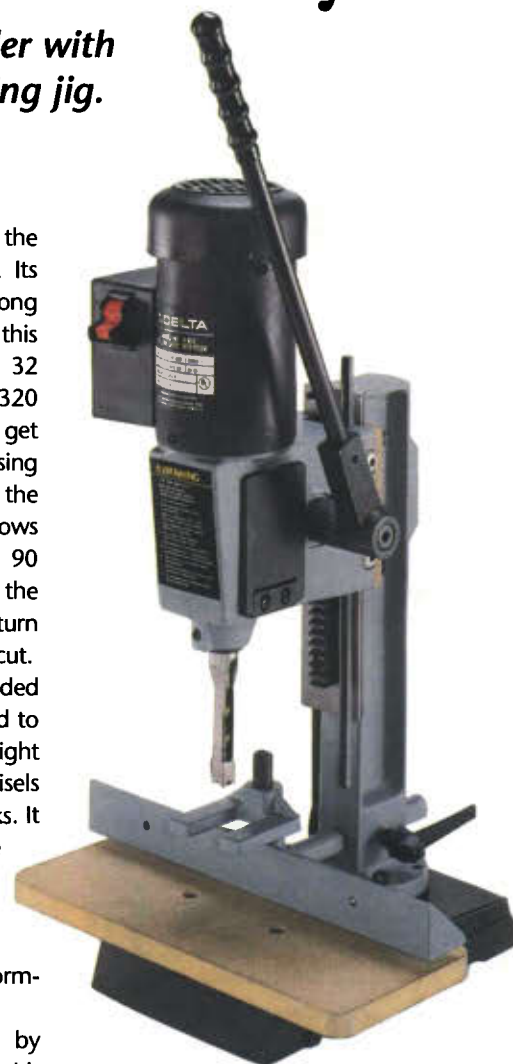
Photo 2 A hold-down, reversible for wide work, keeps parts secure when retracting the chisel. The wood table is on the small side, but a longer piece of plywood can be substituted if necessary. The cast iron fence is drilled so a wood facing can be attached.
