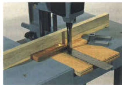
Photo 3 The first step when setting up for any mortise is to be sure the angle between the side of the chisel and the fence is 90 degrees. It's a good idea to check this alignment as you go when doing a considerable amount of cutting. Note the centered insert is easily replaceable.
