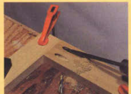
Photos E & F Commercially available jigs make quick work of pocket joints when producing them in quantities of ten or more.
