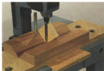
Photo 7 The gauge is used to accurately establish the position for the V-block jig. The text explains the procedure to follow.
