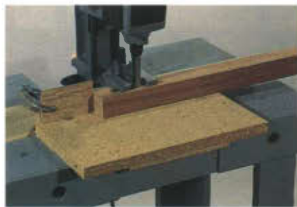
Photo 4 Cutting a traditional mortise. The hold-down should rest on the work, not be forced against it. Note the clamped stop block, in place to gauge the length of the mortise.
