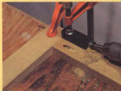
Photos E & F Commercially available jigs make quick work of pocket joints when producing them in quantities of ten or more.
