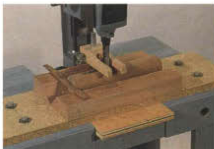
Photo 8 Mortising is done in a fairly routine fashion. The difference is that the work, cradled in a V-block, is round. A strip of wood, tack-nailed across the "V," is used to gauge the length of the mortise.
