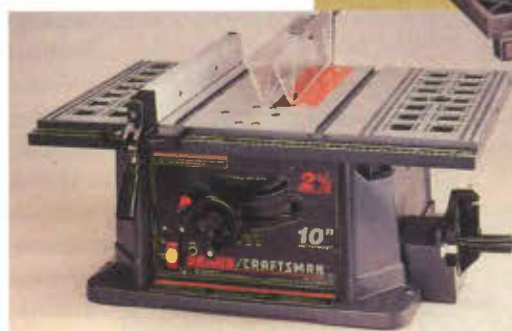
Photo 1 The major sawing tool for the $1,000 workshop is a benchtop, 10" table saw. Even the lowest-price units have the power and capacity to rip, crosscut and cut 45-degree bevels on two-by-four stock.
