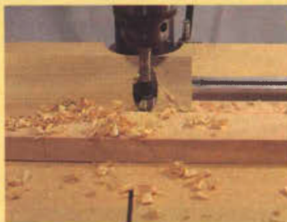
Photo D I cut pockets for hidden drywall screws with a Forstner bit in the drill press. Note that I clamp a stop block to keep the workpiece from moving as the bit first bites into the wood. The wood has a tendency to self-feed without this stop block.
