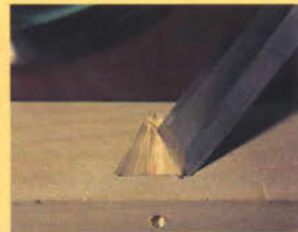
Photos A, B, & C One way to cut the pocket is to drill the screwhole first, marking where the drill bit emerges from the wood. (Make sure you know which face will show, and drill through the opposite side.) Then use a chisel to pare away the pocket.
