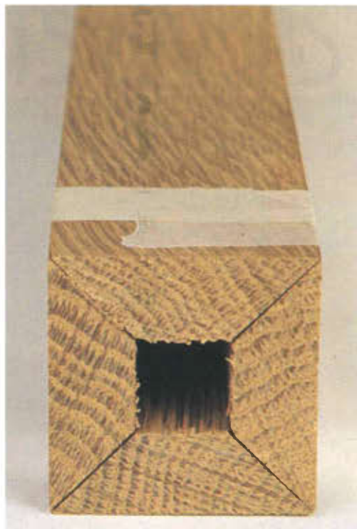
Photo 2 The quadrilinear design saves material and puts quarter-sawn grain on all four sides.
