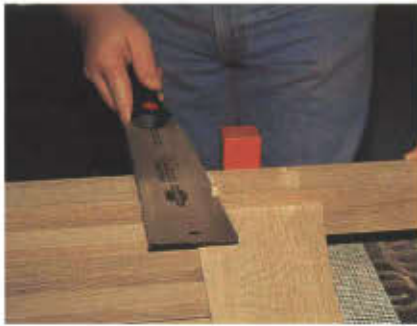
Photo 9 Keep the saw blade parallel to the leg surface while cutting the peg flush.
