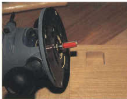
Photo 12 A flush cutting knife makes clean work of the through mortise in the arm.
