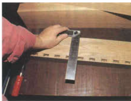
Photo 2 Time spent carefully laying out the mortise locations will pay in big dividends during assembly.
