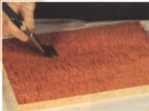
Photo 4 Sealing with a two-pound cut dark shellac.
