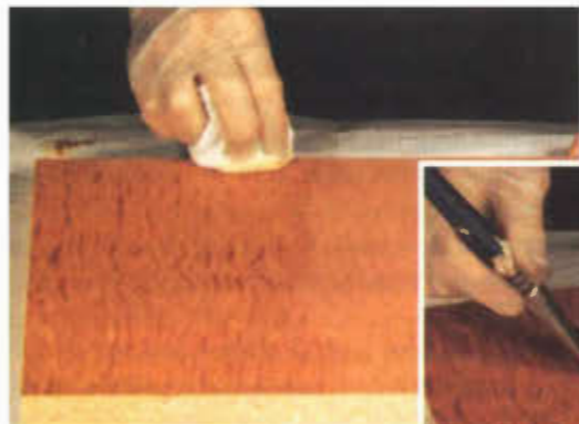
Photo 3 Sealing with linseed oil.
