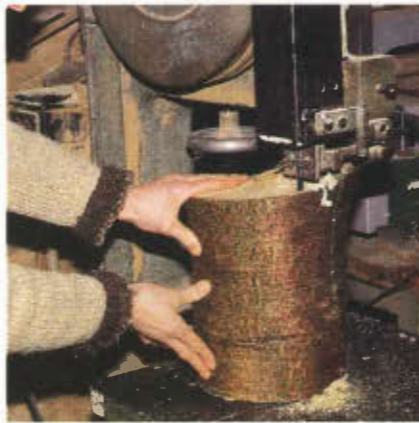
4 Cut a flat off the side of the log half so the blank will sit on the band saw table evenly for circle cutting.
