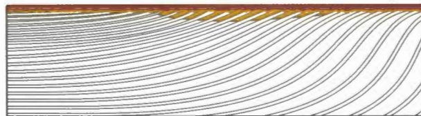
Stain controller fills the wood's pores so the liquid stain can't penetrate. It mixes with the stain controller near the surface.
