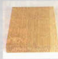
Quarter-sawn oak has near vertical end grain.
