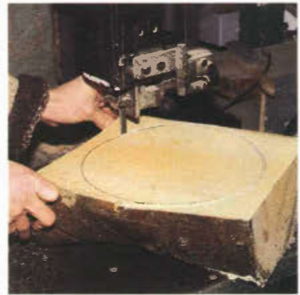
5 Draw a circle on the largest flat face of the log half and cut around it with the band saw.
