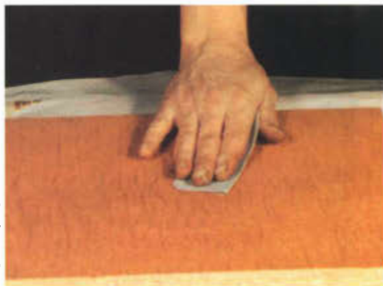
Photo 2 Scuff-sanding the dried dye very lightly with 320 grit. Use your hand to back the paper.
