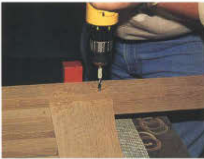
Photo 8 When drilling the peg holes, a piece of tape on the bit inexpensively controls depth.
