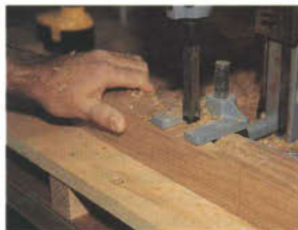
Photo 1 A bench-top mortiser makes the repetitive work more manageable.
