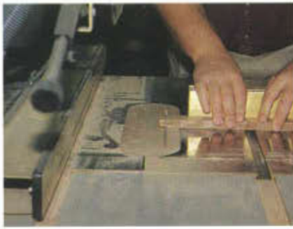
Photo 5 Use a stop block on the miter gauge to set the tenon shoulder depth.
