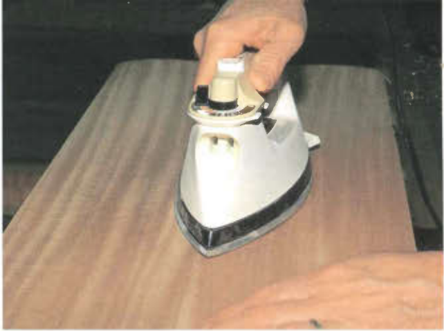
6 Begin ironing each side, working from the center out. Move the iron very slowly, allowing the heat to penetrate through the veneer and glue coatings below.
