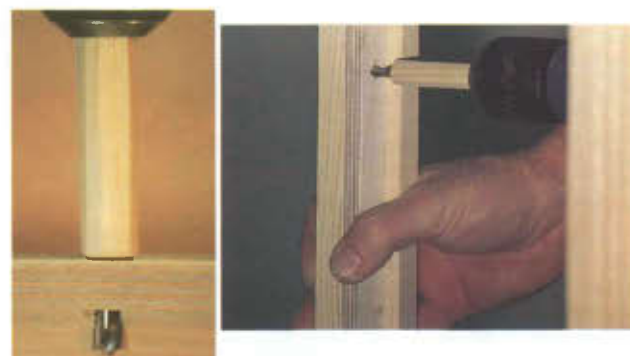
10&11 Two simple drilling jigs assure correct location and depth of drilling. Shown at right are a detail of the two jigs at work and the results they produce.
