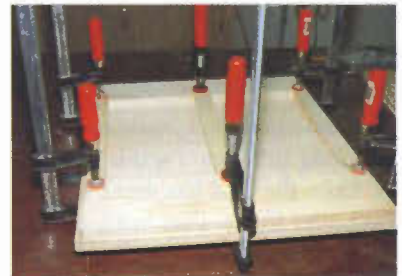
4 The frames will stay flat by clamping them together using a simple MDF backing board.
