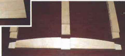
4 The frames will stay flat by clamping them together using a simple MDF backing board.
