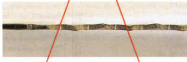
Crosscut teeth filed at a 70 degree angle
