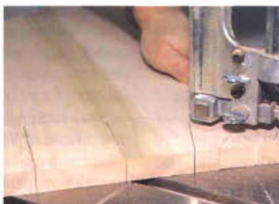
4 Now proceed with sawing the irregular shape.
