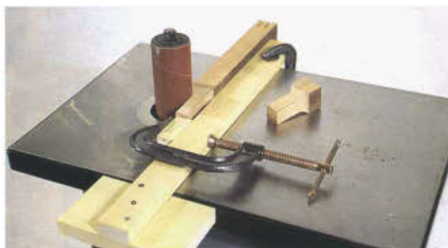
9 You can be quite generous with depth of cut to reduce width if you feed the work at a reasonable pace.
