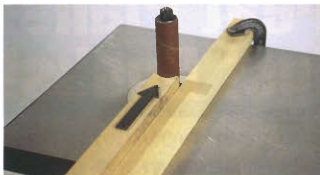
8 Producing a cove on the end of a piece works well, with a little patience.
