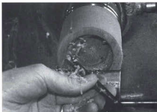
3 With a long bevel ground on the edge of a deep fluted gouge, you can start at the edge and work inward.
