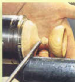
F Sand and polish the outside and inside of the lid before you take the knob too far down and lose stability.
