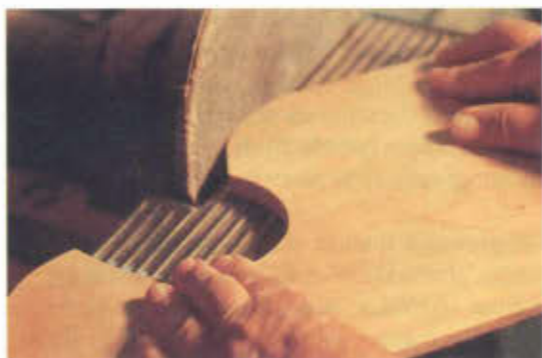
4 Outside curves can be sanded using a disc or belt sander.
