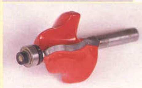
The anti-kickback design offers a much smaller gullet space to avoid anything being trapped between the wings. The extra material also improves the stability of the cut.
