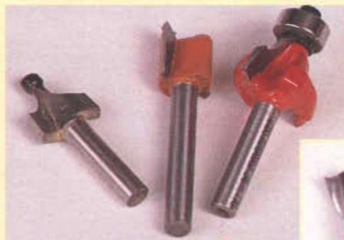
An integral pin-guided bit (far left, note the burned surface of the pin), a non-guided bit, center, and on the right a bearing-guided bit.
