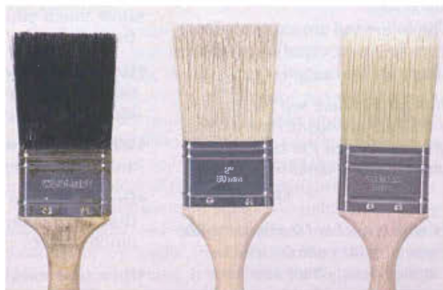
Three types of brushes: a black China bristle brush (left), a white China (center), and a synthetic bristle brush (right).
