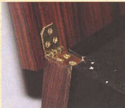
Detail of support bracket and recess cut into the underside of the top (left), and hinge recess at the front near the drawer shown fully opened (right).
