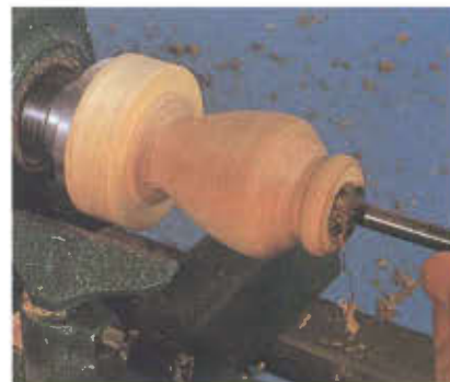
Boring the hole for the glass vial using a Forstner bit chucked in the tail stock.
