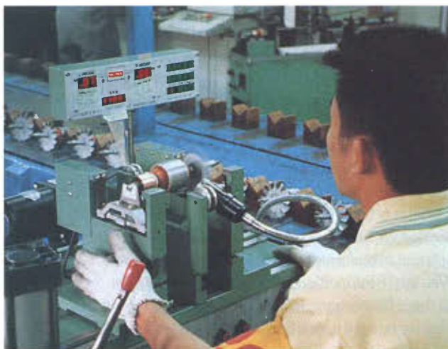
An employee at the Kosta Plant in Taiwan balances the armature on a universal motor. The plant assembles tools and tests motors for Delta Manufacturing.
