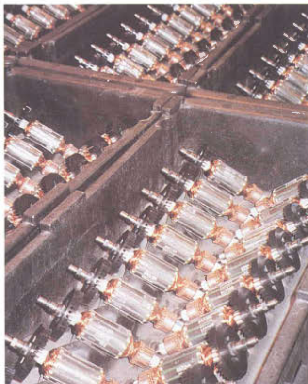
Assembled armatures and commutators at Makita's plant in Georgia. We were impressed with the rigorous tests Makita performed on their universal motors.
