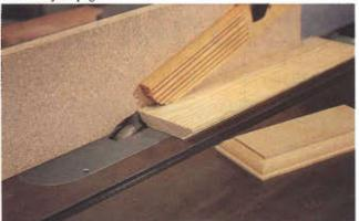
2 A featherboard, clamped to bear down on the work in front of the cutter, will help keep the work in the correct position.
