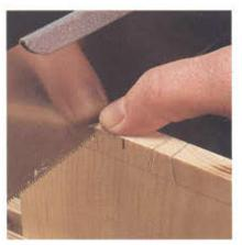
Use a saw with a rigid spine to cut the tails. The traditional European tool is a backsaw. We have become very fond of the Japanese-style saws, which cut on the pull stroke. Definitely worth a \$25 to \$50 investment.
