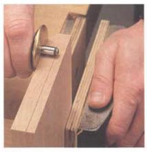
With your marking gauge at the same 1/2" setting, scribe a line on the end grain from the back of the drawer front to locate how far in the tails will penetrate into the front.
