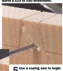
removing the waste. After you make the first cut at an angle (above), you can come back and clean out most of the remaining waste (left).
