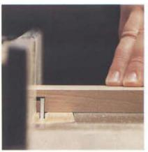
4 Make the second cut on the drawer front's rabbets by keeping the height of the saw's blade at ½". Set your fence to ½" including the blade thickness. Make the cut with the front face up on the table.
