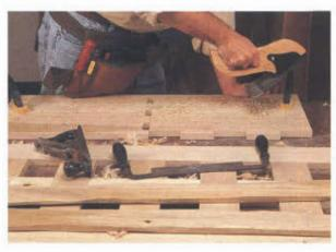
define all of the edges with a <sup>1</sup>/<sub>4</sub>" chisel. Make your cut about <sup>3</sup>/<sub>16</sub>" deep. Then go back and remove the waste up to that line. Now lay out the 24 circular patterns on the bench's back. These are each 1<sup>3</sup>/<sub>8</sub>" in diameter and carved the same way you carved the sides. Finally, carve the square and faceted depressions on the back, seat and sides. See the short story at right for details on how to do this quick-
