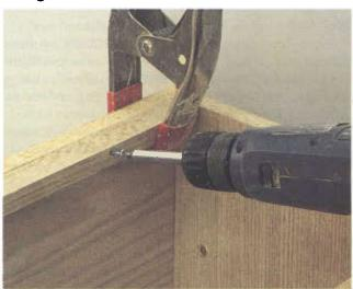
4 CLEATS • Solid wood cleats (poplar is fine) attached to the inside front and back of the lower cabinet strengthen the case, as well as provide a great place to attach the top.
