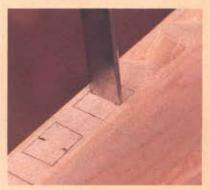
Using a  $\frac{3}{8}$ " chisel, mark the center of the depression. Pound the chisel with a mallet to make this cut about  $\frac{1}{8}$ " deep.
