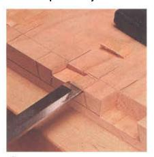
9 Remove the waste around the pins. First chop a line ½16" in from your scribed line (see photo). Then bring your chisel back to your end grain and pop out the waste.
