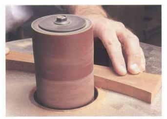
SAND THE LIPS • First cut out the rails with a band saw. Be sure to cut a little wide of the line. Then sand the cuts smooth. I used a spindle sander for this. Use a light touch because cedar is soft.
