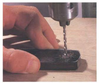
HOLES FOR RIVETS • Drill the holes for the rivets on your drill press. While the epoxy makes a good bond, the rivets will make that bond even stronger.
