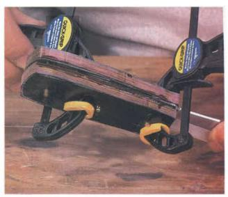
4 EPOXY MAKES IT EASY • Mix up some fresh 30-minute clear epoxy and apply it to the blade tang, handle material and rivets. Assemble everything and clamp together (wax paper will keep the epoxy from sticking to the clamps). Clean off any epoxy that oozes out.
