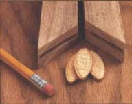
Ability to join face frame stock as narrow as 1 1/2" with our new, exclusive face-frame biscuit. Dust port accepts standard bag or can be connected to a vacuum for a clean work environment.
