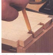
Now place your cut tails on top of the end grain of its drawer front mate. Using a sharp pencil, mark the outline of the tails onto the drawer front. This makes the outline for the pins.
