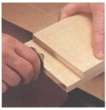
Though this is a source of debate, cut the tails first. Set your marking gauge to ½" and scribe a line all the way around the front end of the side pieces.
