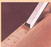
Clean out the waste on the two sides of the depression with the chisel.
