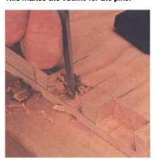
10 Hold your chisel at an angle as shown above to pare out the waste down to your scribed line. Once you make these angled cuts, go back and hog out the waste with your chisel parallel to the scribed line.
