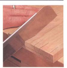
On the inside of the drawer front, bring the mark for the end grain straight out to the scribed line. Cut these with a backsaw. You can make the cut 1" or so beyond your scribed line. This will allow you to clean out a lot more waste with your saw. And don't worry, it's a traditional method.
