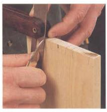
Now lay out the tails. First mark the center of the end grain on the sides. Work out from there to determine how many pins and tails you want. Our tails here are 11/4" wide with 5/16" between each tail. Be sure to lay out your tails so the groove for the bottom will be buried in a tail.
