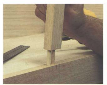
2 FACE FRAME • I used double dowels at all the face frame joints to provide a sturdy joint. Drill straight holes to keep the frame flat.
