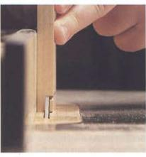
Now make the second cut on the sides that completes the rabbet. Set the height of the saw's blade to  $\frac{1}{2}$ ". Then set your fence so that there's a  $\frac{1}{4}$ " space between the fence and the blade. The outside of the drawer side is against the fence. Make this cut on both ends of the sides. No cuts are required on the  $\frac{1}{2}$ "-thick back, which nestles nicely into the rabbet on the sides.
