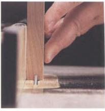
2 Use the same setup to run both ends of the drawer front on edge with the inside face of the drawer front against the fence.
