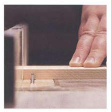
The order of these steps is critical because you want to reset your table saw as little as possible. First work on the drawer sides. Raise your table saw's blade to  $\frac{1}{4}$ " high. Set your fence for  $\frac{1}{2}$ " including the blade thickness. Cut both ends of the sides using this setup with the inside face down on the table.
