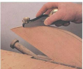
SHAVING AN ELLIPSE. If you are going to change the size of the top, you'll need to use an ellipse-marking jig (top). If not, cut out the wing patterns in the PullOut Plans, Make copies of the wing pattern halves and tape them together. Glue the patterns on the appropriate wings and cut out the oval-shaped wings. Next, clean up the edges of the wings with a block plane and prepare for mortising the hinges (bottom).
