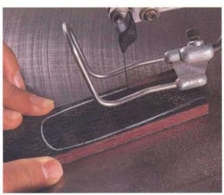
**2** LEAVE SOME MEAT • Leave about an <sup>1</sup>/8" margin of extra material all around the scribed lines. After cutting the first piece, scribe the second piece, being careful to match sides with the first piece.
