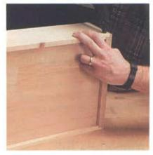
5 After cutting the groove for the bottom, assemble the drawer using glue and nails (7/8" or 1" will do nicely). Three nails in each rabbet are enough for your average drawer. Set the nails, putty the holes and sand the sides.
