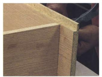
**1** BUILDING THE CARCASE • The bottom is set in a  $^3$ 4" x  $^3$ 8" deep dado,  $2^1$ 4" up from the bottom. In both the upper and lower cabinets, the back sits in a  $^3$ 8" x 1" rabbet. This allows for easier fitting to a wall, and in the upper cabinet, allows room for running wiring for the lighting fixtures.
