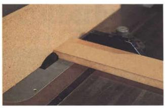
3 End cuts, especially when the work is narrow, are done safely by moving the work with the miter gauge. Be sure of correct alignment. The angle between miter gauge and facing must be 90 degrees.
