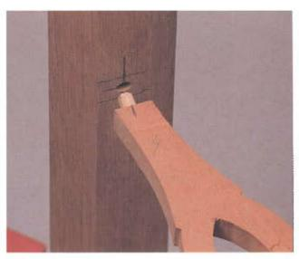
6 MOUNTING THE STRETCHER • After fitting the stretcher, lay out and drill dowel centers so that the stretcher will attach 5" up from the bottom of the legs.
