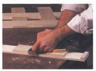
**PRECISION** COUNTS . Because you're dealing with 21 lap Joints, your cuts need to be precise as possible. No matter how careful you are, you might find a little trimming is necessary. I recommend you use a rabbet plane for trimming the sides of the lap joints.
