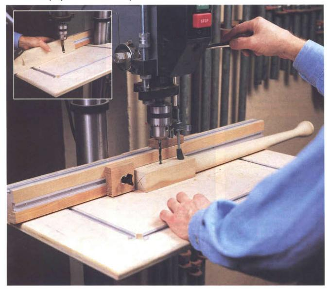
DESPITE THE FACT that your drill press is designed mostly for poking holes in sheet metal, it has many uses in a woodshop. It's a mortiser, a spindle sander, it bores huge holes, and — of course — drills holes at perfect right angles to the table. Because the table on most drill presses is designed for metalworking, it's hardly suited for these tasks. So I built this add-on table with features that will turn your drill press into a far friendlier machine:
