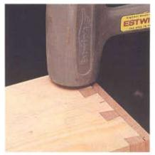
11 Finally, fit the pins and the tails. After fitting, use a dead-blow mallet to push the tails into the pins evenly.
