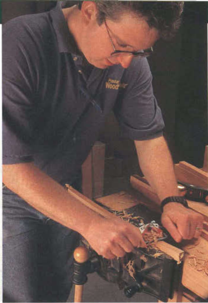
While the slats can be sanded smooth, I find that a spokeshave helps remove irregularities left by the band saw. It also gives the piece a hand-worked appearance.
