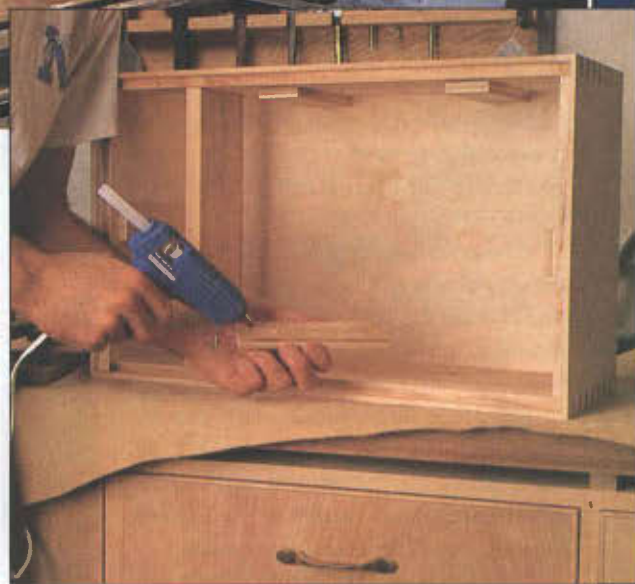
Use hot melt glue to attach 6"-long blocks that keep the saw kerf open when you cut the front off the cabinet (inset). After that, ripping the cabinet is almost cake.
