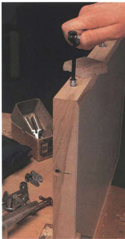
Measure the center locations of the existing holes on the saw table and the fence bars. There are five threaded insert locations per top. Next, drill the 3/8" receiving holes for the inserts. It helps to use a doweling jig, but it's not necessary. Make sure you measure every hole on both sides. They aren't located in exactly the same place.
