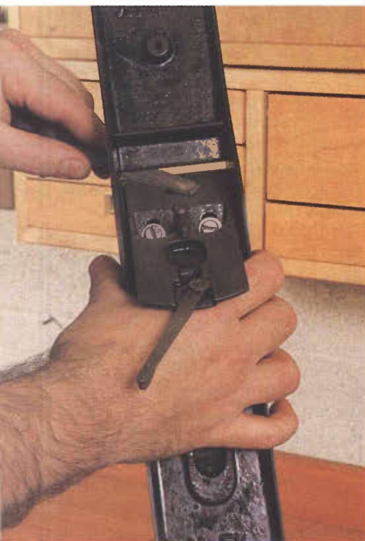
A small metal file works well to clean up the area where the frog meets the sole.
