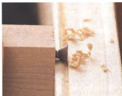
The homemade 10-minute cockbeading tool in use.
