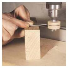
While the wheel is chucked in your drill press, use a common scratch awl to cut a groove around the edge to hold the O-rings.
