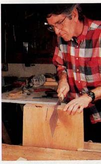
Cut the dovetail sides using a saw without a back because the cut is nearly 3" deep. Also, make sure when starting the cut that the saw is properly aligned on both faces of the panel. Make the cut slowly until you've established the saw kerf following the layout line.
