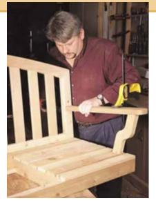
The back of the arm is simply screwed in place through the back stile, while the support is attached to the arm and seat with dowels and polyurethane glue. Notice the foamy squeeze-out of the glue at the joints.
