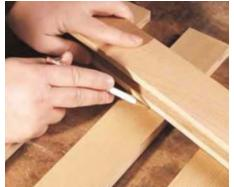
Holding the arched top rail steady was the most difficult part of routing the top groove for the slats. Remember to make the cut in two passes on each side. In this photo you can see that the rail hasn't been cut for length yet, allowing extra support for the router at the beginning and end of the cut (at left).
