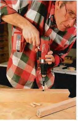
Transfer the dowel hole locations using dowel centers. A slight tap on the top of the legs drives the center point of the dowel center into the beam. Then drill the holes.
