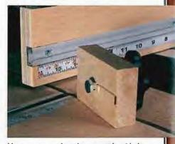
Here you can see how the stop works with the fence system. Note the thin guide strip that prevents your stop from wobbling as you set it.
