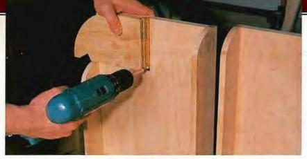
The easiest way to assemble the wing is to attach the hinge to the upright assembly. Then remove it and attach it to the wing. Clamp the upright in a vise and reattach everything. Make sure to mark each hinge's location. Otherwise you'll mess up how some parts go together.
