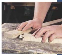
Here's a close-up look at the loose-tenon construction. Cut the mortises in the rails and stiles using a spiral bit in a router.
