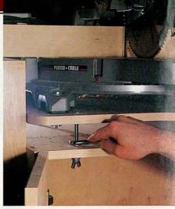
Adjusting the height of the saw is as easy as loosening the wing nuts inside the cabinet and using the jam nuts on top of the cabinet to raise or lower the saw until it's flush with the wing
