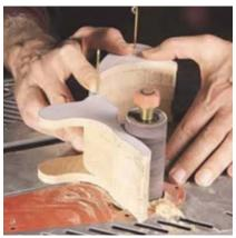
After you adhere your patterns to your wood, drill all the registration holes and then cut the shapes out. I prefer a band saw to a scrollsaw because I'm cutting wide of the line and prefer the speed over the accuracy (left). The trick to sanding the toad is to sand in stages. Once you assemble the first few layers, use your spindle sander to get to the spaces you won't be able to get to once you add the next layers (above).
