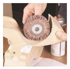
I use an old flap sander chucked into a drill or drill press for the final sanding. An old used flap sander produces a better finish.
