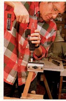
The tapered leg is joined to the bottom beam with two 1/2" dowels. Although the spacing is tight, two dowels can be used. Use a doweling jig for alignment and, depending on placement, make sure you don't drill too deep.
