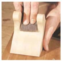
Before finishing, I like to rub the toad's body with a grey synthetic steel wool Scotch Brite® pad made by 3M.
