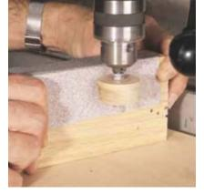
Sanding the wheels can be tricky. If you chuck the wheels into a drill press and press sandpaper against the turning wheel, you're going to create an ellipse. That's because the end grain and long grain of the wheel will sand differently. To prevent this, use a backing board as shown in the photo.
