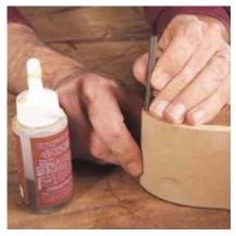
Yes, you can use your spindle sander to smooth the tongue. Use a backing board as shown in the photo to make sure you're sanding it square (left). Once you get the tongue sanded and you've drilled the pilot holes, it's time to add the weight in one end that makes the toad work almost every time. I use polyurethane glue here because it expands as it cures, which locks the rod in place (right).
