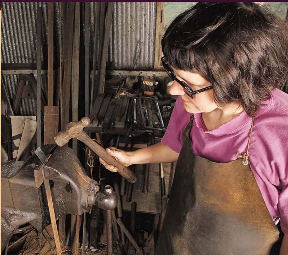
Accomplished blacksmith Marsha Nelson starts the process of hand making a hinge by cold bending flat stock on a jig secured in a vise. The jig provides the correct opening size for the the pintle, or hinge pin (above).
