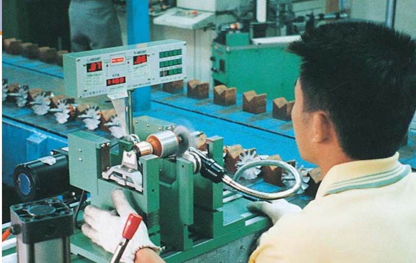
An employee at the Kosta Plant in Taiwan balances the armature on a universal motor. The plant assembles tools and tests motors for Delta Manufacturing.
